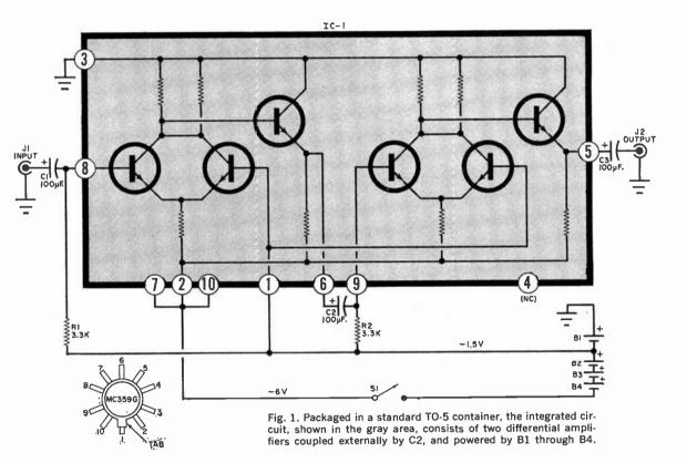
two voltages or currents), each coupled to an emitter follower stage. The output of the first emitter follower is applied to the base of the second differential amplifier input transistor through coupling capacitor C2.
