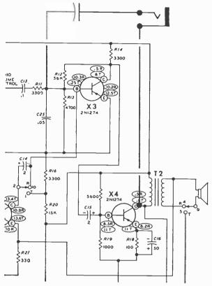
Lines in color on this partial schematic of the GD-51A Heathkit transistor intercom show simple feedback loop. Capacitance value is not critical. Try 0.01 to 0.1  $\mu$ F units to obtain maximum howl. Almost any intercom can be modified using this technique.
