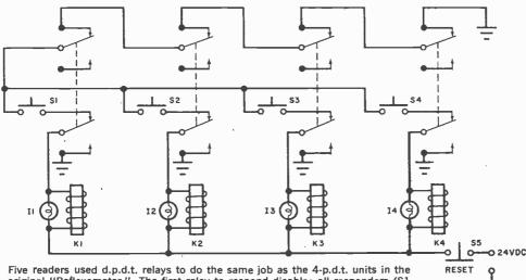
original "Reflexometer." The first relay to respond disables all responders (S1 to S4) and remains "locked" until S5 is reset to start another round of fun.
