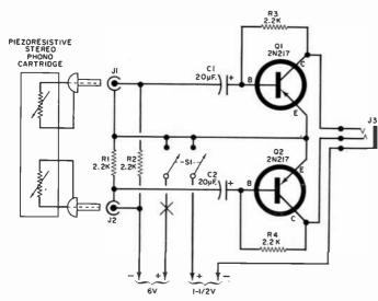
Fig. 1. Strain gauge cartridge acts like a variable resistance and modulates 6-volt d.c. source to drive simple stereo amplifier in step with stylus motion. Text explains stereo phase manipulation. Fig. 2. Mount all parts except the batteries on the back of the front piece of the cabinet. There is enough room to permit installation of an optional volume control. Observe polarity of capacitors.
