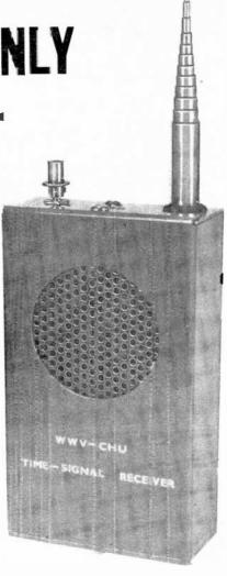
**B** UILD a portable time-signal receiver and you can tune in on standard time broadcasts from your living room, picnic table, boat, car, or even from a private plane. This miniature receiver is a complete superhet circuit with crystalcontrolled local oscillator, prepackaged pretuned i.f. module, and *transformerless* audio amplifier. A printed circuit board makes it easy to build and only a screwdriver (no test equipment) is needed for alignment!
