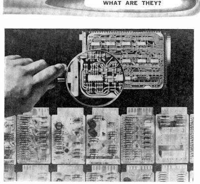
Monolithic integrated circuits, such as the one shown magnified above, are used in Sperry Rand's new UNIVAC 9000 series data processing systems. They perform the same functions as the large conventional printed circuit boards. One chip is the equivalent of 14 conventional printed circuit boards like the ones shown in the lower area of the photo.
