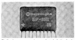
Similar in appearance to a packaged electronic circuit, this Burroughs' IC package features rugged dependability, making its use in electronic equipment subject to shock and vibration most desirable.
