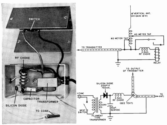
All parts needed to operate the antenna relay from the ham shack are mounted in a small metal box. Note in the diagram how the small chokes keep the r.f. out of the relay circuit. See text for elbow details.
