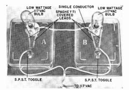
between the two boxes. Whenever a.c. power is applied and switch A is thrown ON, lamp B lights. When switch B is thrown ON, lamp A lights. When both switches are ON, both lamps light—and when both switches are OFF, both lamps are dark.
