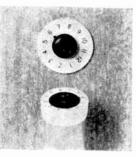
to take your next pill can also be used as shaft position indicators on your electronic projects. To make such an indicator. remove the pointer disc from the lid and drill a 3%"diameter hole in the center of the cap. Then slice off the dial portion of the cap, using a
