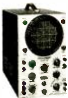
Model 460 Wideband Direct-Coupled 5" Oscilloscope. DC-4.5mc for color and B&W TV service and lab use. Push-pull DC vertical amp. bal. or unbal. Inp.t. Automatic sync limiter and amp. $89.95 kit. $129.50 wired.
