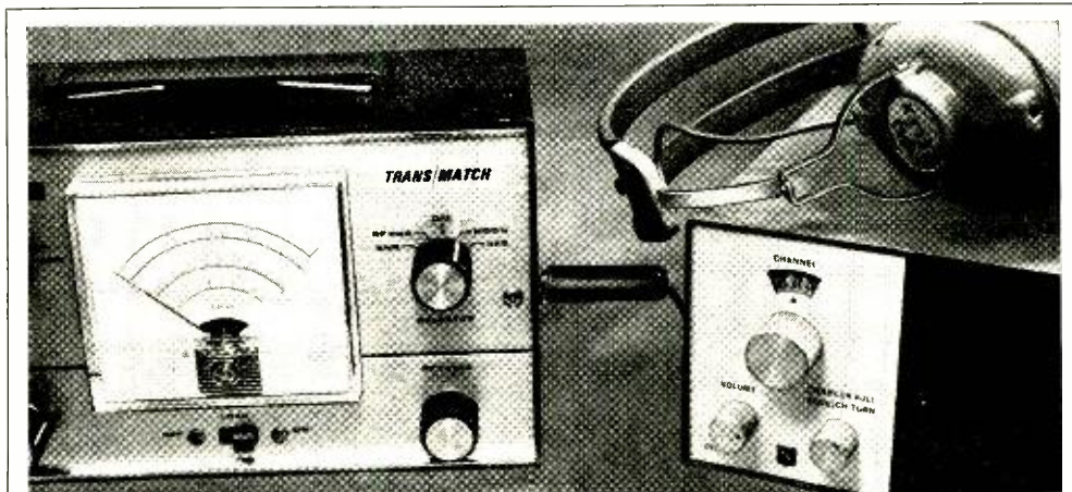
Multiple-purpose test instruments. One of the many recently introduced multiple-purpose testers is the EICO 715 "Trans/Match." Besides measuring power output in watts, serving as a field strength meter, and checking SWR when inserted in the transmission line between transceiver and antenna, the "715" will also read percentage of modulation. In this photo, a Squires-Sanders "23'er" is being tested. Headphones plugged into the side of the "715" permit an on-the-air type aural check of quality.
