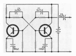
Oscillator, timing, and other tuned circuits, whose frequency of operation depend on controlled circuit values, call for stable low-loss units. In this regard, C2 and C3 are critical, whereas C1, C4, and C5 can vary considerably. Except for polarized types such as electrolytics, polarity is not a factor.
