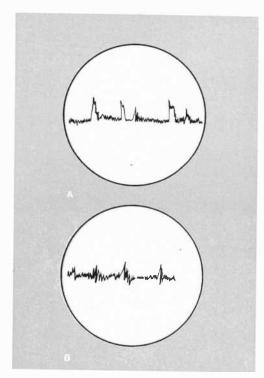
Fig. 1. Though these "pips" look like range marks or targets, they are not returns from a radar Ascope. The jumble in (A) shows the "ping" sounds that some types of fish make. In (B) is another kind of fish "chatter" which resembles plain grass.
