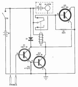
Fig. 1. This innocent-looking pool alarm circuit can be set off by just a splash of water to warn you that an intruder has entered your swimming pool.
