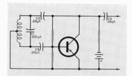
Value of C1 is critical here—both capacitor and coil determine the frequency of this Hartley oscillator. Capacitors C2 and C3 merely serve as d.c. blockers and should be high enough to offer very little impedance at the operating frequency. As with most coupling capacitors, C4 blocks d.c. and should be large enough to easily pass the signal.
