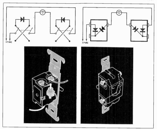
Two four-way switches (d.p.d.t.) and two diodes wired back-to-back in a two-wire circuit provide three-way light control. If the light stays on regard-less of switch position, reverse one of the diodes.
