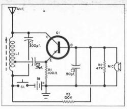
Fig. 5. Easy-to-build experimental wireless microphone submitted by reader Carl Bergquist features a single pnp transistor used as a modulated oscillator. The unit's operating range is kept limited.
