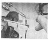
support two components or wires, two clothespins clamped back-to-back can be employed. If you don't want to use a vise to hold the clothespins, you can mount one or more pins on a small block of wood.—Robert E. Kelland
