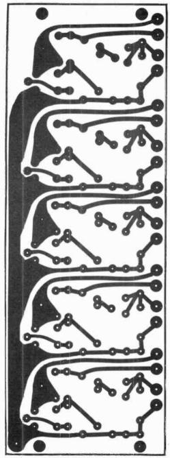
Fig. I1. Actual-size illustration of printed circuit board. For hole drill sizes, refer to Fig. 4.
