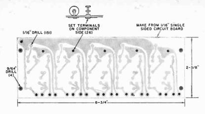
Fig. 4. Printed circuit board showing overall dimensions and drill sizes for all holes required.
