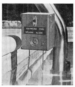
When installing the alarm, bend the probes close together and make tests to determine optimum separation. Best results will be obtained by installing the probes at the pool, with the alarm being remotely located at a convenient listening post.
