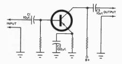
Coupling capacitors C1 and C3 in a transistorized audio amplifier generally require higher values than their counterparts in a tube circuit. Bypass capacitor C2 is not critical, but must be very high in value to prevent low-frequency degeneration. The main reason for the higher values is that transistors have a lower impedance.
