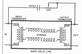
the mechanical delay without any ill effect on the lower frequency sounds.
