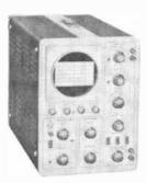
able either as a kit or factory-assembled. The vertical channel of the IO-14 has a d.c. to 8 MHz bandwidth. a sensitivity of 0.05 volt/cm a.c. or d.c., a rise time of 0.04 µsec.. a precision delay line with 0.25 µsec. delay. and a 9-position. fully compensated vertical attenuator. The horizontal channel has 18 triggered sweep rates in 1, 2, 4
