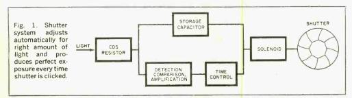
a full two minutes. Should the light level change during the exposure time, the circuit will automatically compensate for this change by making an appropriate correction in the exposure time.
