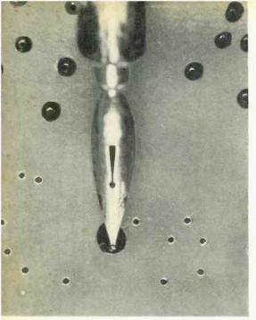
Fig. 6. Use a pen or other applicator to put on liquid resist. After all drilled holes are circled, draw lines to connect them following your sketch.
