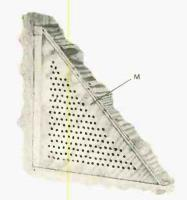
Cage side cover is held in place by 21/2"-long screws fed into front and bottom of cabinet from outside, and by 11/4" screws through piece L.
