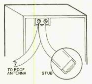
length of lead-in wire across the set's antenna terminals, letting the free end hang loosely toward the floor. Check to see if there's an improvement in the picture. Progressively shorten the stub by cutting into the insulation with a razor blade so as to short out the pair of wires. Cut the lead at the point where the ghost disappears or is substantially suppressed. Then twist the two wires together as shown.
