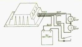
Assembling a project with a module is easy. This dual flasher needs only the module, battery, switch and light bulbs. Hard-core experimenters say that these projects offer the builder no challenge.
