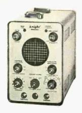
16 pounds. Identified as the Knight Model KN5005 scope, it boasts a flat frequency response within  $\pm$  3 db, from d.c. to 6 mc., and has a vertical sensitivity of 0.05 volt/division. Its horizontal circuit provides linear sweep from 1 microsecond/division to 50 microsecond/division,  $\pm$  10%, with a sweep as fast as 0.2 microsecond/division when its built-in multiplier is used.
