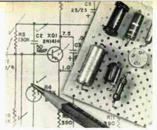
Fig. 3. Mock-up of printed circuit board showing preliminary parts layout. Terminals are interconnected in accordance with circuit schematic diagram.
