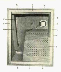
Location of tweeter is not critical. Cover side away from woofer cage and back with polyurethane foam plastic. Glue and screw all cleats in place.
