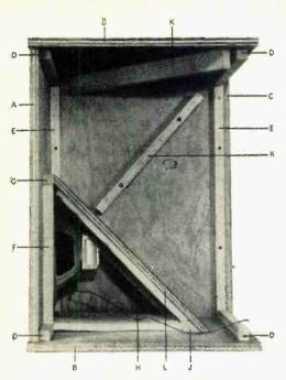
Except for the front, all inside surfaces of the woofer cage are covered with faom plastic. Loosely pack the woofer cage with a sheet of fiberglass.
