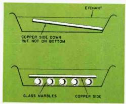
Fig. 9. Place copper surface on glass marbles in a nonmetallic tray with etchant solution at a temperature of 90° to 120°, and agitate frequently.
