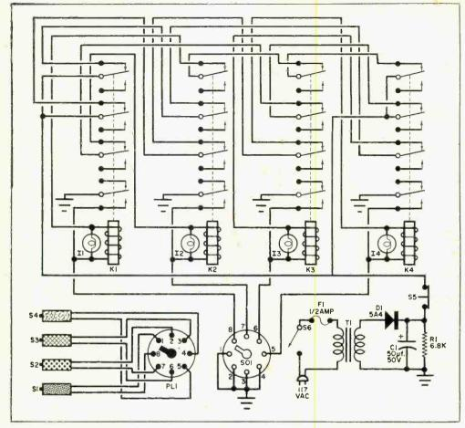
Fig. 1. Responders \$1 to \$4 can complete only one relay circuit at a time. The first switch closed latches its respective relay, lights its lamp, and disables the other relays until the circuit is reset.
