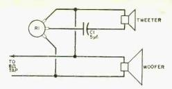
Low and high audio frequencies are separated by C1 and kept in balance by L-pad R1. For best results, the tweeter and woofer must be wired in phase.
