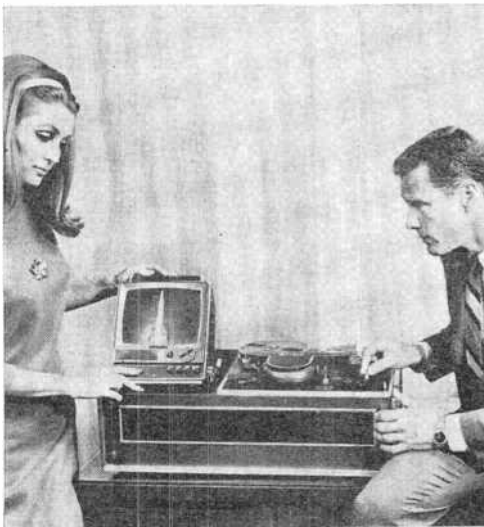
Sony's $1000 recorder is attracting considerable public attention. With a tape width of 1/2 inch and a 7.5-ips speed, the picture quality is quite good.
