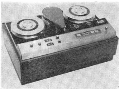
The new Ampex home TV tape recorders will sell for about $1300. This is a helical scan recorder and should be capable of recording color TV signals.
