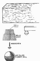
mold into place on a side of the base. Then cement the rubber ball in place inside the mold. If the sides of the base are too thin to hold the screws, you can build up the cabinet with a block of wood.
