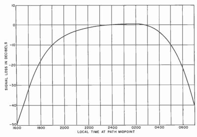
This graph, copied from CCIR Report 264, Geneva, 1964. shows the expected signal loss of AM broadcast-band signals vs. time at the mid-point of the signal path. Across the North Atlantic, AM signals should be strongest between 9 p.m. and midnight, Eastern Standard Time. Strength of the AM signal drops off rapidly after about 1 a.m. EST.
