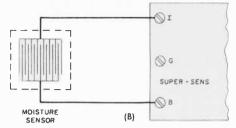
Fig. 8. These circuits can be used to control humidifiers and lawn sprinklers. Just a drop of rain on the sensor will release the relay in circuit (A). Circuit (B) can detect slightest trace of moisture.
