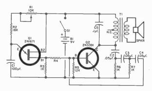
age becomes sufficiently positive, the emitter becomes forward-biased, and discharges C1 through the emitter and B1 junction and R3. The voltage drop across R3 forward-biases Q2 and turns it "on." As C1 becomes discharged, the current through R3 drops, and Q2 shuts "off."
