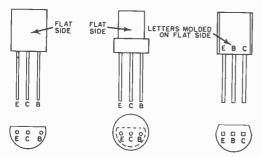
Fig. 1. Silicon transistors featuring in-line lead connections instead of usual spaced lead arrangement. Flattened side facilitates lead identification.
