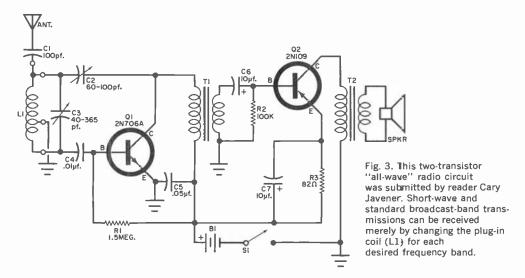
ner (Rt. 1, Box 208-A, Cameron, Wis. 54822), who submitted the general-purpose receiver circuit shown in Fig. 3. Cary says his little two-transistor "all-wave" radio does a superb job receiving amateur and s.w. bands, in addition to the standard broadcast band. The only requirement is that a new coil be substituted for each band since there are no provisions for switching.
