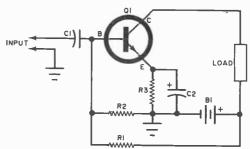
Fig. 2. Circuit configuration of typical amplifier stage using a silicon transistor. Base bias is determined by resistance ratio of R1/R2 combination.
