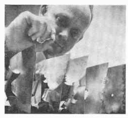
"OLD-FASHIONED" METAL SCORES COMEBACK—A pea-size pellet, traveling at meteoroid speeds, wrecked these sheets of aluminum during tests made by Boeing Company engineers in Seattle. The purpose of the tests was to find the best metal to use in building manned spacecraft. Despite the damage shown here, test results favored use of the "saucepan" material over space-age metals.
