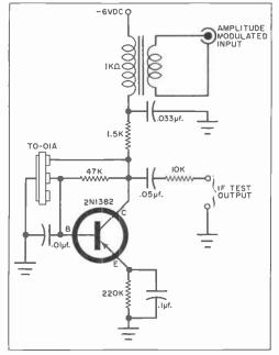
Fig. 3. Test oscillator using a TO-01 transfilter and a single transistor. The unit can be built and housed in a small pocket flashlight case, complete with penlight batteries and all, at a very low cost.
