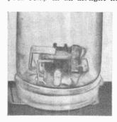
housings be made from a variety of containers such as screw cap jars. coffee cans with plastic snap-on covers, or for the really small relay, small vials. The lid, or cap, of the container with relay attached is mounted on the
