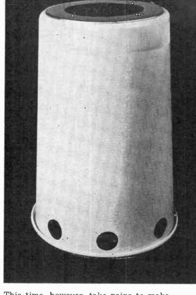
the speaker itself as a template; a paper punch or any sharp, pointed instrument will do the job.
