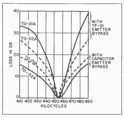
Fig. 1. Typical relative frequency response of transfilterized receiver i.f. stage. Note attenuation when Clevite TF-01 replaces emitter bypass capacitor.
