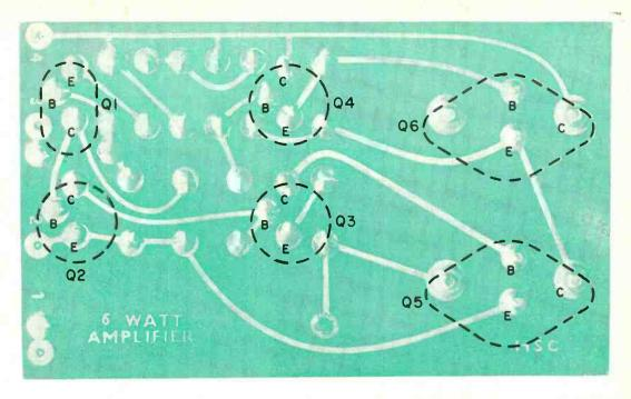
Fig. 3. Use this full-size guide in making your printed circuit board. Space the transistors about  $\frac{1}{2}$ " above the board and hold transistor leads on top side of board with a pair of long-nose pliers when soldering.
