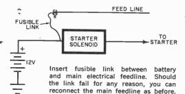
heavier, the link will burn out before the regular wiring has a chance to do extensive damage in the event of a short. At 30 or so amperes, the link runs hot; and at about 40 amperes, it quickly melts. Normal total current requirements in a car rarely exceed 30 amperes. For the system to operate again, once the link fuses, it must be replaced. Special heatresistant insulation is used to safely contain the hot link.
