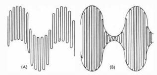
Fig. 5. These waveforms show what happens when two identical signals are handled by (A) linear (distortion-free) amplifier and (B) nonlinear amplifier.
