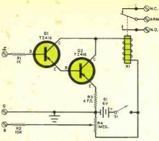
Fig. 1. As little as 0.2 μa. at 1 volt is enough to trigger relay; up to 50 megohms can be sensed.
