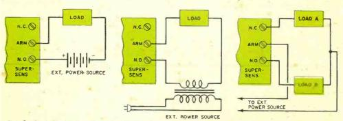
Fig. 3. Controlled external load circuit can utilize almost any source of power. If power requirements exceed the relay contact's rating, a power relay can be added. One or two loads can be switched.
