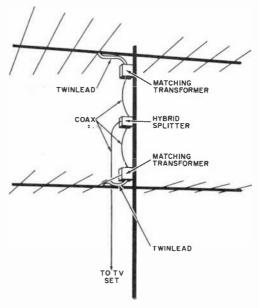
Fig. 1. Hybrid splitter allows signals from each antenna to add to each other, and minimizes loss when one antenna acts as a load on the other. Leads to transformers and splitter should be equal.
