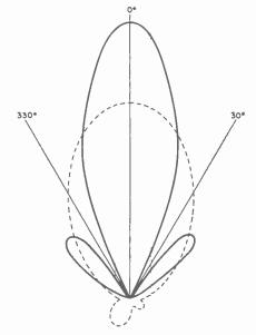
Fig. 3. Angle of null points can be changed by adjusting the spacing between horizontally stacked antennas (solid line) to drop out interference. Dotted line is response curve of single antenna.
