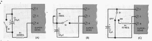
Fig. 6. An RC network can be added to make a time-delay relay. Circuits (A) and (B) stay on for a desired time after the switch is opened. "Turn on" is delayed in circuit (C) when the switch is closed.
