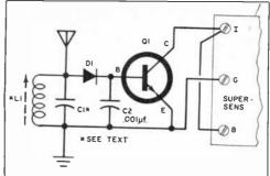
Fig. 10. Radio control can be achieved with simple detector. Tune C1, L1 to desired frequency.
