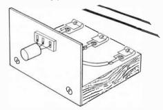
wood measuring approximately 3½" x 3" and attach it to a metal plate of the same size. Mount a transistor socket on the plate and connect the socket terminals to three Fahnestock clips on the block as shown. Material and dimensions are not critical.
