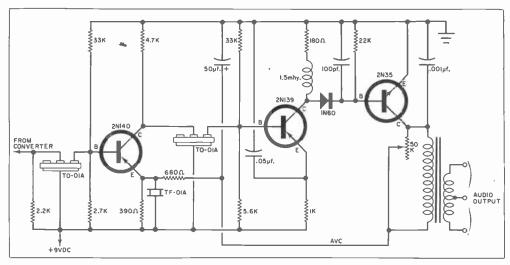
Fig. 2. This transistorized circuit uses transfilters in place of conventional i.f. transferriers. Insertion loss is less than 3 db, and bandwidths of from 4 to 10 kc. provide a selective or high-quality i.f.
