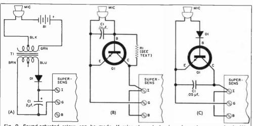
Fig. 9. Sound-actuated relays can be made. If microphone is low-impedance type, use circuit (A); high-impedance pickups work well in circuit (C); a low- or high-impedance unit can be used in circuit (B).
