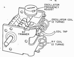
Fig. 2. These components determine the operating frequency of the tuner. The coils are adjusted by compressing or expanding the turns as necessary for good frequency coverage and tracking in the band.
