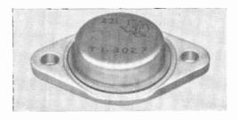
without any heat sink whatever, it could run at a 2-watt continuous power level.
