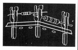
Fig. 8. These Vector connectors feature serrated slots for the component leads. Connectors can be soldered if desired.
