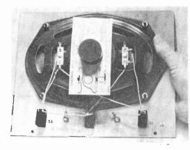
The input jacks on either side of S2 can be eliminated by connecting the test leads directly. Before mounting, check voice coil phase and wiring details.
