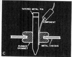
Fig. 6. Solderless connectors using rubber-like materials. Shown are (A) ETA's "Flexi-Klip" rubber sleeve type, (B) tube and cup type, and (C) PIC's grommet and pin type.
