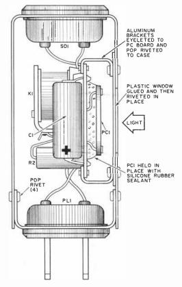
Fig. 6. After all the parts are preassembled on the circuit board, and the unit has been fully wired and tested, install the plastic window and pop-rivet the aluminum brackets to the case shield.
