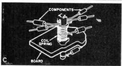
Fig. 5. Solderless connectors using wire springs.
