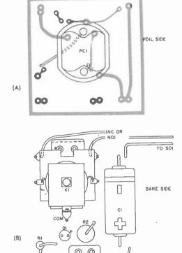
Fig. 5. Here's the component layout. Photocell PC1 is mounted on the foil side of the circuit board as shown in (A). All of the other parts are mounted on the bare side of the board as shown in (B).
