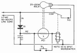
Fig. 7. This low-cost touch control circuit can easily be wired to any desk or table lamp by adding a microswitch across PC1. To turn on lamp, touch S1 gently. To turn off lamp, bring hand near PC1, shielding it from light. For proper operation, PC1 must be shielded from other strong light sources.
