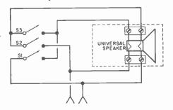
The two 20-ohm voice coils are tied together: in series by S3 to effectively obtain 40 ohms impedance; and in parallel by S1 and S2 for 10 ohms. Either S1 or S2 alone provides a 20-ohm speaker load.
