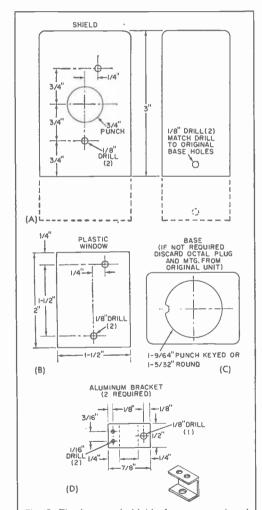
Fig. 3. The base and shield of case are cut and punched as shown. Then they are finished with lacquer or paint, or are anodized. The two brackets at bottom are made from 1/32-inch aluminum sheet. Window is made from heavy plastic film such as Mylar; avoid using brittle material.
