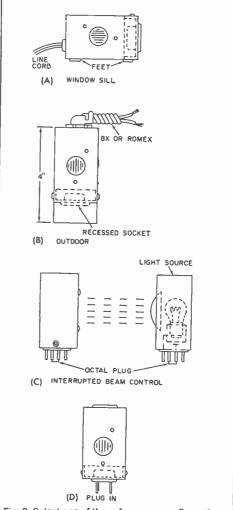
Fig. 2. Select one of these four case configurations for the Dusker. For table or desk lamp touch control applications, the outer casing is not used.
