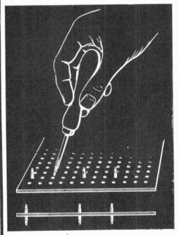
Fig. 4. These Vero connectors feature terminal pins with self-cutting serrations.
