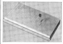
Fig. 14. Components are assembled on Vicon "Proto-Board" by inserting their leads into the soft material comprising the plastic base.
