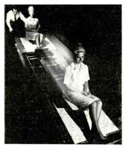
RIDING ON AIR—Principle of magnetically floating transit cars is demonstrated by Westinghouse test vehicle above. In a full-scale system, the frictionless floating cars would be driven at speeds in excess of 150 m.p.h. by a linear electric motor.
