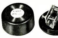
Both R1 and D1 can be mounted under buzzer cover.
