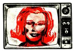
Some reflected signals may not be bad enough to create much of a disturbance on a black and white picture, but can cause intolerable color distortion.
