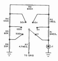
Fig. 3. Alternate hookup of voltage divider provides extra 0- to 1-volt range.
