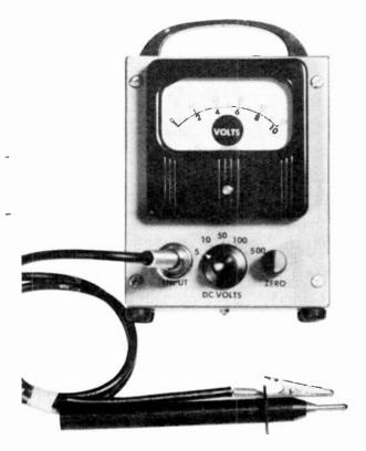
Unit measures voltage in a.g.c., grid bias, oscillator and other high-impedance circuits without loading
