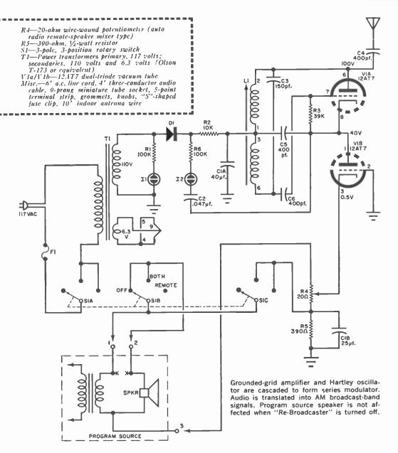
grounded-grid amplifier. The grounded grid shields the input from the output circuit and prevents oscillation. Input signals applied to the cathode vary cathode potential with respect to the grid in "step" with the signal. This action varies and controls current flow through the tube, making the tube work like an ordinary amplifier.
