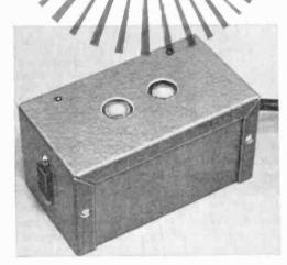
Point the "eyes" away from direct light to automatically compensate for varying ambient light levels.
