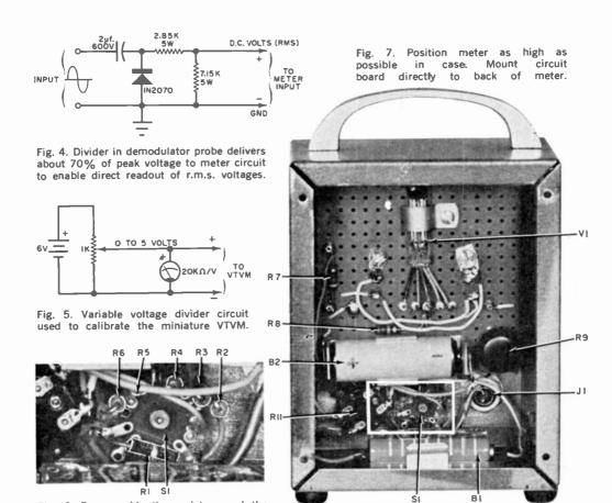
Fig. 6. Preassemble the resistors and the switch in "turret" fashion before mounting.
