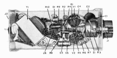
Locate T1 as close to the back of box as possible; note location of tube sockets, and mounting hole for C6. Jack J2 (for strobe connection) is hidden at rear of box.
