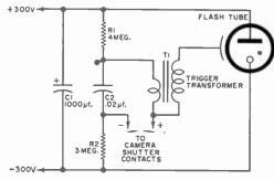
Flash shutter contacts are polarized. Check with a voltmeter, and connect positive side to V2's plate.
