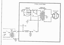
a filament transformer with a voltage equal to the radio's original working voltage-6 or 12 volts-and with a current rating that equals or exceeds the radio's battery drain current (usually 6 or 7 amperes for a 6-volt set, half that for a 12-volt set). Connect
