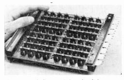
Electromagnetically operated reed switches replace conventional relays in the "No. 1 Electronic Switching System." These switches respond to commands from the central control and connect telephone subscribers to trunk lines.
