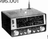
• Reliable 10 transistor, 6 diode circuit • Fixed-aligned ceramic 1F "Transfilters " • Covers 550 kc to 32 mc in five bands • 50-inch telescopic whip antenna • Zener diode voltage regulation • Smooth, easy flywheel tuning • Built-in 4" x 6" speaker • Large, slide-rule dial for easy station selection • Headphone jack for private listening • BFO for code & SSB transmissions • Compact & battery powered for portability, yet can operate on 117 v. AC with optional XP-2 accessory (a \$9.95)
