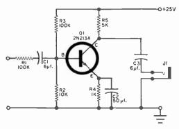
Harold Reed's impedance-matcher enables use of low-impedance headphones in high-impedance audio circuits without excessive loading. A potentiometer in place of R5 could serve as a volume control.
