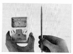
A NEW application has been found for the temperature-sensitive thermistor, a semiconductor. Braun Electronic, a West German firm, has put it to work in a medical thermometer that accurately gauges a patient's temperature in seconds. Named "Tastomed," the device has a probe which is held under the patient's tongue, and a meter calibrated in Centigrade and Fahrenheit. U.S. representatives: Electro-Physical Instruments of Ogdensburg, N.Y.
