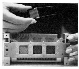
Temporary memory in the No. 1 ESS is made up of Western Electric ferrite plates, each containing 256 holes carefully laced together with sense wires. Magnetic material surrounding each hole stores a binary code signal to record subscriber line usage and numbers of the called and calling phones.
