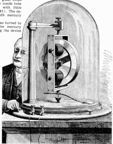
Several types of gyroscopes were used for classroom demonstrations of the earth's rotation, among them the battery-powered version shown at right. Other units were powered by steam or with a crank.
