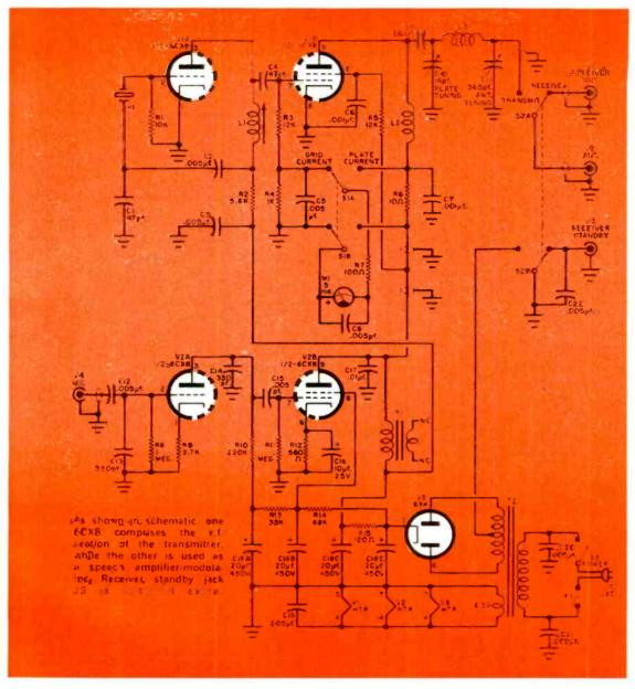
and taped. In completing the Companion Transmitter, make sure the meter switch is labeled correctly: "G" for grid drive and "P" for plate current. Drill a  $\frac{3}{8}$ " hole in the top of the box for adjusting grid drive coil *L1*, and cut a row or two of holes in the back of the box cover for ventilation.
