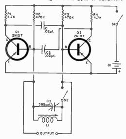
The code practice oscillator (CPO) circuit in Fig. 3 was submitted by reader Mark Humphries (553-31st St., Manhattan Beach, Calif. 90266). According to Mark, his circuit will deliver ample power for group practice.
