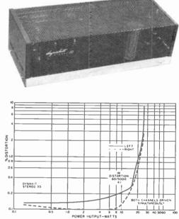
Intermodulation distortion as measured by the Hirsch-Houck Laboratories was below 0.5% for all output levels up to 17-18 watts output per channel.
