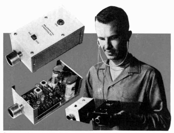
The ultrasonic transmitter is mounted in the same case as the Sniffer. The board is held by spacers and the batteries are clamped to the rear wall with spring clips.
