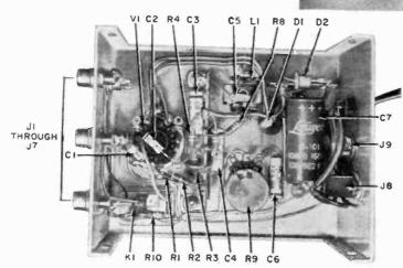
Indicator lamp jack is connected to miniature plug so lamp can be mounted at tuner or amplifier panel.
