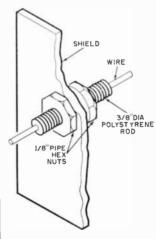
pipe hex nut in a vise, and chamfer the the end of a % " polystyrene rod. Thread the rod by screwing it into the nut, making sure to get the thread started right. Cut the threaded rod into 3/4 " lengths and drill through it with a  $\frac{1}{16}$ "-1/8 "-diamto eter drill. Then
