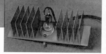
with two  $4-40 \ge \frac{1}{2}$ " round-head bolts and nuts. Don't forget the nylon washer to insulate *PC1* from the heat sink. Block off the two open sides of the heat sink with pieces of scrap aluminum and fill in the boxed area with an epoxy such as Castolite. After allowing the proper curing time, paint the encapsulated area with several coats of black paint to prohibit incident light from affecting the
