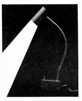
right on the seam of the can for best appearance. Center-punch all holes before drilling, and work carefully as the metal is soft and thin. Then deburr the holes with a large drill, and paint the outside of the can—the author used bright gold Krylon spray, but any color could be used. When the outside paint has dried thoroughly, carefully mask the entire outside of the can, and spray the interior a gloss white.
