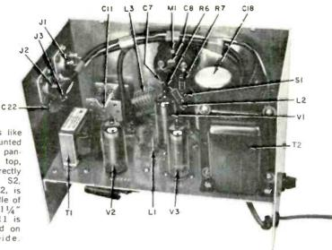
Top of rig looks like this, with M1 mounted at center of front panel and  $\frac{1}{2}$ " from top, S1 and C10 directly below it. Switch S2, hidden behind T2, is mounted in middle of panel and about  $\frac{11}{4}$ " in from side; C11 is similarly mounted on the opposite side.
