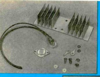
Assembled heat sink is shown below, before encapsulation and painting.
