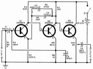
Fig. 2. Hi-f phonograph preamplifier circuit developed by General Electric employs three of its low-cost epoxycased silicon units. Transistors Q1 and Q2 serve as high-gain common-emitter amplifiers and transistor Q3 as an impedance-matching emitter-follower.
