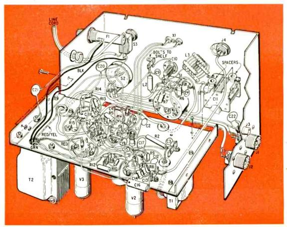
from receive to transmit. A 6X4 rectifier (V3) and the *RC* filter circuits of *C18* and *R13*, *R14*, *R15* deliver the required B-plus voltages to the transmitter circuits.
