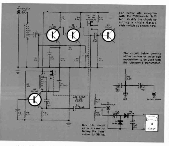
L1 until it is raised flush with the top of the coil housing can. Now reverse the direction of slug travel and turn the slug three turns back into the coil. Set R4 at about one-fourth turn from the counterclockwise stop.
