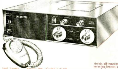
Small, Compact Measures Only 1174 Wx6734 Dx37H Law Current Drain . 350 ma on Receive, 850 ma on Transmit
