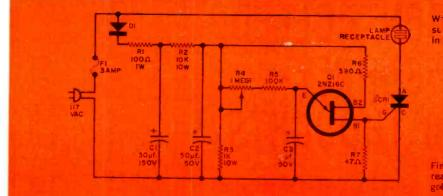
When wiring the unit, be sure that no parts come in contact with chassis.
