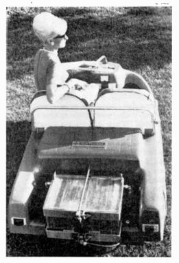
This fuel-cell-driven golf cart made by Allis-Chalmers shows the feasibility of putting fuel cells to work powering vehicles. A fuel-cell-operated farm fractor was demonstrated by firm as early as 1959.
