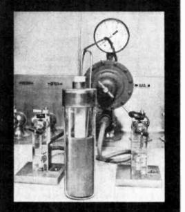
Below is a cutaway mockup of one of the fuel call canisters installed in Gemini. Fuel call modules — the first may be in orbit when you read this —produce drinking water for astronauts as well as up to two kilowatts of electrical power.
