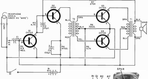
Fig. 4. A typical audio amplifier circuit for demonstration purposes. Breadboarded version appears at the right. See Transitips for details.
