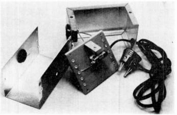
Unit is shown open at right, with back of terminal board. Angle bracket supports board, resistor R2 mounts on reverse.
