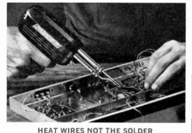
Wires or leads will then become hot enough to melt the solder and it will flow into the joint. Never apply heat directly to the solder.
