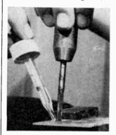
the tap breaks off. To prevent this sort of tragedy, try using carbon tetrachloride as a tap lubricant. Because of its high rate of evaporation. neither gumming nor binding will occur. and you'll have a cleaner job. The carbon tet
