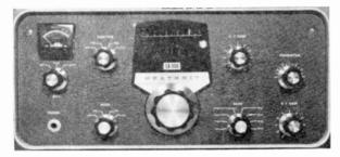
both during the course of a single evening. The average ham should be able to align the SB-300 in less than two hours, using either the built-in 100-kc. crystal calibrator or a standard signal generator as the signal source. Also required is a vacuum-tube voltmeter to measure the crystal-oscillator d.c. grid voltage (at a test point) in the preliminary oscillator adjustment.
