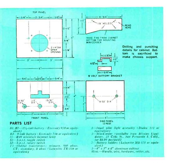
volts for the light. Connect the black primary lead and green secondary lead of T1 together and to ground. Connect the hot speaker terminal to switch S2's wiper with shielded wire, and the Min-Corder signal lead to one switch terminal along with the brown secondary lead from T1. The primary green lead from T1 goes to the other position of S2.
