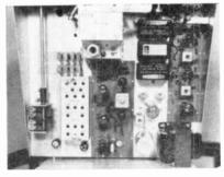
Inside and outside views of the Heathkit SB-300 receiver. Although there are more steps to complete than with the average kit-type unit, the SB-300 is not difficult to assemble. Printed-circuit boards are used in the critical r.f. and i.f. sections.
