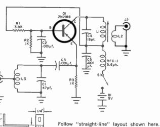
Follow "straight-line" layout shown here. Leads must be kept short for good results. The positive battery terminal is grounded.
