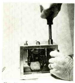
After wiring, fasten all components in place.
