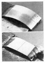
The entire story becomes dramatically clear when we compare heavily worn head (lower) with new one. Note how abrasive tapes have worn down the head, widened recording gap. Uneven wear characteristics are caused by improperly slit tape. Note, too, the accumulation of oxide in the gain and around the head. This head is useless!
