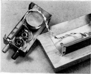
C1--0.1-µJ., 600-volt paper capacitor J1--Closed-circuit phone jack (key) J2--Open-circuit phone jack (phones) R1--20,000-ohm, 5-watt wire-wound resistor R2--100,000-ohm, 5-watt wire-wound potentiometer (Centralab WW-104 or equivalent) 1--Fluorescent lamp (GE T-8 recommended) 2--Fluorescent lamp (tombstone" connectors 1--1½" x 2¼" x 4¼" aluminum Minibox 2--Insulated binding posts
