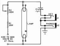
lamp oscillated, the GE 15-watt T-8, which is one-inch in diameter and 18" long, was found to be the most practical.
