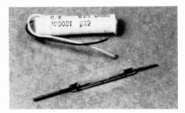
Magnetic reed switch (above) slips into center of the coil which applies electromagnetic force to operate the switch. of the cell and thereby reducing its shunting effect on L1, causing more current to flow through it. When the light level is sufficiently low, the field generated by L1 becomes strong enough to cause switch S1 to close as the magnetic switch is mounted in the coil. When the switch operates, it closes the 117-volt circuit to the socket, turning on a small lamp that's plugged in.\*
