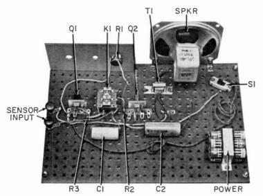
Transistor Q2 is employed as an audio oscillator in the rain alarm, with the primary of T1 serving as its collector load.
