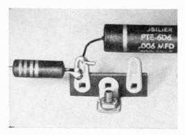
Crimped resistor (left, above) is on its last assignment. Lead is too short for a salvage operation, mechanical connection too tight. Compare with capacitor (above, right).
