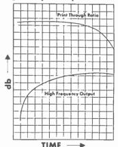
Notice how severely high frequencies suffer if milling time is too short; how print-through is degraded with prolonged milling.
