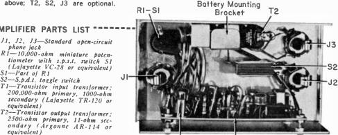
Follow parts placement indicated (unit is inverted in this photo) to avoid possible feedback problems.
