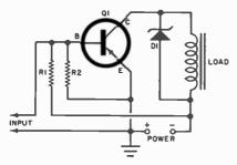
Fig. 2. Typical circuit for damping out excessive transient voltages uses zener diode (D1) to shunt the inductive load.
