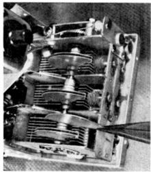
removing the screws at the sides and back. Rotate the tuning capacitor so the plates are fully unmeshed. You will notice that all the rotor plates, except the one at the left, are tied together at the tip with a support. Using a wire cutter, clip the support between them except for the last two on the left in each section.
