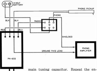
Toggle switch S1 supplies the signal from the phonograph arm or the tuner to the amplifier.
