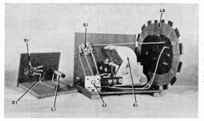
Looking at the backs of the two couplers diagrammed in Figs. 2 and 3, it's obvious that there isn't any complex wiring to be done. Use point-to-point wiring throughout, build panels of Masonite, wood scrap.
