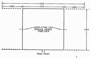
The end ½-wavelengths (shown by the dashed lines) of two ½-wave dipoles are bent towards each other and joined to form a quad antenna element. Gain: 0.9 db.
