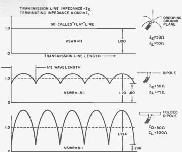
The VSWR is determined by the impedance of the line termination and the impedance of the transmission line as in several examples at left. To simplify things, line losses are not included in figures.
