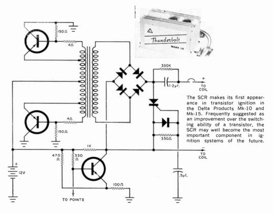
In this Slep TS-30 system, two transistors were tied in parallel. This company offers a variety of systems up to and including a 500:1 model.
