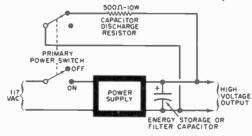
SUPPOSEDLY dead power supplies can give you quite a jolt—filter capacitors will store a lethal charge for days, and high-capacity electrolytics such as those used in electronic flash units can give you a painful shock even months later. A simple safety device that will act as a bleeder even if the regular bleeder resistor fails is diagrammed at left. Simply add a resistor and use a d.p.d.t. on/off switch.
