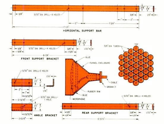
Easily worked aluminum is used for fabricating the pickup. The tubes can be conveniently cut from ten 6' lengths of  $\frac{3}{8}$ " diameter stock, the support brack-
