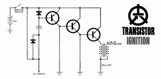
Nuclear Electronic Laboratories Inc. (N.E.L.I.) developed its "Trans-nition" circuit using three transistors cascaded (four in positive ground version). Point current is reduced to under 12 ma. and special 260:1 coil must be used.
