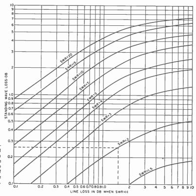
Transmission line power loss is increased with an increase in standing waves. Note that the loss can be more than doubled if high standing wave ratios are on the line.
