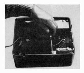
Locate a convenient spot under the turntable, and mount the tuner on brackets; add switch.
