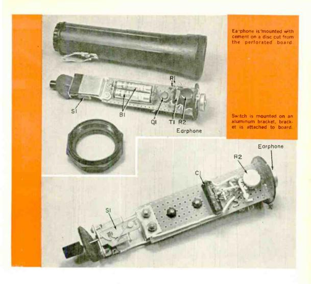
Looking at front end, earphone which is used as a small speaker is protected by flashlight glass disc.
