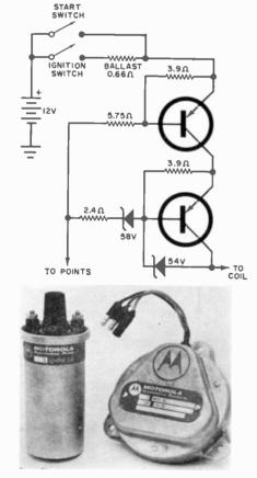
This Heathkit GD-212 system differs slightly from the Motorola unit at the bottom of the page so far as parts values are concerned. and uses slightly different transistors. The coil ratio in this circuit is 250:1. Meter is used to establish current in ignition coil. START SWITCH IGNITION BALLAS' IOΩ-IW 100 W 5.5Ω 12 V IOW 10Ω-IW 5Ω 56V TO POINTS
