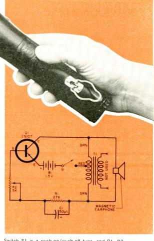
Switch S1 is a push-on/push-off type, and R1, R2, C1 determine frequency varied by potentiometer R2.
