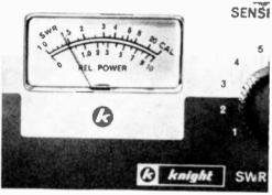
Three different SWR meters were inserted in the same line one at a time. Notice the close similarity in readings that was obtained. The Heathkit AM-2 (top) and the General Radiotelephone Co. 615 are one-piece types in which the transmitter connects to the input, and the transmission line to the output. The Knight-Kit P-2 SWR/power meter has a separate unit that connects into the transmission line; unit shown contains meter and controls.
