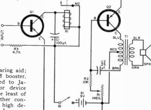
"eye-glass" type transistorized hearing aid; and a transistorized all-band FM booster.
