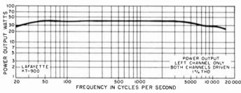
This power response curve was made with both channels driven. Output was measured with a simulated 8-ohm load. Considerably more power output can be obtained by driving one channel and leaving the other quiescent, which may account for the discrepancy between the manufacturer's claim and the results that are shown here.
