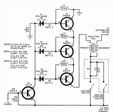
This schematic shows the wiring of either a 12- or 6-volt positive ground ignition system. Cars with 6-volt batteries do not have the ignition starting switch, or resistor Rb and capacitor Cn shown within the dashed lines. The ignition switch in 6-volt cars connects directly to the coil. The capacitor which shunts the breaker points must be removed in all cases.
