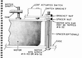
Fig. 4. Use of spacer tube and nut will avoid risk of bending motor case and misaligning cam.
