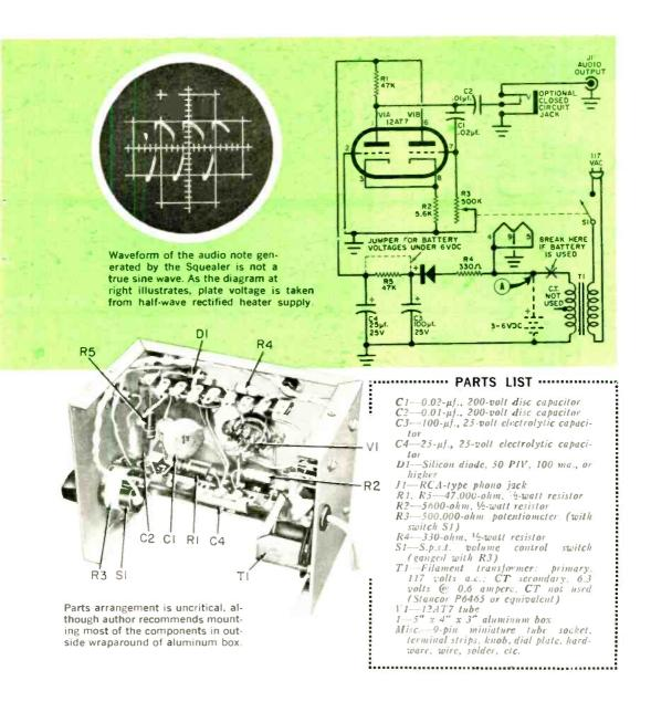
the box opposite the transformer. Since no pilot lamp is employed, a dial plate is used with the potentiometer as an on-off indicator and to spot the different output frequencies.
