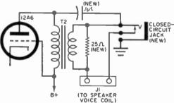
"Command" receiver by adding a .1-µ1., 400-volt coupling capacitor, a 27-0hm, 2-watt voltage limiting resistor, and a closed-circuit jack to the audio output circuit. This scheme will work best with high-impedance headphones. Although it might be possible to squeeze the jack on the front panel, a better way is to mount it in a small Minibox.
