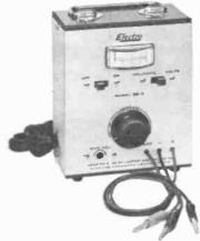
meter and can supply 0-20 volts of well filtered d.c. at currents of up to 150 ma. (or 24 volts at 100 ma.). The output voltage is continuously adjustable over its range. In addition, a separate adjustable bias output of from 0 to 6 volts is available. Model EC-3 is supplied with pre-attached clip leads.
