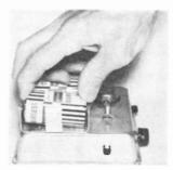
equipment. In addition to scraping the contacts of the batteries and holders, you can do a quick, in - the - holder cleaning job by grasping each cell with your thumb and index finger and
