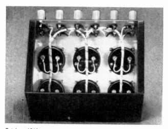
Mount the six meters in a logical pattern so that the scales increase from left to right and top to bottom. Bring the meter leads out to insulated terminals or binding posts on the top ledge of the cabinet. Use color-coded terminals so that red indicates the plus meter lead and black the minus lead.
