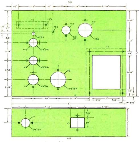
All chassis dimensions are based on California Chassis Type A-120. Since this unit may not be available from some suppliers, two alternatives are given in the Parts List. Both are larger in width and depth by one inch. The builder can easily compensate by centering cutouts on the slightly oversize chassis. Square cutout for T7 may not be required if one of the alternative power transformers is selected.
