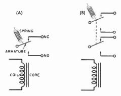
Fig. 3. Symbols for electromagnetic (A) s.p.d.t., and (B) d.p.d.t. relays. See Transitips for information on how to select substitute relays.
