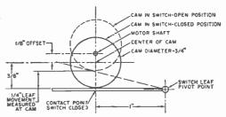
Fig. 3. Dimensions shown must be followed closely to insure correct cam and switch action.
