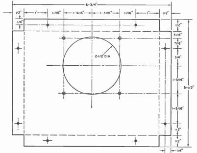
The builder will need six sheet aluminum panels for the three modules. The front panel on the audio module requires a speaker cutout; the back panel is plain. Buy the chassis before cutting out your panels to be sure they fit—see text.
