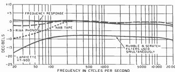
In this family of curves, the overall frequency response is compared with RIAA phono equalization. Tape equalization appears somewhat inadequate below 200 cycles. The use of both rumble and scratch filters simultaneously lessened the effectiveness of the scratch filter which, used alone, worked well.
