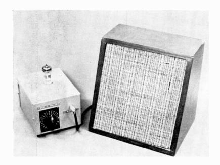
Coupled to a 3-transistor amplifier in the speaker enclosure, the Squealer had a resounding wallop. If the Squealer's output circuit was broken with a telegraph key, this arrangement could be used for code practice.
