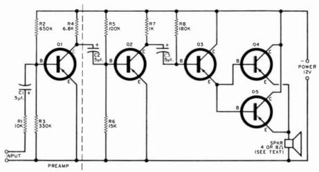
Fig. 2. Medium-power audio amplifier circuit submitted by reader Norman Huffnagle uses five pnp transistors. Modifications can be made to suit individual needs as described in text.
