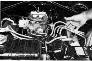
Newly shielded spark plug leads are clamped together and attached to a special shield bracket at the distributor. The kit does not include bypass capacitor for generator or voltage regulator.
