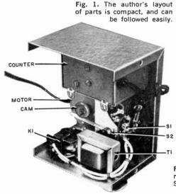
Fig. 2. Mechanical mounting of motor and switch S2 must maintain alignment.
