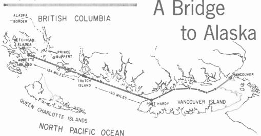
The tropospheric scatter network has two legs with a central relay as shown by the map (the link from Port Hardy to Vancouver is conventional microwave). Each antenna—see photo at right—weighs 70 tons and is built of galvanized steel sheets to take winds up to 120 m.p.h.
