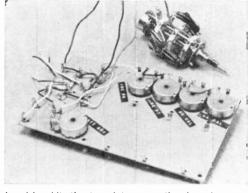
In wiring kit, the transistor mounting board comes first, then the Range and Battery Off switches.
