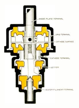
High transconductance, close element spacing, and very low lead inductance are the design factors responsible for the good performance of the light-house tube at frequencies up to 3000 mc.
