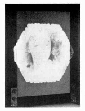
projected—in reduced size—onto the polished end of a glass rod fiber optic element. The image is transmitted through the 6" fiber optic path and then projected through an enlarging lens onto a small viewing screen.
