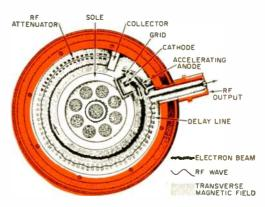
Wave motion in the backward-wave oscillator is in the opposite direction to wave motion in other traveling-wave tubes, but the principle is the same.
