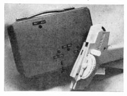
The small size of the DeVry TRVM can be realized by comparing it with an ordinary wrist watch. Test lead input jacks are mounted just below the Function and Zero Adjust knobs.
