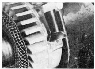
A tachometer based on a pickup is easy to construct following the information in the text. Either the relative or—with calibration—actual rpm can be read.
