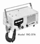
3-channel, crystol-controlled transmit and receive; universal (117- and 12-volt) transistorized power supply; 11-tube performance superhet (1 r.f. and 2 455-kc. i.f. stages); series noise limiter; adjustable squelch; ceramic mike; pi-network output. Accessories: field strength meter (\$6.95) and various
