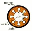
The multi-cavity magnetion has advantages that are important in practical radar applications.
