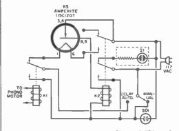
circuit causes constant recycling of K2 and K3 with the switch in manual position.
