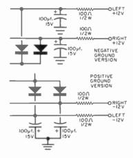
engine is running. A remedy is to add two RC filters to the device to filter out such "hash" as shown in the diagram.
