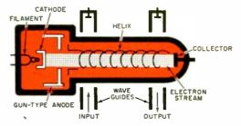
Traveling-wave tube provides broadband amplification in the 3000 to 50,000 mc. frequency range.
