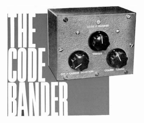
This stable "front-end" BFO makes CW and SSB sets out of marginal receivers
