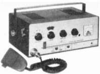
receiver; universal power supply (117- and 12-volt); 9-tube performance double-conversion superhet (1 r.f. stage), 1650-kc. conversion, 455-kc. conversion and i.f. stage); crystal-controlled second oscillator; gated-audio noise-limiting squelch system; 5-meter; ceramic mike, pi-network output; no relays—electronic switching; 12 3/16 x 5/g x 9 7/16; 13 lb.
