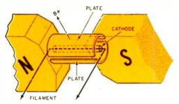
For efficient magnetron operation, a definite relationship between plate voltage and magnetic field strength in the interaction space must always be maintained.
