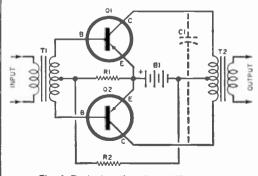
Fig. 4. Typical push-pull amplifier stage.
