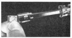
steel and grind the opposite edges parallel so that each blade is a snug push-fit in one of your hex-nut drivers. Then grind the end to leave  $\frac{1}{8}$ " to  $\frac{3}{16}$ " projecting. Finally, grind the tip to the thickness you need for those special narrow or broad screw-slots.
