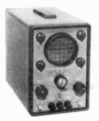
from 2 cps to 500 kc., and horizontal response from 2 cps to 300 kc. Vertical sensitivity is 25 millivolts per centimeter, and the horizontal sensitivity is .25 volt r.m.s. per centimeter. Synchronization is fully automatic on all ranges from 10 cps to 100 kc. Special features of the lightweight unit (11 pounds) include
