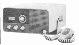
10-channel, crystal-controlled (frequency synthesis) transmit and receive, plus tunable receiver; universal pawer supply (117- or 12-volt); double-conversion superhet (1 r.f. stage, 1650-kc. conversion plus 1 i.f. stage); noise limiter; adjustable squelch; carbon mike; pi-network output; 5-meter and modulation indicator; 101/<sub>8</sub> x 51/<sub>8</sub> x 107/<sub>8</sub>; 18 1b.
