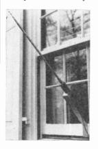
The antenna operates on six different bands-2, 6, 11. 10, 15, and 20 meters-by virtue of a shorting bar for 2 and 6 meters. and small interchangeable coils for the other bands. Rated at 175 watts PEP and 100 watts for AM, the antenna extends to 60 inches. Included in the package are 10 feet of RG-58A/U transmission line,
