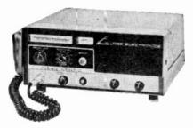
11-channel, crystal-controlled transmit and receive plus tunable receiver; "spotling" switch; universal power supply (either 117- and 12-valt, or 117- and 6-valt ovoilable at the same price); 14-tube performance double-conversion superhet; series noise limiter; adjustable squelch; ceramic mike; speech clipping and filtering for effective modulation; pi-network output; S-meter; 11½ x 4½ x 10; 16 lb.
