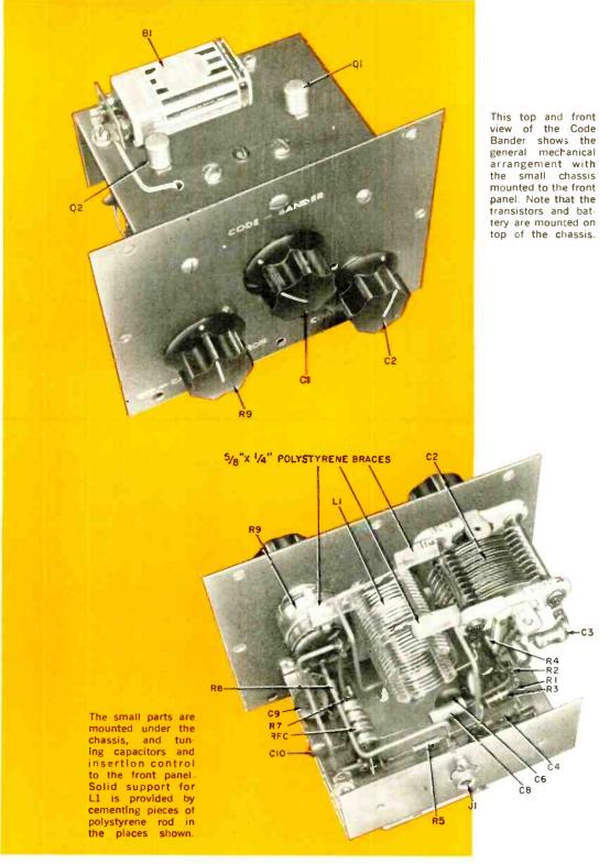
20, and 15 as well. Control R9 adjusts the output so that optimum balance between the received signal and locally generated carrier can be achieved.
