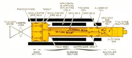
The image orthicon is one of the most complex, precise vacuum tubes in common use.
