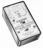
battery supply; can be used as crystal-controlled signal generator with tone modulation; built-in loop will detect r.f. fields near base of antenna; cable connections permit use as remote r.f. indicator; may also be used to check modulation; plate current, etc.
