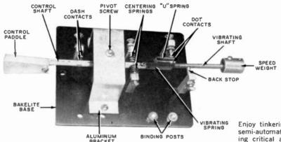
Enjoy tinkering? Try building this semi-automatic key. There's nothing critical about the parts—use what you have on hand. Properly built and adjusted, the key is capable of good c w. from 10 wpm up.
