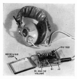
Plastic box houses wireless earphone (above); loop is wound around cover. Below is external view of combination unit; note tuning dial on side of cabinet.
