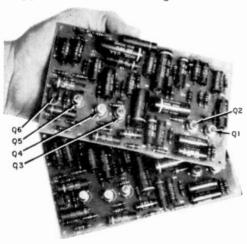
The tetrode transistor output stage provides constant voltage independent of load resistance and signal frequencies. The speaker impedance determines maximum power output. This also means that the user connects his speakers to the four speaker terminals and forgets tubestyle matching problems.
