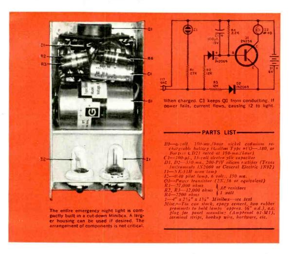
nents are larger than absolutely necessary. Only a little over 3 ma. flows through the battery charging circuit, and about the same current is required to keep the capacitor charged. Obviously, half-watt resistors are adequate, but one-watters have a longer life potential. Likewise, the capacitor, transistor and rectifiers are all over-rated for the job. This is one way of building in dependability.
