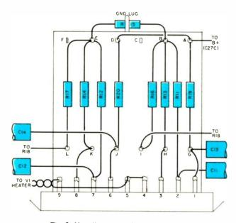
Fig. 6. Mounting turret detail at tube V2.
