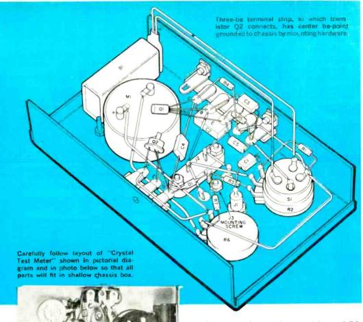
**Operation.** To check a crystal, turn on switch S1, keeping "Level" potentiometer R2 turned all the way down. Then set meter M1 to zero indication by means of "Zero Adjust" potentiometer R6. Plug in the crystal and slowly advance R2 until you observe an indication on M1.
