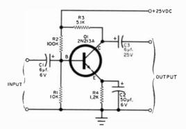
Plug-in module (far left) utilizes a mere handful of components connected to the pins of a defunct miniature tube. Schematic diagram (above) calls for 25 volts of B+, which can be tapped from most power supplies.
