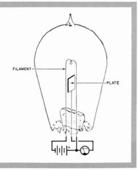
It all started with Edison's observation that electric current flowed back to the battery in this experimental light bulb.
