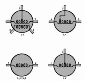
the entire coil in molten paraffin for several seconds. When the wax has dried, remove the Masonite ends and cover the end windings with a coating of cement. Slip on the collar, solder the leads, and cement the collar in place. Give the coil a second dipping in molten wax for about ten seconds, and then push on the mounting clip. This second coating is especially important for L3, since its two windings will be at a 250-volt differential.
