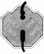
Fig. 4. This drawing, based on a microphotograph, shows the "leaf" configuration of the new line of Bendix planar transistors, with base and emitter leads attached.
