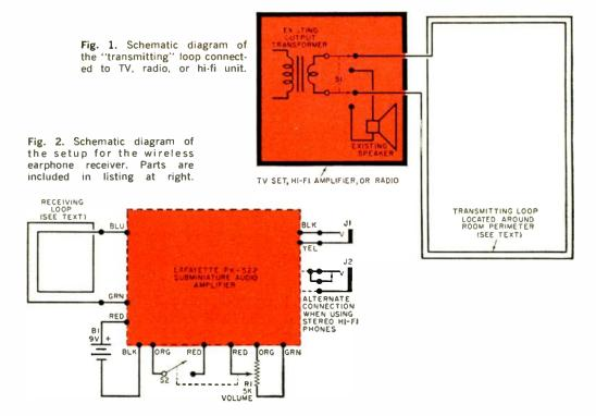
the miniature receiver in his pocket or place it on a table next to his chair. The amplifier or TV set "broadcasts" an audio signal that is inductively coupled to the listener's receiver through a loop antenna placed under the living-room rug. In this way, the listener has complete freedom of movement and trailing wires are eliminated.
