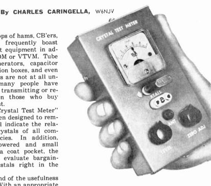
detected by diode D1 and amplified by transistor Q2. Meter M1, in Q2's collector circuit, then shows a reading which indicates the relative activity of the crystal.
