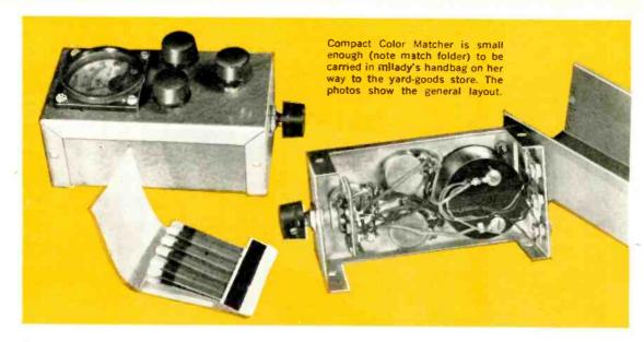
shunt for a selected deflection, then making the same adjustment for green and blue. When another color sample is substituted, the three readings will be the same if the color is the same, or will indicate a mismatch and excesses or deficiencies of red, green, and blue. The three controls can also be set for a standard deflection while viewing a plain white surface; relative red, green and blue readings will then be obtained with color samples.
