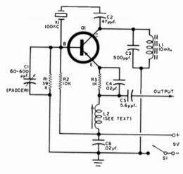
frequency inverse feedback to reduce stage distortion. Capacitor C1 serves as an input coupling and d.c. blocking capacitor. Operating power is supplied by B1, controlled by on-off switch S1.
