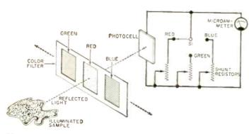
Basic color meter circuit is shown at left; its operation is similar to that of a light meter. The author's model differs in detail—three photocells with fixed filters are used, making a cumbersome, costly, filter switching arrangement unnecessary.
