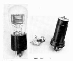
Gone but not forgotten are these three pioneers. The 200A (left) was one of the first mass-produced tubes. A 954 Acorn relped introduce VHF to communication services. At right is an 1851, a superhigh-gain tube developed just before World War III.
