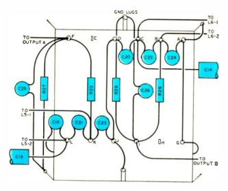
Fig. 5. Mounting post detail for filter section.
