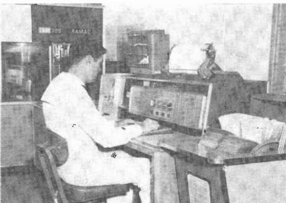
Operator at console of RAMAC electronic computer instructs machine to locate and type out information previously stored on magnetic "memory" tracks.
