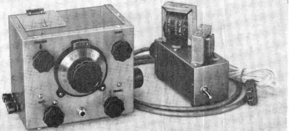
All-wave receiver and its power supply, ready for use. Since power requirements are comfortably low (about 150 volts d.c. @ 25 ma., and 6.3 volts a.c. @ 1.0 ampere), you may be able to "steal" the power from an existing receiver or amplifier and thus save yourself the trouble of building a separate supply.
