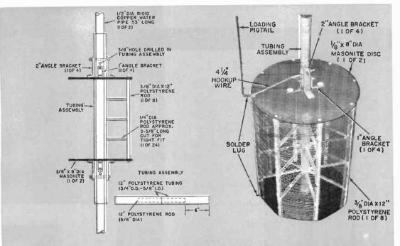
Fig. 5. Follow the details for the loading coil frame very carefully. Hack saws can be used to cut polystyrene rods. Use metal drills to make holes.
