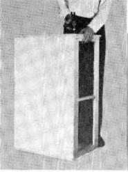
Building the Club Sandwich is much like building a house – construction begins with a wooden frame. Celotex is nailed on first, and layers of Sheetrock are then glued and nailed to the Celotex, as pictured below.
