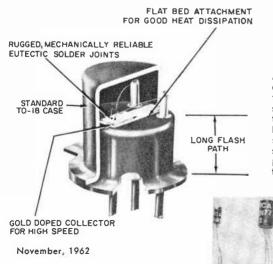
At left is cut-away view of post-alloy diffused type. Photo at right shows meltback diffused type with cover removed. Below (l. to r.) are subminiature, standard small-signal, medium power and high-power types of transistors.
