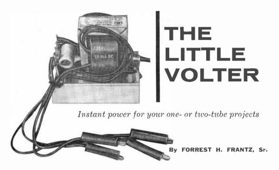
LTHOUGH experimenters are devoting more and more of their time to transistors these days, circuits always seem to come up which require the use of one or two tubes. And it's for just such circuits that this inexpensive little power supply was designed.
