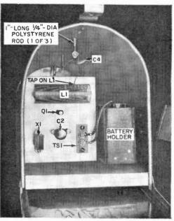
of the antenna pipes, forms a series-resonant cir-cuit which appears, electrically, as if it were a full-length quarter-wave vertical antenna. Chokes L3, L4, and capacitors C5, C6, C7 and C8 filter r.f. from the modulator line, thus stopping it from acting as a portion of the antenna system. Provided battery potential does not exceed 19.5 volts, the total resistance of R3 and R4
