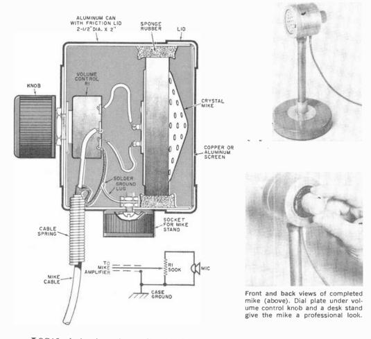
OCAL electronic parts suppliers stock many makes of low-cost crystal microphone replacement cartridges, and a cartridge with a frequency response of 30-7000 cps can be had for five dollars or less. With one of these cartridges and a little bit of effort, plus some spare parts and a microphone desk stand, you can come up with a useful microphone that has a built-in level control (see diagram) and is ideal for tape recording or p.a. announcing.
