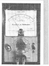
Make a few adjustments here and there, and hum level should drop markedly. A meter is a "must" for such work, due to comparative insensitivity of the ear. be done about minimizing much of the hum, however, and this "something" doesn't require a degree in electronics engineering. Nor do you have to get inside the cabinet with a soldering iron to rearrange the carefully planned, humminimizing design of the manufacturer. "Workshop" skills are enough: "workshop" skills—and the right meter!
