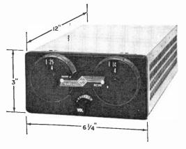
The transmitters and receivers used on private airplanes are almost incredibly small. This unit, a NARCO "Mark V," is crystal-controlled for 90 transmitting channels and 190 receiving channels!
