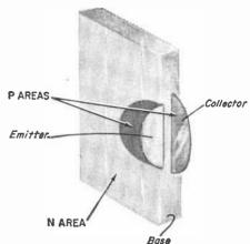
process which permits the formation of a very thin base region. Typically, a wafer of *n*-type semiconductor material is placed between two very fine streams of a metallic electrolytic solution. A d.c. potential is applied, causing the solution to etch away the semiconductor material.
