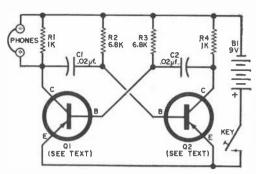
Fig. 3. Code practice oscillator built by reader Ron Raymer employs two pnp transistors in a standard multivibrator circuit. Layout is non-critical.
