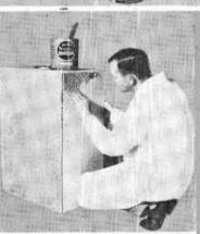
Some types of adhesive must be applied to both surfaces. Exact method of applying adhesive will vary with different brands, so be sure to read instructions on can and follow them carefully for best results.
