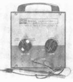
400-cycle tone into r.f., i.f., or audio stages. An output volume control is provided, as well as two 18" test leads. The "ground" test lead is terminated in an insulated alligator clip, the "hot" lead in a thin test probe for maneuvering freely in crowded circuitry. Power for the two transistors (a 2N363 and a 2N483) is supplied by an internal, 6-volt battery. Price, \$9.95. (GC Electronics, Inc., 400 S. Wyman St., Rockford, Ill.)
