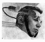
front of him. The apparent size of the image (up to eight feet in diameter) varies according to where he focuses his eyes. Many other applications are anticipated for the new device—it's being used by the pilot at left, for example, to receive pictured information from the control tower on air traffic and ground conditions.
