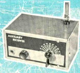
Auxiliary receiver tunes 122-144 mc., operates from any 12-volt car battery
