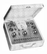
types can be accommodated. Instructions and tube charts are supplied in a ring-bound manual, and free supplementary tube listings are periodically made available. Housed in a Bakelite case, the Model 213 sells for \$18.90 in kit form, \$28.90 wired. The same unit in a wooden case (Model 213P) is priced at \$21.90 for the kit, \$32.25 wired. (Electronic Measurements Corp., 625 Broadway, New York 12, N. Y.)
