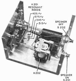
Parts placement for the relay unit is not critical, and there's plenty of mounting room. But be sure to insulate the frame of K201 from the box.
