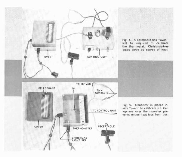
outlet, using the contacts of relay *K1* as a power switch. Finally, cut an opening in the cover of the box to view the thermometer, and paste a piece of cellophane over the opening to minimize heat loss.
