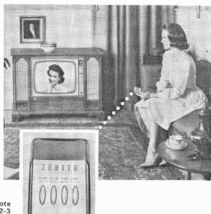
Fig. 1. Transistorized remote control is now simple as 1-2-3 on many new TV sets. Press a button on the "transmitter" (inset) and a transistorized "receiver" in the TV set does all the rest.
