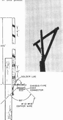
BAMBOO POLE WRAPPED WITH ALUMINUM FOIL
