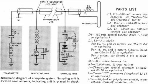
Schematic diagram of complete system. Sampling unit is located near antenna, indicating unit is placed in shack.
