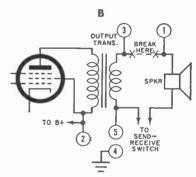
Sample schematics of wiring you may encounter in audio output stage of base transceiver. Type "A" requires only four wires to the relay circuit; "B" needs five.
