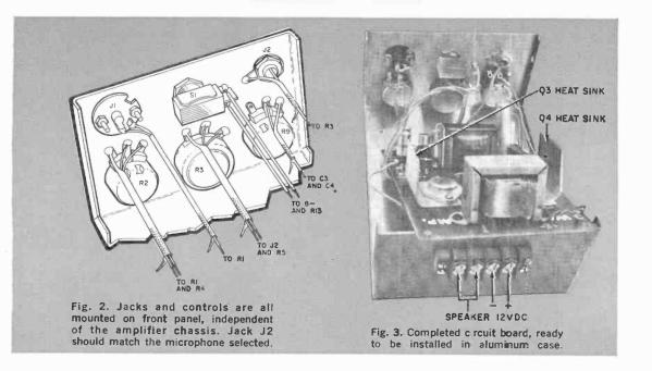
that the screws should again be about 1/2" long, since longer screws may short to the case. With this part of the wiring completed, set the circuit board aside for later installation in the metal case.
