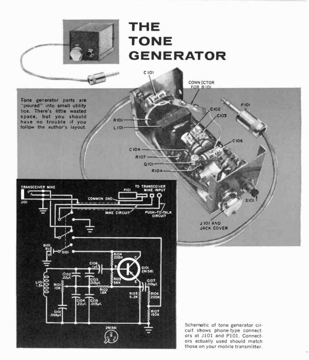
Building the Tone Generator. All of the tone generator components are fitted into a  $5'' \times 2\frac{1}{4}'' \times 2\frac{1}{4}''$  aluminum utility box as shown in the photo and pictorial diagram. Since paper capacitors are unstable when subjected to the temperature extremes encountered during mobile operation, don't attempt to substitute them
