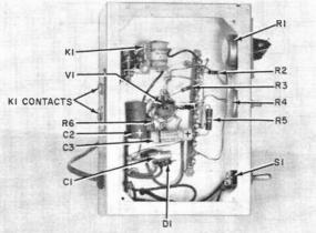
Fig. 2. Top view of thermostat. Transistor is connected to a barrier-type terminal strip.
