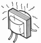
2 If a 50-cps transformer is operated at 60 cps, the transformer will overheat.
