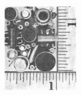
now being marketed by Otarion is said to be the world's tiniest. It measures 1" x 11/4" x 5/8" and weighs less than half an ounce. Containing 27 miniaturized components on a printed-circuit board, the receiver has a built-in tuning
