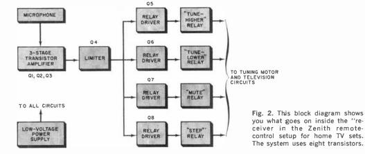
A four-position stepping relay, controlled by Q8, is used to turn the TV set "on" and "off," as well as to adjust the audio volume to one of three fixed levels. Special filters provide a proper time constant for relay control and prevent noise pulses from causing false operation. Different frequencies are used for each control function, of course.
