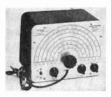
280 has usable harmonics to over 120 mc. Three types of output signal are provided: unmodulated r.f., modulated r.f., and 400-cycle a.f. A single output cable, in conjunction
