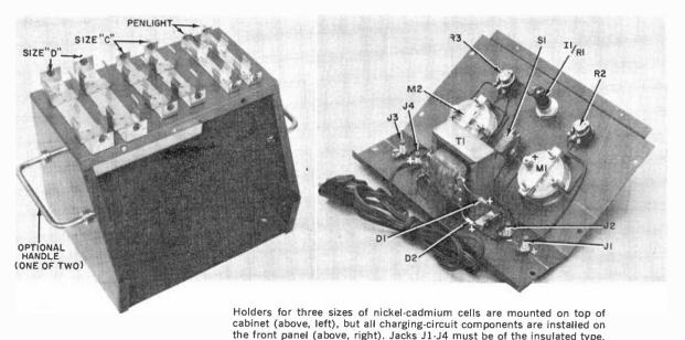
sloping-panel cabinet. All of the components in the charging circuit are mounted on the panel itself, and a series of holders for the batteries to be charged is installed on the cabinet top.
