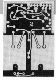
Fig. 1. You'll find construction a "snap" if you use the special printed-circuit board. Heat sinks for power transistors Q3 and Q4 can be cut out from an old aluminum chassis.
