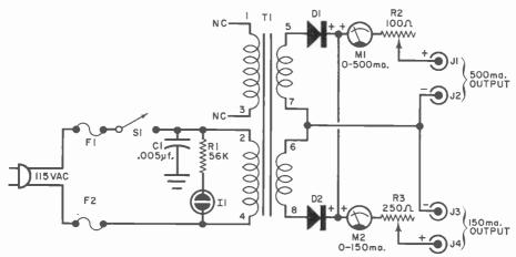
Schematic diagram of N-C charger. Two diodes are used as a full-wave rectifier, but TI's center tap, contrary to usual procedure, is not grounded.
