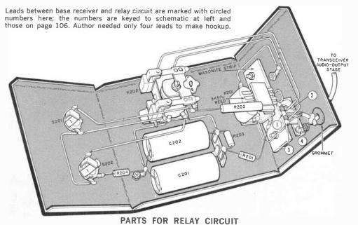
C201, C202—40-uf., 350-volt electrolytic capacitor
