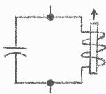
9 The tuning slug on an oscillator coil is most withdrawn at the top end of the band.
