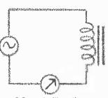
2 Current will continue to flow, even after the supply voltage has dropped to zero.
