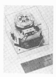
It worked—this time! The electronic timer built into Explorer VII failed to shut off the transmitter on 19.99 mc. in October, 1960. A similar timer installed in Explorer XI worked perfectly and switched the satellite to a new experimental program in late May. Explorer XI operates on 107.97 mc.
