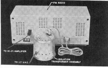
emphasis capacitor, as shown in the schematic diagram. Although the exact mounting details will vary from set to set, the jack can usually be placed at some convenient spot at the rear of the radio.
