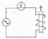
7 The lamp will glow more brightly as the iron core is moved out of the coil.
