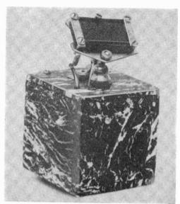
Framed photocell is mounted on optional ball-and-socket joint.
