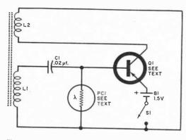
Fig. 4. Reader Kuhr's "light meter" transmits a tone that varies with the output of photocell PC1.
