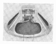
the hole to catch any metal chips—and be careful not to punch the paper cone with the drill. Many speakers already have transformer mounting holes which can simply be reamed out to the proper size. Make sure that all connections are tight and that the binding posts are properly insulated from the frame before trying out the speak--Art Trauffer
