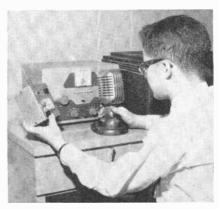
cuit is so designed that use of the monitor output does not disable the VU meter, and the unit is tunable from below 80 meters through 10 meters using "stock" coils.
