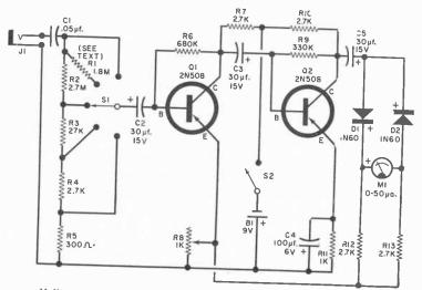
Voltmeter circuit incorporates a sensitive transistorized amplifier.
