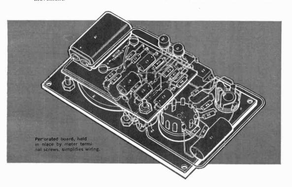
All of the other parts are mounted on the board by passing their leads through the perforations. Leads which are to be connected together are run through a common hole or joined with a length of wire running across the back of the board. Do the soldering from behind, using a small, well-tinned iron and rosincore solder. Heat should be applied for the shortest possible time to avoid damaging the components (the diodes and transistors are most sensitive).
