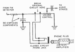
Schematic diagram shows how a closed-circuit phone jack can be added to your FM radio to permit it to function either as a tuner or as a receiver.
