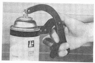
Handle-and-trigger removed from an old coffee maker enables you to hold and aim a spray can in "pistol-fashion."
