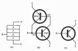
Fig. 2. Basic construction (A), equivalent circuit (B), and schematic symbol (C) of Tung-Sol's new "Dynaquad."
