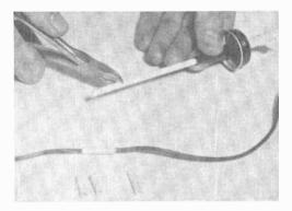
cutters to clip it into the lengths you need. You can also cut away the metal cap of the sprayer and remove the nozzle, leaving a handy plastic grommet for wire or cable feedthroughs.
