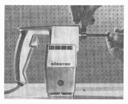
1800-rpm motor acts as a drill stand and may be firmly anchored to a workbench if desired. Chips and shavings are prevented from obscuring the hole being drilled by means of a controllable chip blower. Price, \$30.00. (Disston Division, H. K. Porter Co., Inc., Porter Bldg., Pittsburgh 19, Pa.)
