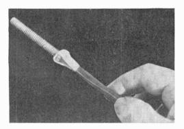
the size of the threaded part of the bolt or screw in a small strip of cellophane or masking tape, and pass the threads through the hole with the sticky side of the tape facing the head. Finally, draw the ends of the tape up and stick them to the blade; a twist of the screwdriver will pull the tape away after the threads have been started. You can use a similar technique for a nut, positioning it over the hole in the tape so that its threads are accessible.
