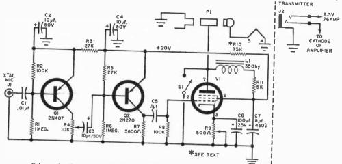
Schematic diagram of modulator. Modulate/test switch S1 is shown in "modulate" position; resistor R10 should be selected to produce about 20 volts at the emitter of Q2.
