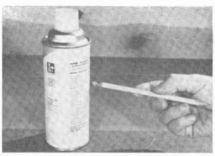
4 An accessory spray head (below) produces a "spatter-type" finish for old cabinets, enclosures, panels.
