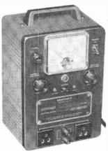
(300 watts continuous duty, 500 watts intermittent), improved meter accuracy (± 1 volt), and new styling. The IP-10 completely isolates equipment under test from the a.c. line. Output is variable from 90 to 130 volts in
