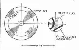
chassis punch, positioning the hole as shown in the diagram. To change speeds, turn off the motor and place the mechanism in the "rewind" position. Slowly rotate the supply hub to turn the drive pulley while using a hook bent from a stiff iron wire to guide the belt into the proper groove. During operation, the hole is covered by the supply reel and does not detract from the appearance of the machine.
