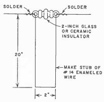
Fig. 4. Shorted stub on reflector loop serves to tune the element for maximum rejection of CB signals at the rear of the Quad antenna. Inspect soldered joints at insulator before installing antenna.
