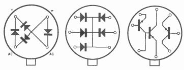
Fig. 1. Schematic diagrams of typical circuit packages produced by Fairchild Semiconductor Division. Four diodes at left are connected in bridge rectifier circuit, while five diodes in center have common cathode connection for use in logic circuits; three transistors at right (two in cascade) are intended for use in subminiature amplifiers. Diodes at left are assembled in a TO-18 package, other two circuits in TO-5 case.
