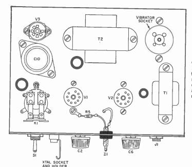
Drawing of top of chassis, with case removed. Neon bulb 11 serves as a tuning indicator and is held in place by a rubber grommet; R5 is soldered directly to one lead and attached to a solder lug under a screw at V1's socket.
