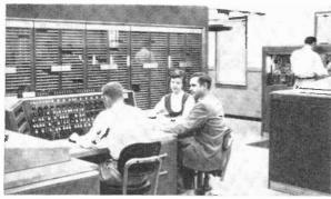
The U.S. Navy maintains a space surveillance system (NAVSPASUR) which has been in operation since 1959. It detects, tracks, identifies and determines the orbits of all non-transmitting space objects. Orbit computations are performed by the Naval Ordinance Research Calculator (NORC) at Dahlgren, Va.
