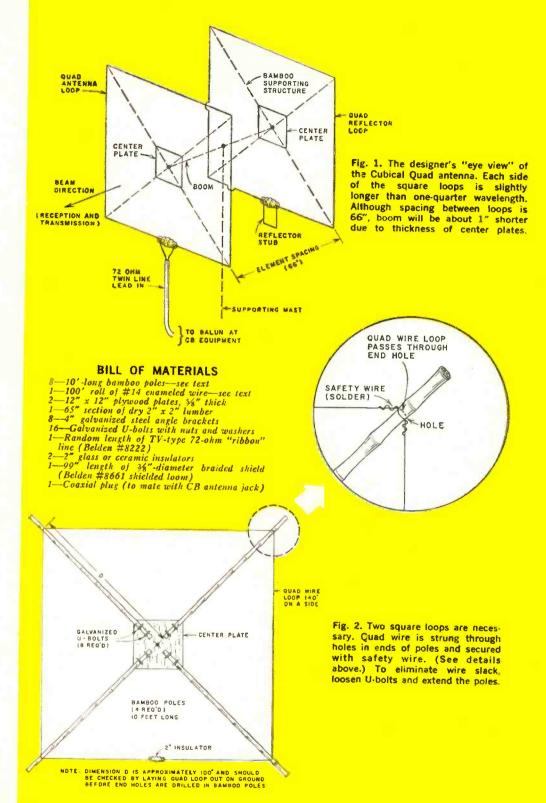
best picks up r.f. signals—is in a plane at right angles to the plane of the loops and *through* the driven element.
