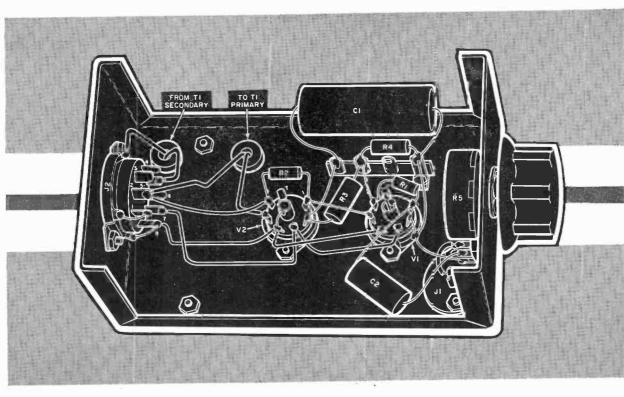
lifier. Almost any of the common tubes can be used if slight changes in circuit values are made; some tubes, of course, will give more gain than others. Two very common types are used here—the 6AU6 pentode (V1) and the 6AQ5 beam power audio tube (V2).
