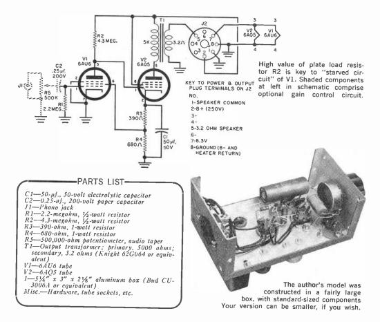
looking at the data sheets for a 6AU6 pentode. This tube gives a gain of about 300 with a 250-volt plate supply; and if the voltage is reduced to 100, the gain may fall as low as 110. If the screen and plate voltages are reduced to about 15 volts, however, the gain may go up to well over 2000 under the right circuit conditions.
