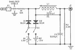
Placement of parts and wiring details for the "Ear Saver" are shown above. Capacitor C2 can be increased to 0.1  $\mu$ f. to reduce high-frequency background noise on c.w. signals. Experiment with the value of resistor R2; with some headphones, this value should be changed, or the resistor eliminated.
