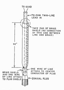
Fig. 6. Neatness counts when wiring up the simple balun. Poor solder joints and incorrect lengths will lessen power gain of the Cubical Quad. So do it right!
