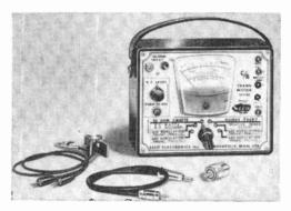
to 5 watts r.f. and has a 0-400-ma. scale. You can check to see how much power you are losing in your transmission line—read the meter and weep!
