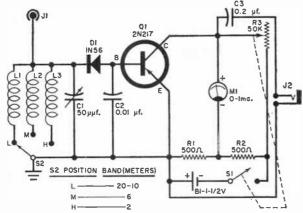
Capacitor C3 isolates headphone circuit from d.c., as shown in schematic diagram, so that high-fidelity crystal headset can be used. Battery B1 could be an ordinary 1½-volt penlight cell, but the mercury battery specified in the parts list has a lower internal resistance, longer life.
