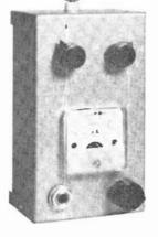
The FSM has headphone output jack for use in checking transmitter's audio quality. Plugging in headphones does not change sensitivity of instrument.
