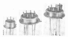
ample, is a cylindrical enclosure approximately \( \frac{1}{4}'' \) high by a little over \( \frac{1}{3}'' \) in diameter. A "TO-18" case, also cylindrical, has about the same height as its diameter, measuring close to 1/5" in each dimension.
