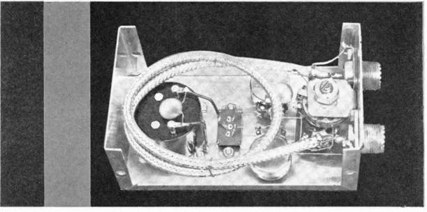
Parts layout of power meter is highly symmetrical and reflects arrangement of schematic diagram on page 64 very closely. See text for details of pickup loop.
