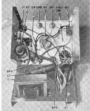
View of aluminum box with chassis removed. Operating controls are mounted on top of box, with fube V1, transformer T1, and most small components on chassis.
