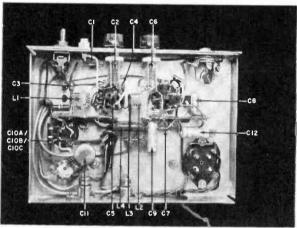
The three cables coming from relay K1 are shielded; ordinary phono cable will serve very nicely. Note that in each case the shield grounds at only one end of the cable (at the underside of the chassis).
