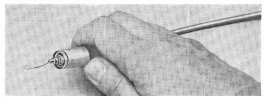
YOU CAN INCREASE the utility of your vacuum-tube voltmeter considerably by building an r.f. probe for it. Although a standard VTVM has an input capacitance which limits its a.c. measurements to frequencies below about 50 kc., an r.f. probe will push this frequency range well into the shortwave region. In fact, the probe described here can boost your VTVM's upper frequency limit into the 6-meter band—a frequency jump of over 1000 times!
