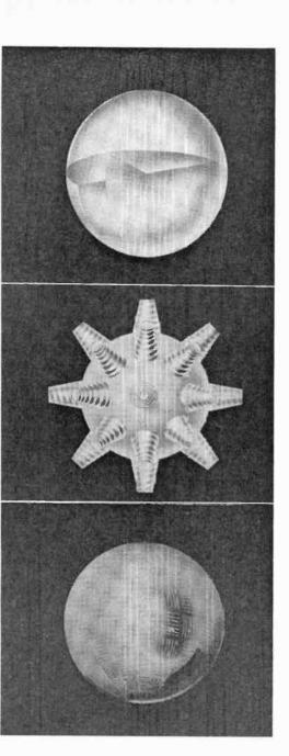
Suggested designs for passive or Echo-type satellites worked up by Ryan Aeronautical Company. At the top is a corner reflector fitted into a sphere. In the center, 26 cones have been formed into helical antennas. At bottom, dipole strips have been attached to the balloon—they are at right angles to one another to counteract polarization changes as the satellite spins and wobbles in orbit.
