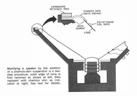
aside, since you will want to glue it back in place later. Now, using a razor blade or small scissors, cut the cone rim, except for the four tabs, as shown on page 68.
