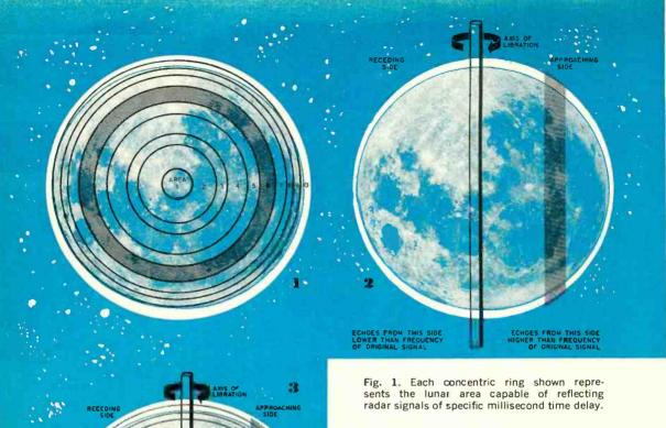
Fig. 2. As the moon rotates, it also librates, so that radar echoes vary above or below their radiated microwave frequency. Shaded section at right represents a certain frequency band which is located above radiated frequency.
