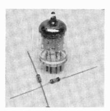
Two low-cost diodes replace 6AL5 vacuum tube, saving filament power and space.
