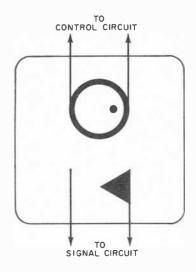
Fig. 2. Schematic symbol for the Raysistor. Note that there isn't any electrical connection between the control and signal circuits.
