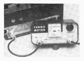
Globe output meter serves as monitor and modulation check. It is left in transmission line at all times.
