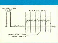
Lunar radar echoes are long in duration since the same narrow pulse must be reflected from a spherical surface. The echo can be easily divided up into segments to match those in Fig. 1.
