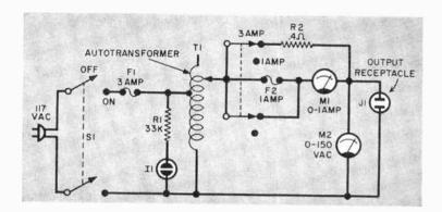
Schematic for the EICO Model 1073. Meter range switch automatically cuts out fuse F2 when 3-ampere scale is being used. Fuse F1 then protects meter as well as autotransformer
