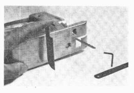
tute from a standard hacksaw blade. Break off a piece of the hacksaw blade and grind it down to fit into the power saw chuck. The blade's tip should also be rounded off to make cutting starts easier.
