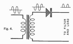
most efficient. Half of the a.c. power is not used. However, by connecting three additional diodes into a "bridge" circuit, the half-cycles of opposite-polarity a.c. can be steered in the proper directions so that both halves of each cycle are used and yet the power supplied to the filter is direct current. Refer to Fig. 5.
