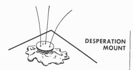
Need some way to shock-mount a lead-type transistor? Simply build a little pool of Duro plastic rubber and stick the transistor—wire leads up—in it. When the latex dries, the transistor will be shock-mounted and the leads readily accessible.
