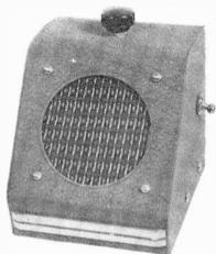
Audio tone source submitted by reader Eugene Richardson is housed in meter case. Control on top adjusts frequency.
