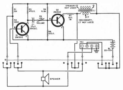
Two-stage transistorized amplifier above is heart of each of the three-way intercom units. External cable connections are made to terminal strip TS1.
