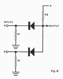
choosy—it will produce an output signal only if you give it signals at both of its inputs. If you give it a signal at only one of the input terminals, it produces nothing. This is called a logical "and" circuit, since it must have both signal A and signal B to provide an output. Another way of putting it is to say that the circuit must decide whether both inputs are present before deciding to produce an output.
