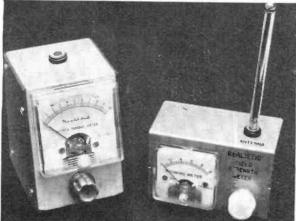
Heathkit and Radio Shack field strength meters have magnets in underside of case to hold meter to automobile steel dashboards.
