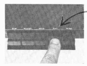
Push buttons on Telectro 900-4 provide for simple operation
