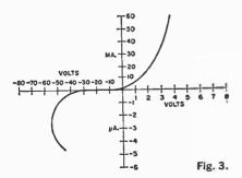
The vertical scale in Fig. 3 shows current; the horizontal scale, voltage. Note that forward voltages and currents are
