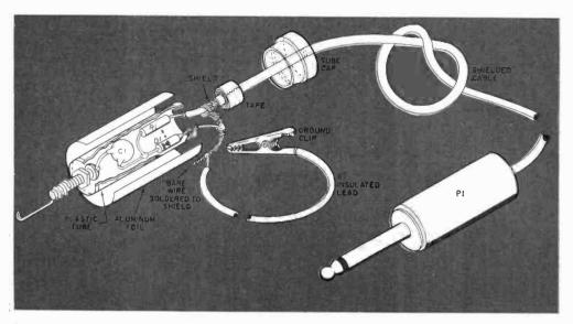
Fig. 2. Pictorial diagram shows how author's probe was assembled. Hook added to probe screw simplifies trouble-shooting.
