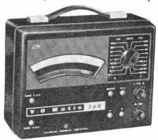
cise readings, and the meter is protected against extreme overload. Sensitivity is 20,000 ohms per volt d.c., 5000 ohms per volt a.c. The unit covers a.c. and d.c. volts, d.c. current, a.f. (output), and resistance in 25 ranges; 18 separate overlay meter scales are provided for supplementary ranges. Price, \$59.95; an optional leather carrying case sells for \$11.95.
