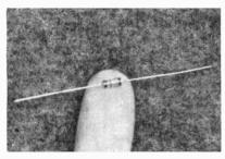
Small semiconductor diodes have axial leads, eliminating the need for sockets.
