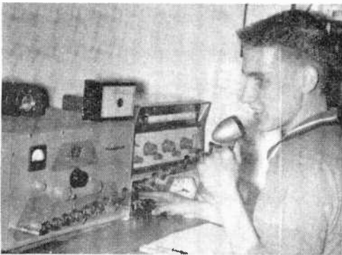
Jack Ray, K4MZW, uses his Heathkit DX-100 and Gonset G-43 for both phone and c.w. operation.
