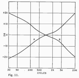
correct this situation by attenuating the treble and boosting the bass. If this circuit were perfect, its characteristic curve would be the exact opposite of curve A in Fig. 11 and would look like curve B.
