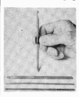
ment tools. Use the hooked end of a needle to manipulate dial cords in tight corners; file the other end to fit tuning slugs and screws on i.f. transformers. A small "knob" can be formed in
