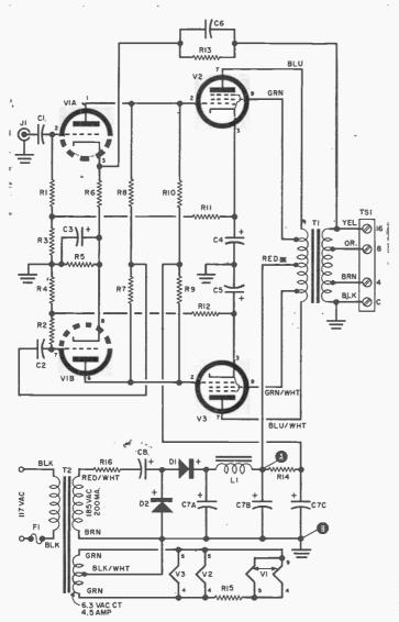
In normal operation, voltage from point A to point B is 390 volts d.c. Heater current to tube V1 is "starved" by use of dropping resistor R15.
