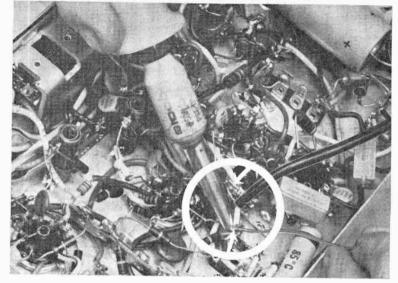
Hot lead of Q-Multiplier's output cable can be connected to plate of first i.f. tube at i.f. transformer (lower arrow in photo). Cable's shield should be soldered to ground lug nearby (upper arrow).
