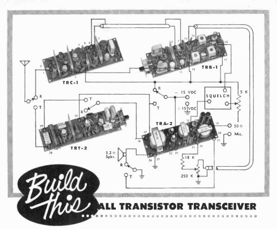
Now you can build your own All Transistor, Crystal Controlled, Portable Transceiver for Citizens band or Amateur communications. International subassemblies, prewired and tested are "quickly" interwired and ready for operation. Fifteen transistors for transmitting and receiving. Dual conversion superheterodyne receiver. Noise limiter and squelch. International precision crystals and highest quality components throughout. Power requirements: 15 volts dc @ 60 ma average. Positive ground.
