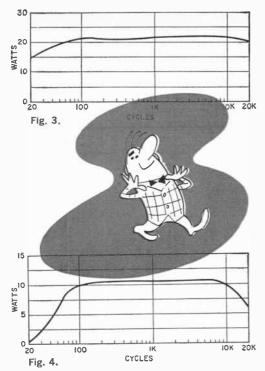
20 watts at 50 cycles, and, at 20,000 cycles, the curve has just barely begun to dip.
