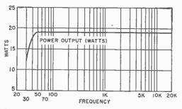
Power response of amplifier is shown above for a Harmonic distortion of 2%. Note that due to use of a special output transformer the output is flat from 48 to 20,000 cycles. Harmonic distortion at 18 watts output at 30 cycles is less than 3%.
