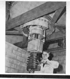
Mammoth electron beam generator (left), produced by General Electric, delivers some 3.5 million electron volts. Electrons emerge from thin titanium window at bottom of anode (funnel-shaped structure with cooling fins, above).
