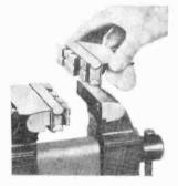
of adjustable jaws available from Mid-American Import Co., Inc., 1919 Champa St., Denver 2. Colo. Steel fingers in each jaw adjust to hold any shaped object firmly. The "Uni-Grips,"
