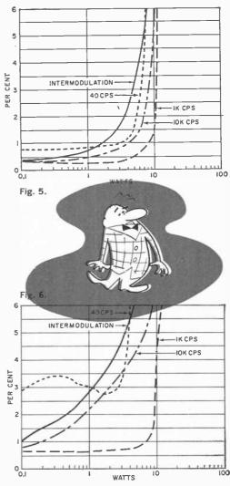
6% at 8 watts. Harmonic distortion at 1000 cycles remains low—below 1%—almost to 10 watts. But the figures at 40 and 10,000 cycles again tell a different story.
