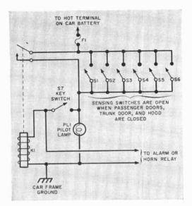
The alarm operates and relay K1 locks up when both key-operated switch S7 and any sensing switch (S1 to S6) are closed. Sketch at right, above, shows suggested spots for placing sensing switches.
