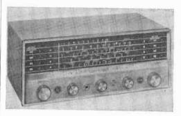
front-panel-controlled BFO; and provisions for up to three antennas. Essentially an improved version of the older S-38E, the S-120 comes with a built-in loopstick antenna for the standard broadcast band and a collapsible whip antenna for short-wave reception. Employing a sensitive, four-tube superhet circuit with a selenium rectifier, the S-120 also has its own built-in speaker. Price, \$69.95. (Hallicrafters, 4401 W. Fifth Ave., Chicago 24, Ill.)
