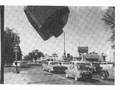
Traffic detector—the "Traffitrol"—uses infrared beam to detect and count vehicles traveling at speeds up to 80 miles per hour. Highly accurate and virtually foolproof, the device is among the first to apply infrared principles to traffic problems. The "Traffitrol" is manufactured by the Heiland Division of Minneapolis-Honeywell.
