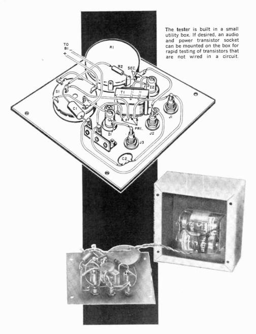
maximum resistance position, the "bad" lamp shouldn't light; if it does, the transistor has excessive leakage. If both lamps light when R1 is at a maximum, it indicates that the transistor is operative but may not work in critical circuits.
