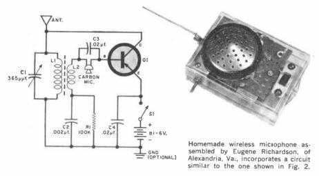
Fig. 2. Wireless microphone circuit submitted by Edward Morris has hand-wound oscillator coil (L1-L2). FCC regulations limit antenna length to 10 feet.
