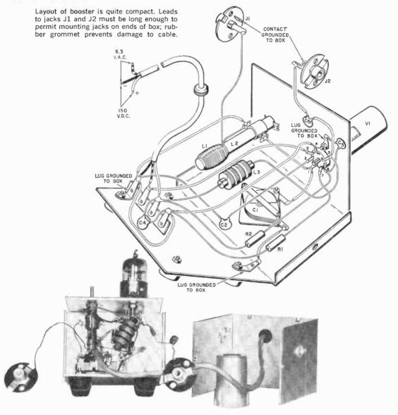
ungrounded 6.3-volt a.c. heater lead. With power applied, the booster is ready for operation. Connect a dipole antenna to jack J1 and connect the receiver's antenna terminals to jack J2. For operation with a long-wire antenna, connect only the center (hot) terminal of J1 to the antenna with a good ground connected to J1's ground.
