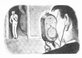
phones' were developed by the Infrared Industries of Waltham, Massachusetts. They permit talking over distances of several hundred feet by means of beams of infrared radiation.
