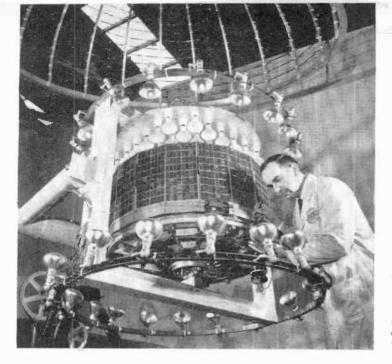
Magnetic orientation system being tested at RCA's Space Center in Princeton, N. J. Lights above and around the satellite are L sed to check operation of solar cells which surround satellite.
