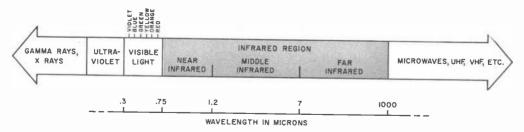
Infrared band, sandwiched between visible light and microwave regions, comprises wavelengths from 0.75 to approximately 1000 microns.
