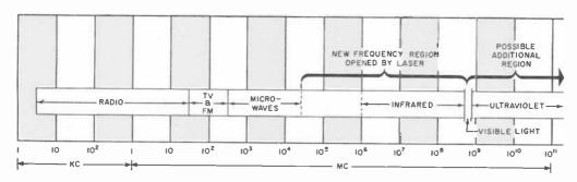
Frequency spectrum, showing new frequency region opened by laser. Note laser's wide operating range.
