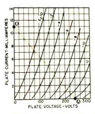
"Good, but remember this, Larry. The load line you just drew is only good for a 6J5 with a load resistor of 22,000 ohms and a plate supply voltage of 240 volts. There's (Continued on page 128)
