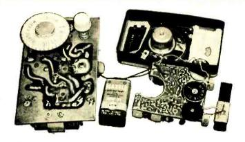
Etching techniques were identical for printed-circuit radios shown here, although model at left is a home-brew unit.
