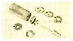
drilling a ¼" pilot hole, inserting the pilot rod on the punch, selecting and assembling die and punch, and hammering it through the chassis. The punch costs \$4.98 and is available from "Punches," P. O. Box 415, Toledo 1, Ohio.
