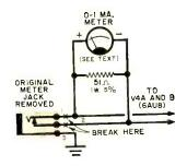
Meter jack leads are disconnected and rewired to plate current meter; jack need not be removed from set.
