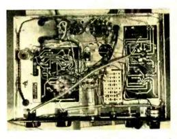
**Underchassis** wiring is simple; the majority of connections are already on printed-circuit boards.
