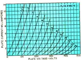
and plate voltages. You can see that we don't take an output from the tube, either. This is the setup used to work out what are called the static characteristic curves for the tube."
