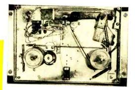
**Top view** of tape deck with cover removed. Drive belt must be moved from larger to smaller diameter pulley to change tape speed from 7½ to 3¾ ips.
