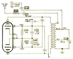
**Push-pull** bias-erase oscillator employs a single 12AU7 tube in a special low-distortion circuit.
