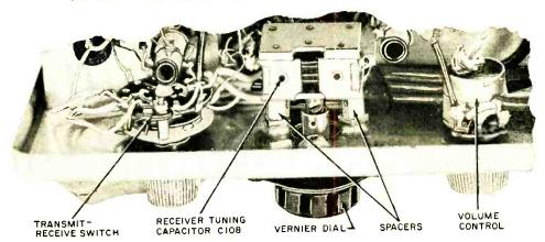
Tuning capacitor C108, above, is remounted to front panel with spacers; shaft is modified to fit vernier dial.
