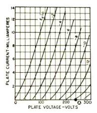
"Good enough, Larry. You have one of the points for the load line we're drawing. I should mention that a resistive load line is linear, which simply means that it's a straight line and not curved. So, if we can find one other point and mark it on the chart, we can connect the two points and have a load line. Do you follow me?"
