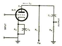
"This looks more like the real thing, Ken. It's an amplifier and it has a resistor in the plate circuit, and . . ."
