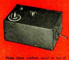
Photo timer controls mount on top of cabinet; R3 has timing scale (white circle).
