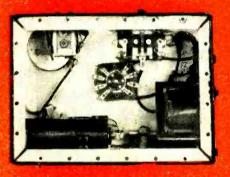
With bottom cover of relais can be seen on upper apron; line switch is in center.
