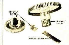
around the broken portion and solder the ends of the strip together. Use a minimum of heat when soldering to prevent damage to the knob. Flat strips of brass can be obtained from automobile parts dealers who sell this material for shimming purposes. -H. L. Davidson, Fort Dodge, Ia.
