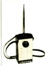
Harbor, Mich., in both kit and factory - wired form. The unit has a batteryoperated, fourtransistor circuit, and features a fixedtuned superregenerative receiver. According to the manufacturer, the crystalcontrolled transmitter can
