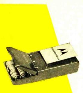
Radio paging receiver is carried by each individual in a remote paging system. This completely transistorized superheterodyne unit, made by Motorola, delivers 1/2-watt output to built-in speaker.
