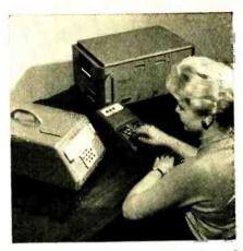
Three-part psychomotor skill trainer of Rheem Manufacturing Company includes: (1) a program display unit; (2) a standard IBM keyboard; (3) a computer control unit.
