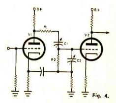
see, it is very similar to the frequencydetermining network in the EICO 377 signal generator. Tube V1 is a phase splitter. It takes the incoming signal, slices it into two parts 180° out of phase, and applies both parts to the grid of V2. But one part is applied to the grid through series network R1-C1, the other through parallel network R2-C2.
