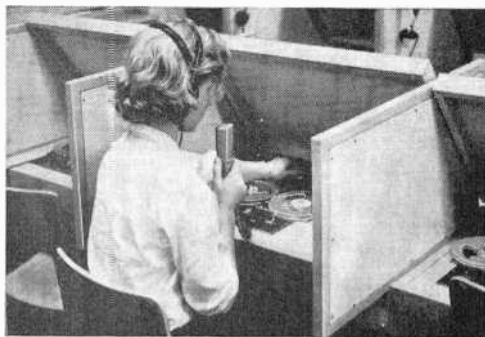
Student's booth contains a tape recorder, a microphone, and a set of headphones. The student listens to a prerecorded lesson and repeats it phrase by phrase into his tape recorder. In playback, he hears the two tracks one after the other and is able to compare his pronunciation with that of the instructor.
