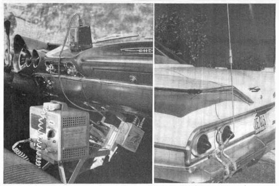
Rack holds transceiver (above left) at convenient distance from driver; note antenna change-over switch and field strength meter on top of dash. Antenna bumper mount (right) is easy to install.
