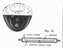
and weight are important—in airborne equipment, for example. Another important advantage of the new movement is its ability to handle overloads that would instantly burn out the relatively delicate Weston movement. The manufacturer claims that an overload of 1000 to 5000% will not damage these movements.
