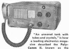
"Workhorse of Industry." **Poly-Comm** II, is most rugged and reliable citizens band transceiver made. Designed for continuous duty and featuring a super-sensitive dual conversion superhet receiver . . . optimum selectivity through dual conversion with 16 tuned circuits and three 455 Kc IF stages (If you hear him he's on your channel) . . . completely weather and rust proofed . . . tefton wiring . . . solid steel cabinet and chassis for rugged use under any conditions.
