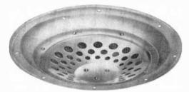
signed to mount in any ceiling, wall, or other baffle, the SK-175 features an unusual construction that places its 12-oz. magnet in front of the cone rather than behind as in conventional speakers. The voice coil is 1" in diameter; frequency response is from 90 to 9000 cps; impedance, 8 ohms. Outside diameter is  $9\frac{1}{2}$ ", including the integrated metal baffle; a  $6\frac{5}{2}$ " wall cutout is required. Price, \$5.95.
