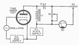
Fig. 2. Dynamic-conductance testing circuit in Heath Model TT-1 tester. Circuit approximates actual operating conditions, and tube is subjected to working test. Meter MI measures output voltage.
