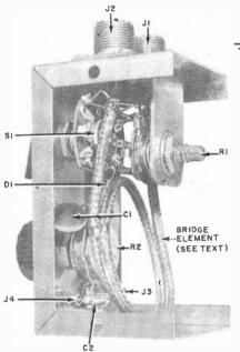
a 75-ohm, 500-watt element, use RG-59/U cable. If you want a 1-kilowatt element, substitute a 10" length of RG-8/U for a 52-ohm system or RG-11/U for a 75-ohm system.
