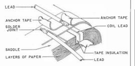
Fig. 5. Method of tapping secondaries in Acrosound transformer for identical leakage reactances.
