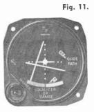
connected to the electronic receivers in an aircraft instrument landing system and arranged so that they show the pilot whether he is on or off course (Fig. 11). Such meter applications are virtually endless.
