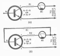
Transistor-testing circuits Fig. 4. in EICO Model 666 tester. Circuit (A) measures emitter-to-collector leakage; circuit (B) measures beta.
