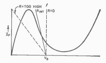
Fig. 4. Load line for typical tunneldiode oscillator. Load must be as low as possible to restrict diode to negative-resistance portion of curve.
