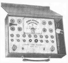
"Quick" tester manufactured by Superior Instrument Co. has several sockets with pin connections permanently wired to reduce pre-test adjustments.
