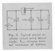
point, the diode reverts back to type and the current increases as the voltage is increased above Vv. By operating the tunnel diode on the negative-resistance portion of its curve, we can make it function as a negative-resistance oscillator, as will the tetrode above.
