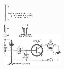
Schematic diagram of field strength meter. Exact values of CI and MI will depend on desired range and sensitivity of unit; switch SI can be omitted if antenna is unplugged whenever meter is not in use.
