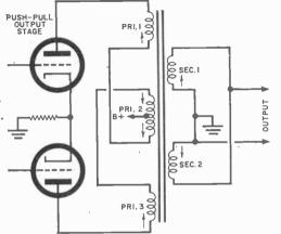
Fig. 4. Circuitry of Dyna hi-fi output transformer. Interleaved and counterbalanced windings help reduce leakage. fiers at a reasonable cost we needed better output transformers. Because of the lack of suitable commercial transformers, Williamson advised constructors to build their own. But manufacturers soon took steps to correct this situation.
