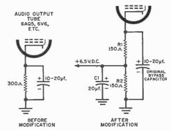
and R2 serve as a voltage divider, and capacitor C1 insures that no audio variations will appear in the output voltage. Any cathode-biased output tube can be used, but the output voltage will of course depend on the tube's bias and the ratio between R1 and R2.—James Romelfanger, Baraboo, Wis.
