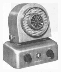
A simple device for producing and controlling negative ions in a closed room, the Wesix lonaire consists of a rectifier and a piece of radioactive tritium foil mounted within a conducting tube.
