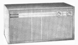
An air-purifying device, the Granco lonator effectively combines mechanical filtering, electrostatic precipitation, and negative ionization actions.
