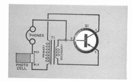
Fig. 1. This audio oscillator, submitted by reader Steven Brattman, works as long as the sun shines. It's a good code-practice unit for out-of-door use.
