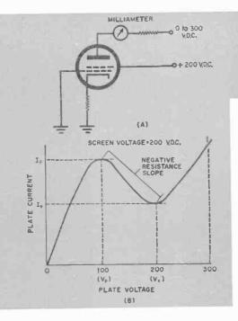
When the plate voltage reaches the value of the screen voltage, 200 volts in this example, the plate current increases as before.
