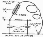
lead of the resistor to the other end of the wire. Then connect the remaining resistor lead to the probe tip. When you have turned off the equipment, fasten the alligator clip to the unit's chassis or ground bus. Then discharge all filter capacitors by touching the probe to their positive terminals for a few seconds—*Clifford Marshall*, *Edmonton, Canada*.
