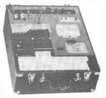
**Revolutionary tester** by Hickok Co. applies modern computer principles to tube testing. Punched card corresponds to particular tube under test.
