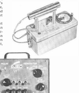
Test instruments are becoming more and more transistorized. Cubic Corporation's pulse generator and Universal Transistor Products' Geiger counter (top photo) are examples of this trend.
