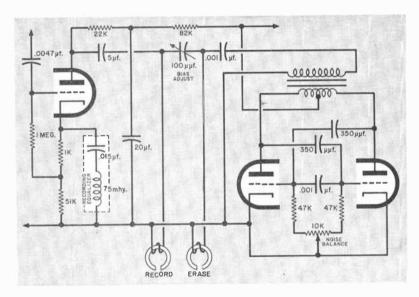
Fig. 1. Recording circuit of the Ampex 910. The 10,-000-ohm potentiometer allows the push-pull oscillator to be balanced for minimum harmonics. Erase current is supplied through the  $.001-\mu f$ . capacitor, and bias for the record head can be adjusted by the 100-µµf. capacitor. Network in cathode circuit of driver tube boosts high frequencies in recording process.
