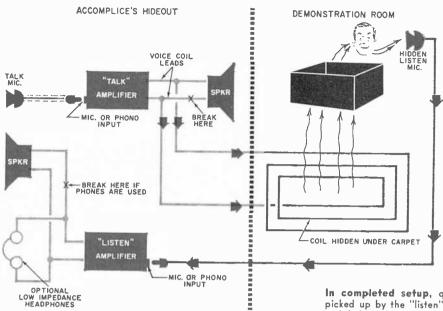
In completed setup, questions are picked up by the "listen" microphone and fed to the accomplice's hideout. The "talk" amplifier sends his answers back to the demonstration room where hidden coils transfer them electrically to the amplifier in the black box.
