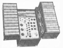
test leads, etc.; and tests over 700 tube types. Its 21 sockets are made of phosphor bronze, its panel of etched aluminum. Price, \$74.50.
