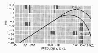
Fig. 2. Unequalized recording curves for a high-quality head.
