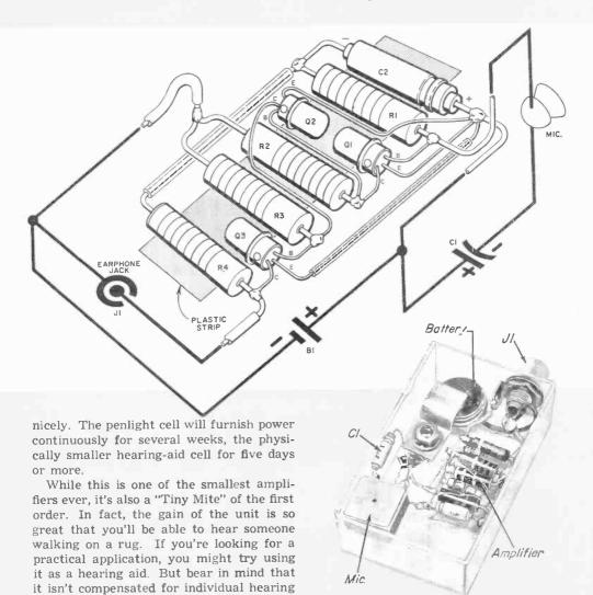
Amplifier, microphone, battery, and earphone jack are mounted in a plastic hardware box. Miniaturization can be carried still further through the use of ultraminiature resistors.
