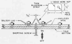
Transistor amplifier for black box is built on disc cut from plastic or Masonite sheet and attached to larger sheet. (See pictorial above and exploded view at right.) "Screwswitch" SI (detail above) is optional; batteries can be wired permanently into circuit.
