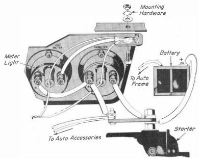
Illuminated meters show battery chargedischarge current and voltage at a glance.
