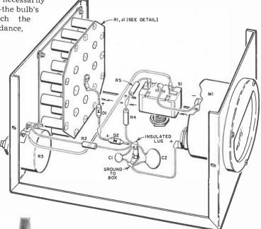
Standard Minibox serves as chassis for power meter. For best results, use a single insulated tie-point and ground lug when wiring, as shown in pictorial diagram.
