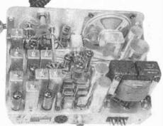
usual click from the press-to-talk switch. A newly developed circuit (patent-appliedfor) makes switching in the Poly-Comm entirely electronic. A portion of the transmitted signal is applied to the receiver's first r.f. stage, which acts as a diode, creating a bias that causes the a.g.c. line to cut off the receiver.
