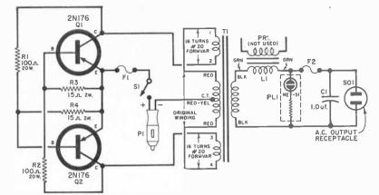
Check the polarity at car's cigarettelighter socket before wiring plug. Choke LI is secondary of 117-volt filament transformer.
