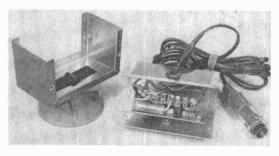
aluminum Minibox. The chassis can be made from a discarded cookie sheet: simply cut out a small piece using a pair of tin snips or a hacksaw, then bend it to shape in a vise.
