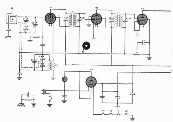
signals needed to align receivers quickly and efficiently. But alignment is complicated in practice because manufacturers supply a wide variety of alignment controls in various receivers. The instructions that follow will serve as a general guide for aligning any receiver, but some adaptation will be needed to cover variations in individual radios. (If you have the manufacturer's alignment instructions, you can follow them with good results.)
