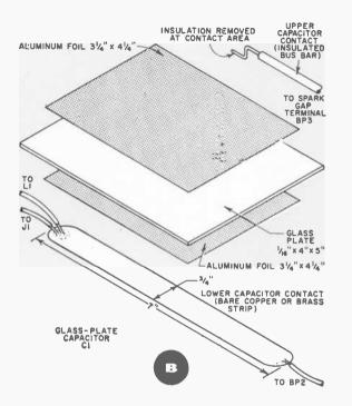
Wiring the unit is simple once components are assembled on 8½" x 12" breadboard (see pictorial, opposite page). Detail "A" (below the pictorial) gives data on the Tesla transformer primary and secondary windings L1 and L2. Detail "B" (left) shows how to construct glass-plate capacitor C1. Wiring is pointto-point, using No. 14 insulated hookup wire.
