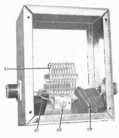
Simple filters suppress harmonics on the 80- and 40-meter bands. Chassis for 80-meter unit is large enough to hold the 40-meter filter as well.
