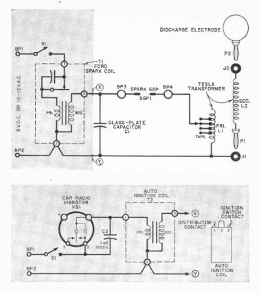
Spark coil TI can be replaced with vibrator and ignition coil combination if desired. Parts required for vibrator supply appear as optional items in parts list; use alternate shaded schematic at lower left.
