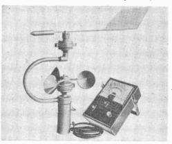
maica 33, N. Y. The transmitter assembly can be mounted on any 1¼" pipe or mast. The indicator is housed in a wooden cabinet and provides two wind-speed scales-0-25 mph and 0-100 mph—and a third scale for direction. Speed accuracy of  $\pm 5\%$  is claimed. Price, complete with 60' cable and a 1½-volt battery, \$59.95.
