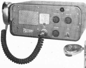
ond oscillator-mixer; a 6BJ6 first i.f. amplifier; two 6BH6's as second and third i.f. amplifiers; a 6AL5 detector/automatic noise limiter/automatic gain control; a 12AX7 first audio-squelch; and a 6AQ5 audio output. The i.f. frequencies are 6.0 mc. and 455 kc.; 16 tuned circuits appear between antenna and detector.
