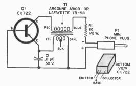
Various transistors and transformers can be substituted in the GDM modulator circuit. Changing the value of the capacitor will vary frequency of oscillation.
