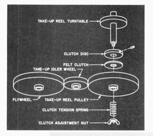
Fig. 3. Slipping-clutch drive system. The amount of slipping is determined by tightening or loosening the clutch adjustment nut.
