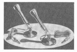
pairs from Sonotone Corporation, Elmsford, N. Y. The "CM-T10" set features response flat from 50 to 13,000 cps at an output level of -62 db. The "CM-T11" set's frequency response is from 50 to 8000 cps with the sensitivity 55 db below 1.0 volt per microbar. Rubber-encased ceramic elements serve as transducers for all the microphones. Price, \$36.75 per pair. Table stands are available at \$5.00 each.
