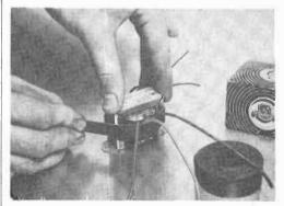
strip of tape around the transformer as shown. This will also help prevent the leads from breaking off or coming loose.—John A. Comstock, Wellsboro, Pa. —<u>30</u>—
