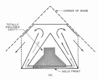
Fig. 2. Horn systems are both the most efficient and the bulkiest type of emclosures. The front-loaded horn (A) uses only the front radiation from the speaker. The backloaded horn (B) radiates the front wave directly and horn-loads the back wave.
