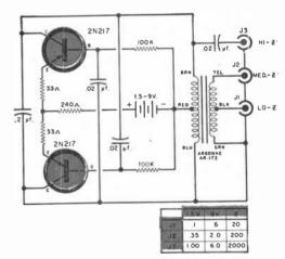
or value. Only the 240-ohm resistor may need adjustment; if it is too low for the transistors the waveform may suffer somewhat, and if it is too high the output will fall off. Frequency of operation can be lowered if desired by adding capacitance across the .2-µf. capacitor.
