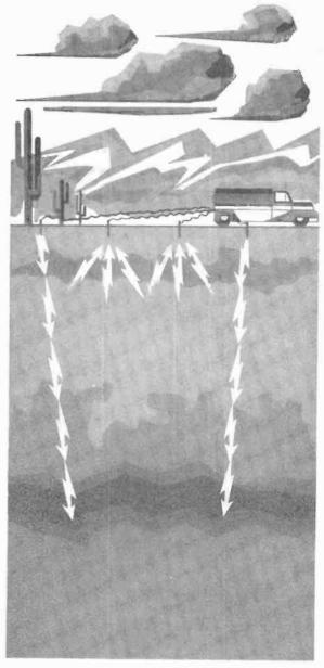
Underground water is located by pulsing current into the ground and then measuring the decay rate of the pulse. The two outside electrodes "fire" the initial current into the ground for a period of about three seconds. The induced polarization decay potential is then picked up by the two inner electrodes and is fed into an integrator-recorder system. By measuring the rate of decay, scientists can determine if water is present, its chemical content, and how far down it is.
