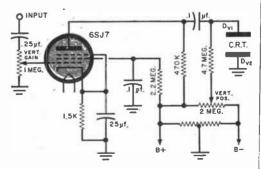
Fig. 1. Typical single-ended amplifier used in early scopes. Circuit has limited frequency response and low sensitivity.
