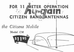
Chrome plated and stainless steel telescoping whip extends to 73" and down to only 23" for easy garaging. Weatherproof, polyethylene enclosed, high efficiency base loading coil includes exclusive Hy-Gain "L" matching network for perfect 50 ohm match. "L" matching network for perfect 50 ohm match. Complete with universal swivel body mount, only one hole to drill for easy mounting.
