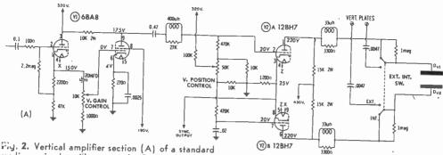
Fig. 2. Vertical amplifier section (A) of a standard medium-priced oscilloscope—the Paco S-50. Note direct-coupled output stage; more expensive models are direct-coupled throughout. A frequency-compensated attenuator switch (B) is used at the input of this amplifier; it has three attenuation positions—maximum attenuation occurs at the X100 position.
