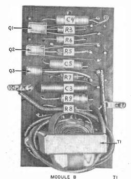
plied. This unit is complete within itself and can be tested without connection to the other circuits. The frequency of the transistor oscillator (Q1 and Q2) can be changed by variation of R4 and C4. The values given for C1 and R1 cause a pulse rate of about 100 per minute in the neon lamp relaxation oscillator.
