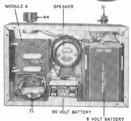
Rear view of cabinet with back panel removed shows relative placement of major components. Use a larger cabinet if you find wiring or assembly too crowded.
