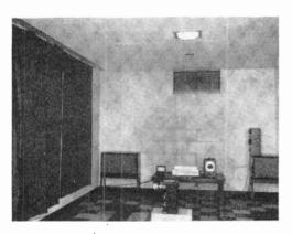
Observations: This test was undertaken to evaluate the possible effects of applying acoustical tile on the walls. Although no improvement was made without the carpet in place, the stereo range was extended to 12 feet with the carpet. At 15 feet from the speaker, the attenuation of the direct sound from the speaker was actually more than that of the reflected sound from the right wall and caused the peculiar reverse effect indicated by the measurements made at this distance.
