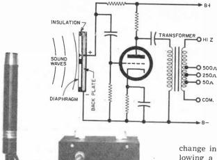
Fig. 2. A capacitor microphone requires a separate power supply. Sound waves impinging on the microphone diaphragm cause variation in the charge on the plates at an audio rate, and this potential variation is fed to the input grid of a triode. The unit shown above is a Capps CM2001.
