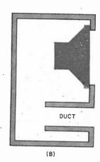
Fig. 1. Bass-reflex enclosure (A) uses the speaker's back wave to augment its direct radiation. Ducted-portenclosure (B) works on the same principle and can be physically smaller than a bass-reflex enclosure which has the same resonance.
