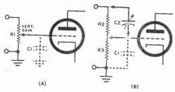
Fig. 3. Uncompensated gain control (A) has high-frequency roll-off due to the action of "stray" capacitance C1. Installation of another capacitor enables enough boost to be added to the circuit (B) to provide the exact frequency compensation needed.
