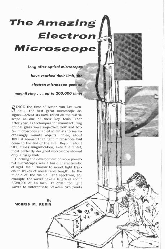
of an object, they must be separated by about one-third the length of a light wave, or about 2/250,000 of an inch. Objects smaller than about half a wavelength cannot be magnified clearly by a light microscope, no matter how perfect its lenses.
