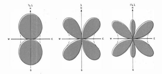
develop on the highest frequency band. Some typical half-wave (λ/2) antenna lengths for use on the short-wave bands are: 62.4 feet at 7.5 mc., 52 feet at 9 mc., 42.5 feet at 11 mc., 31.2 feet at 15 mc., 27.5 feet at 17 mc., and 22.3 feet at 21 mc. Note that one half of the length given is located on each half of the center feed point of a dipole antenna. Use 72-ohm coax for leadin.
