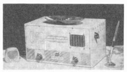
crystal-controlled, and squelch and noise limiting is incorporated. Power input is 5 watts; sensitivity, 1 microvolt. The transceiver operates on 6 or 12 volts d.c., or 117 volts a.c. Price, \$69.95, the kit is furnished complete with all parts, a microphone, and crystals.
