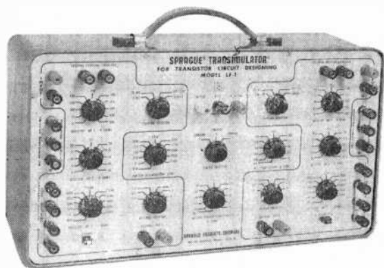
Complete "breadboard" setups for experimenters, such as Sprague's Model LF-1 "Transimulator" shown here, are now becoming available commercially. See text for more details.
