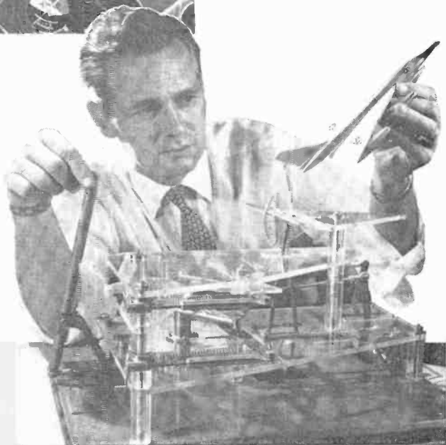
Simplified model of the electro-mechanical linkage used in the B-58's adaptive control system. Designed by Bendix Aviation, this system prevents the pilot from oversteering the plane.
