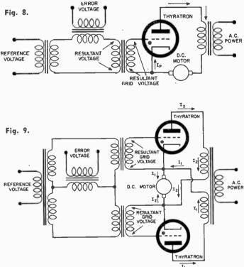
As soon as the error signal appears, the resultant grid voltage undergoes a shift of phase, possibly to the condition given in Fig. 6(C), so that a small current now flows through the motor. This current will drive the motor in the direction which reduces the error signal. If the error signal is larger, the phase shift is correspondingly greater, the conduction interval increases, and the motor turns farther and faster to correct the larger error.
