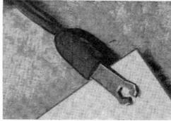
that it is the grounded side. A regular plug may be polarized by splitting and widening the tip of one of its prongs. This widened tip will only fit into the longer—or grounded—side of the a.c. outlet—Ira Glickstein, Brooklyn, N. Y.
