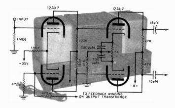
Fig. 7. Acro "Ultra-Linear II" has a cathode-coupled inverter direct-coupled to push-pull triodes. This feature results in an "all push-pull" amplifier.
