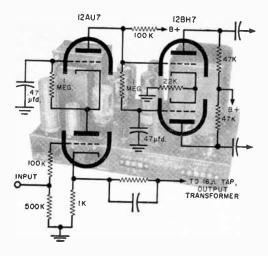
vided evenly between plate and cathode. The output at the cathode is always 180° opposite in phase and equal to that at the plate; therefore, we have the necessary push-pull signal needed to drive a push-pull stage. This inverter is simple and inexpensive, it has low distortion, and with carefully matched plate and cathode resistors, it is capable of well-balanced output. The split-load inverter, however, provides no signal gain.
