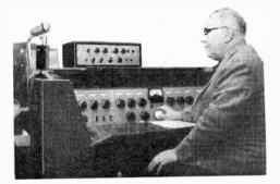
Audio console is "brain" of the TV audio operation. As well as mixing and controlling the many mikes, it can also be used to add reverberation and other special effects to audio portion of show.
