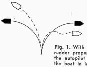
Fig. 1. With left and right rudder properly equalized, the autopilot should move the boat in identical turns to the left or to the right. Dotted lines show the effect of unequal rudder control.
