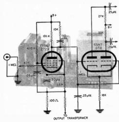
Fig. 5. Mullard circuit as employed in the Eico HF-60 uses a pentode voltage amplifier direct-coupled to a cathode-coupled inverter.
