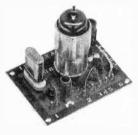
D Tronsmitter Unit (Printed circuit prewired) Oscillator ond amplifier. Crystal controlled .005% tolerance to meet FCC regulations. Requires Unit C for modulation. 6AU8 tube. Shipping weight 2 lbs. Complete with crystal and tube. \$14.50
