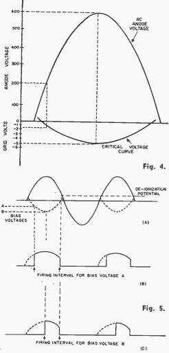
value at the beginning and end of the positive anode voltage half-cycle to a larger value at the peak of the anode swing (Fig. 4). By selecting a bias voltage of the proper magnitude, the thyratron firing can be delayed until a part of the thyratron anode voltage half-cycle is completed. Thus, the average anode current will be less than if the thyratron conducted throughout the entire positive half-cycle.
