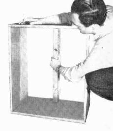
2 Rear 2" x 4" brace is placed with narrow side flush with rear edge of tcp and bottom panels. Two #8 flat-head wood screws and glue should be used at each end to hold 2" x 4" brace in position.
