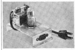
moisture, the photoelectric cell is hermetically sealed in a vacuum tube. Powerhandling capacity, 1000 watts. \$9.95.
