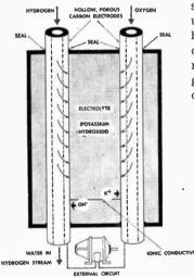
Fig. 1. Operation of the fuel cell. Electron flow from hydrogen electrode to oxygen electrode provides electric current.
