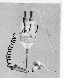
Completed unit is installed in an inexpensive plastic container.
