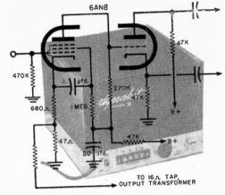
Fig. 4. Dyna "Mark III" power amplifier features a pentode voltage amplifier directcoupled to a tricde split-load inverter. Both functions are handled by one tube, a 6AN8.
