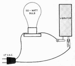
a vibrator that seems to have a sticking reed, connect it to 117 volts a.c. in series with an ordinary 50-watt bulb. By operat-
