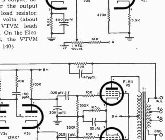
Fig. 14. Eico HF-12 amplifier circuit broken down into its separate sections for the purpose of discussion in the text. Reading from top to bottom, sections are: preamplifier, tone control and power amplifier.
