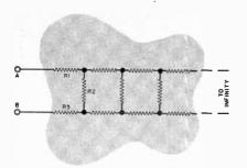
Here is a tricky network consisting of one-ohm resistors with the ladder continuing out to infinity. Joe Homm computed the network's resistance at points A and B in five minutes. Can you?
