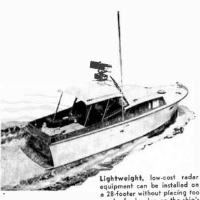
a 28-footer without placing too much of a burden on the ship's battery. (Bendix-Pacific photo)
