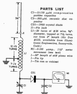
C1. Connect the banded end of CD1 to the plus terminal of M1. Then connect the .005- $\mu$ fd. capacitor (C2) across the meter terminals, and wire the remainder of the connections.
