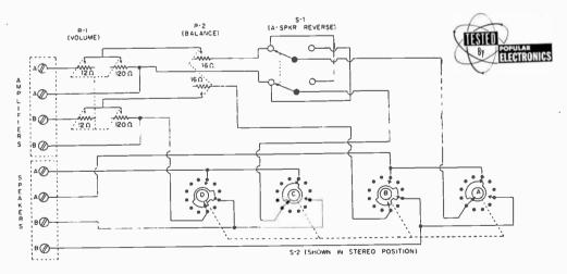
listening to either of the amplifiers on both speakers. The remaining positions provide switching on either channel A only or channel B only for balancing the stereo system.
