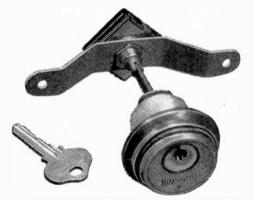
**T** IS often necessary to add a lock switch to an electrical device to prevent its unauthorized use, but sometimes it is difficult to obtain such a switch. An inexpensive substitute can be made from a discarded five-pin tumbler lock of the type used on doors. These locks are of a much better quality than those in most commercial lock switches and have the added advantage that as many keys as desired can be made by the local locksmith.
