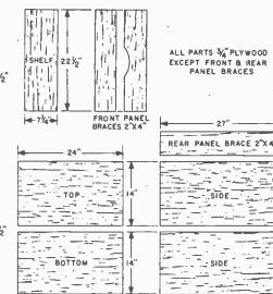
**Construction** of the Reflex 12 is simple since all joints are butted. At left, wooden parts are shown cut to required dimensions. Below is an exploded view of the enclosure's construction.
