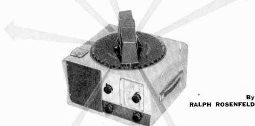
IN TIMES of bad weather and low visi-bility, a radio direction finder can be an invaluable navigational aid, especially for small boats in coastal areas. And it is simple to operate.
