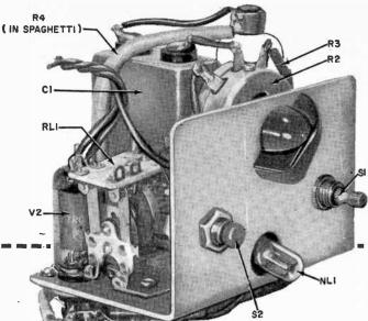
**Construction** of the timer is facilitated by the use of an L-shaped chassis. Unit fits into a 4" x 5" Minibox.
