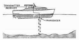
Fig. 1. Depth sounders operate on the principle of sound reflection from the sea bottom. A transducer mounted below the waterline alternately sends out a sound pulse and listens for the echo, with the elapsed time shown on some type of indicator.
