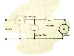
Dewey Dubblecheck, who betieves in making all measurements twice, connected a voltmeter and an ammeter to measure the power drawn in this circuit. Using the formula: W = E × I, he found that the motor drew 40 watts. He made the measurement again, this time using a standard wattmeter, and read only 30 watts. Dewey is puzzled—are you?
