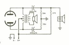
Direct connection of the electrostatic tweeter to the output tubes of an amplifier with push-pull output.
