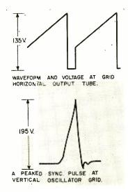
Fig. 7. Typical waveforms (above) from a standard television set.
