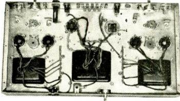
Wire transformer leads in place first. Leads are cut to size and pressed flush with chassis.
