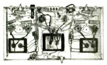
and check the resistances before turning the power on. Very often wiring errors and cold-solder joints can be discovered and corrected before they can cause any harm or grief.
