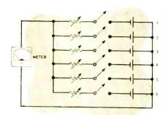
Sam Addit made this simple computer to add any numbers from 1 to 6. The resistors were adjusted so that if battery #1 were switched in, the 0-15 voltmeter would read 1, switching in battery #2 would give a reading of 2, and so on. He figured that if a combination like 2 and 5 were used, the meter would read 7. What did it actually read?
