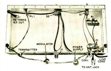
Aluminum chassis after holes are drilled for mounting the modules. Note how the internal wiring of the chassis is led through the 3/8" holes in chassis lip.
