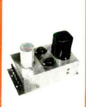
TRANSISTORIZED POWER CON-VERTER - Follow PE's simple directions for converting your 12-volt car battery output to a 117-volt AC supply - providing house current in your car for shaving, ham equipment, etc.!
