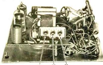
Completely wired unit is at left. Note the three internal adjustment potentiometers. Diagram below is from the construction sheet. Well planned illustrations reduce complex wiring to a simple task.
