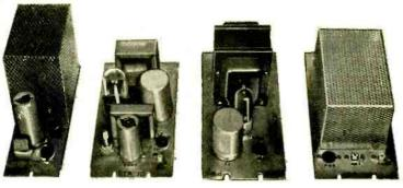
The four modular units in the order that they are installed in the chassis pan. Left to right: transmitter, modulator, power supply, and the converter.
