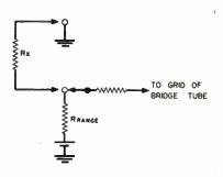
Fig. 10. Simplified input and range circuits of VTVM ohmmeter section.
