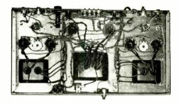
All wiring is in place in the photo at right, prior to connecting the resistors and capaciitors. Completed power amplifier is shown in photo below.
