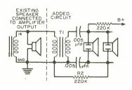
audio voltage. If the audio voltage is too high in relation to the polarizing voltage, the tweeter will overload and distortion will occur. On the other hand, if the polarizing voltage is made too high, the moving diaphragm will are out to the fixed plate. The experimenter may burn out several diaphragms before coming up with the optimum arrangement. Luckily, Saran Wrap is not expensive.
