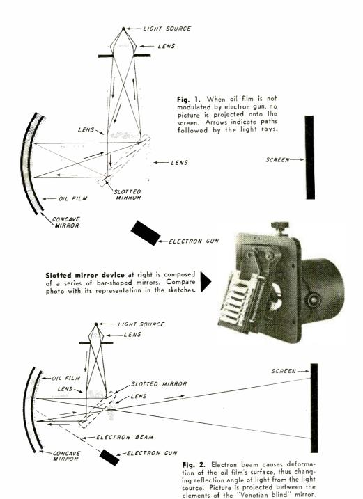
picture between the elements of the slotted mirror. The electron gun uses scanning methods similar to those used in the CRT's of TV sets.
