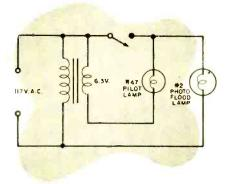
Happy Snap, having only an s.p.s.t. switch, wanted to turn on a flood-light and a pilot light on the control board at the same time. Expecting no trouble, he wired his setup as shown. After double-checking his connections, he held his breath and inserted the wall plug. Things didn't quite work out. Do you have any idea why?
