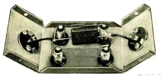
Side panels of cabinet have been folded down only to show internal wiring of Load Box. Note use of rubber grommets to hold pilot lamps and how the wires are soldered directly to the bulbs.
