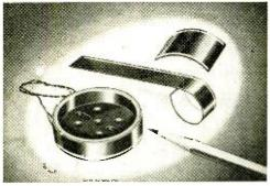
"Contour" photocells and sun batteries are now being made by International Rectifier. See text.
