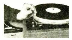
**Position of drive belt** on the platter of Gray HSK-33 is adjusted by loosening or tightening one of the three motor mounting bolts.
