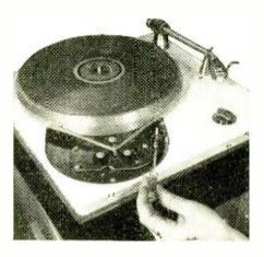
Rek-O-Kut K-33H provides a spring-loaded screw adjustment to increase or decrease tension on the belt which drives the platter.
