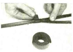
in coming in from the antenna. Don't bare the wires for the direct connection—let the signal be induced from one lead-in to the next. Usually, two or more sets can be coupled together in this manner without adversely affecting reception. If the main lead-in is coax cable or shielded wire, this trick won't work.—Joseph A. Carroll, Brooklyn, N. Y.
