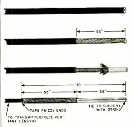
even require a soldered connection! It is called a coaxial ground plane and is constructed from a length of coaxial cable. When mounted in position, the tip of the antenna is suspended from a supporting structure by a length of cord or rope.
