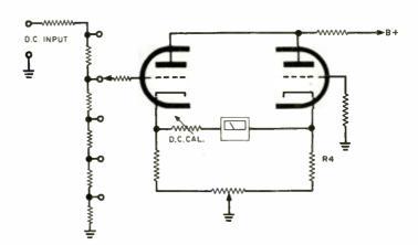
vider tap. The unknown d.c. voltage is now applied to the input grid of the bridge—unbalance of the triodes results and the meter deflects. So much for the d.c. bridge.
