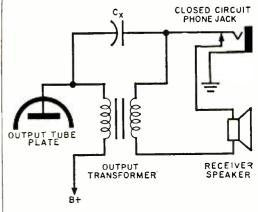
box is not handy) and large size. The simplest method requires but a single capacitor, as shown in the diagram. Capacitor Cx may have a value of from .002  $\mu$ fd. to .1  $\mu$ fd. at 400 volts. This allows the a.c. audio component to pass while blocking the d.c. plate voltage, and thus will provide greatly increased volume when high-im-
