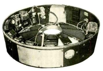
Instrumented payload of "Pioneer" moon rocket includes devices for measuring magnetic fields and the temperature of the vehicle's interior.
