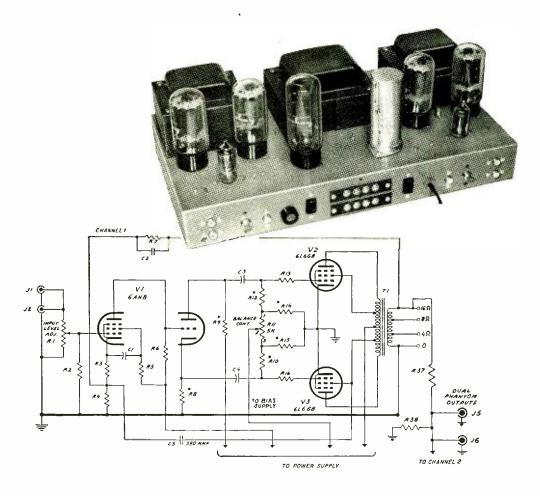
HERE is a fine dual power amplifier for your hi-fi stereo setup. The SPA-55, made by Arkay Radio Kits, Inc., 88-06 Van Wyck Expressway, Richmond Hill, N. Y., offers the hi-fi beginner a top-notch 60-watt monophonic amplifier. And when transition to stereo is desired, dual 30-watt identical amplifiers are available.
