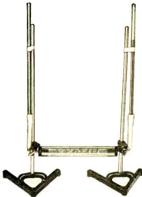
IMPROVED PUMPING UNIT. This is composed of five separate corona-type dielectric pumps "stacked" in glass cylinder to produce more powerful pumping action.
