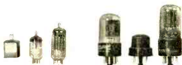
The "active" elements in the VTVM. Standard models usually have a lineup comprising (from left to right) a 50-ma. power supply selenium rectifier, a 6AL5 a.c. rectifier and a 12AU7 bridge tube. An alternate arrangement consists of a 6X5 power rectifier, a 6H6 a.c. rectifier and a 6SN7 bridge tube.
