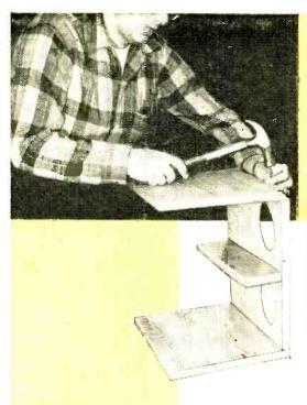
Precut all sections of the cabinet to the sizes specified in the dimensional drawing on page 105. Install the front panel divider exactly between the speaker cutouts and then butt the two side pieces to the plywood front panel. Use 2" finishing nails and a good grade of wood glue on all joints.
