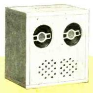
Using a 1/2" wood bit, 36 holes are drilled in the front panel in the area shown in the photo. The exact pattern and spacing of the holes is not im-
