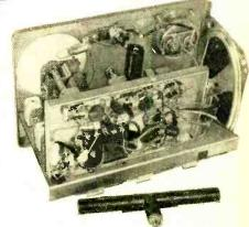
A two-band transistorized receiver, Heath's Model DF-2 uses conventional construction and wiring, with no attempt at subminiaturization.
