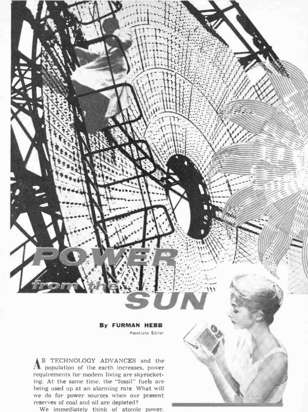
Two contrasting examples of solar applications. At top of page is part of 75-kilowatt solar furnace at Mont Louis, France. Above, solar cells power a Hoffman portable radio.
