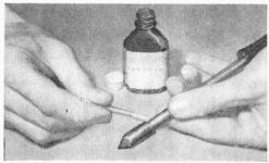
has, don't try to loosen it with pliers—you are liable to damage the tip. Instead, take a cotton swab or brush, dip it in ammonia, and apply it to the tip as shown. This will "unfreeze" the tip in a matter of minutes.
