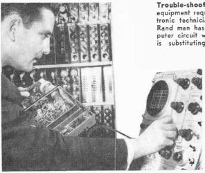
Trouble-shooting highly complex equipment requires a well-trained electronic technician. Here a Remington Rand man has localized a faulty computer circuit with an oscilloscope, and is substituting a new chassis unit.
