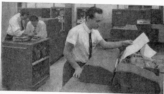
Output data from a computer using magnetic tape can be fed directly to a printer such as the IBM 704 line printer shown here. General Electric is using this equipment in connection with missile development.
