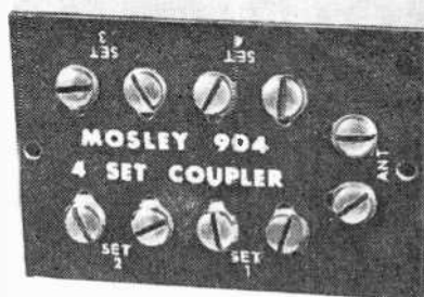
Four-Set TV Coupler. Also a resistor bridging type of coupler for strong signal areas, this enables you to use as many as four separate television sets or combination TV/FM sets on one antenna.
