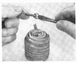
use the compound to hold a nut to the end of a screwdriver or even a piece of wood, such as a dowel, when the nut must be put into a location difficult to reach by hand. -K. M.
