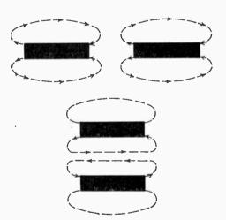
Fig. 8. Two conditions that result in attraction between magnets. In both cases, the directions of the magnetic lines of force are opposed.
