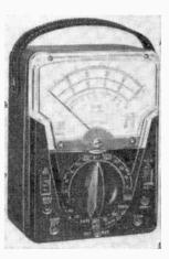
both circuit and range—minimizing wrong settings and burn-outs; and a.c. and d.c. voltage scales of 2.5, 10, 50, 250, 1000, 5000. (*Triplett Electrical Instrument Co.*, Bluffton, Ohio.)
