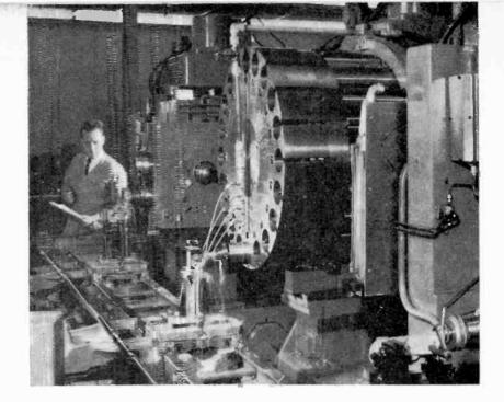
The nation's first all-electronically controlled line of machine tools is installed at Hughes Aircraft in Los Angeles. Working as a team, milling, drilling and boring machines pass parts along automatically after each machine operation. The line is operated by new Digitape electronic controls and was developed in cooperation with the Kearny & Trecker Corp., of Milwaukee.
