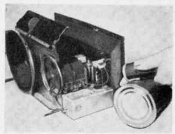
old plunger-type insecticide gun for the job. It saves plugging in and setting up the vacuum cleaner, yet does the job just as thoroughly. Make certain the gun is empty, however, or you may spray "bugs" into your equipment rather than prevent the possibility of them forming due to dust and dirt! J. A. C.
