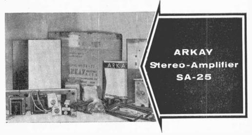
amplifier comprises a 20-watt "superlinear" amplifier with the Williamson circuit arrangement plus tone controls and two preamp-equalizing sections. The first preamp feeds the Williamson power amplifier; the second feeds a 6C4 tube wired as a cathode-follower output. The output from this second channel can be used to drive an additional basic amplifier and speaker system for stereo.
