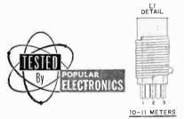
II TURNS #20 PLASTIC COVERED HOOK-UP WIRE TAPPED AT 23/4 TURNS FROM BOTTOM
