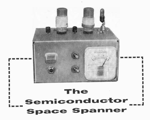
A challenge to your operating skill, this 96-milliwatt transistor transmitter operates on 15 and 10 meters
