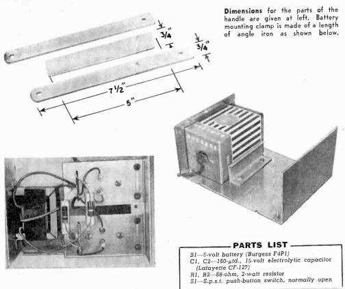
Placement of the heat sinks and transformet is shown in photo above. Note that the collectors of both transistors used in the Transihorn are connected internally to shell.
