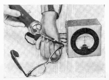
Hearing aids take on a new dimension with the debut of the new Zenith Solaris unit, which employs silicon solar cells (same type as used in the Vanguard satellite) to power its amplifier. The cells are so efficient that they can even use the weak light of a ashlight to register a voltage. Overcast sunlight will run the device properly. In darkness, it automatically switches to batteries. It uses four transistors.
