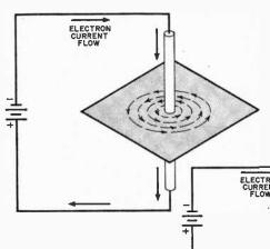
Fig. 1. The magnetic effect of a current passing down through a vertical wire. Iron filings sprinkled on cardboard sheet trace out the magnetic forces.
