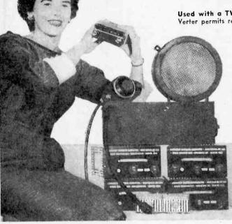
The young lady above is holding a new all-transistor auto-portable receiver which may be used either in or out of an automobile. Compare this in size with the 1929 Cadillac auto radio shown with its B batteries.
