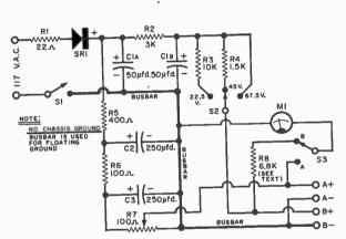
45, or 67½ volts for the "B" voltage. It has a built-in meter for reading either output *while in use.* A compact unit which can be built in a Bud Minibox cabinet, its total cost including the meter should be below \$15.00.
