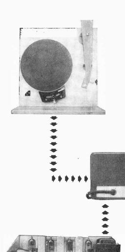
pickups are in this category. Crystal pickups, tape recorders (with their own preamplifiers) and tuners have an output voltage of from 0.5 to as high as 10 volts, or medium-level signals.
