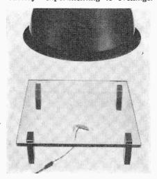
Both 100-watt and 200-watt bulbs are commonly used as sun substitutes. If they are placed too close to the "sun batteries," however, the cells will be subject to heat in excess of the manufacturer's limit.
