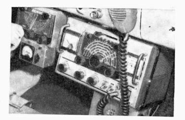
Typical mobile installation located under the instrument panel in the front seat of a car,
