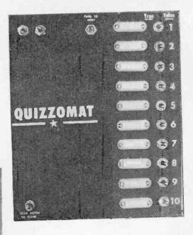
Quizzomat front panel above shows the parts layout to be followed. The two switches on the upper left side of the panel set the "programing" which determines the "right" and "wrong" sequence for each topic sheet. Note that the timing and scoring circuit components are mounted on the inside aprons of the chassis box (below).
