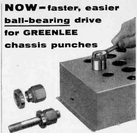
New GREENLEE Ball-Bearing Drive Nuts and Drive Screws reduce friction and make it easier than ever to cut smooth, accurate holes with GREENLEE NO. 730 round Radio Chassis Punches. The new faster drives are available for all round-type GREENLEE Punches sizes 11/16" through 2-25/32". Operate with ordinary wrench for quick socket openings etc. in metal, bakelite, or hard rubber.
