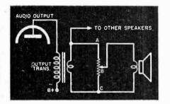
Fig. 1. Pot used as a speaker volume control (not recommended).
