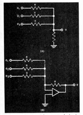
Fig. 1. Analog computer feeds value measurements into input (A), where e is analog of sum of voltages e1, e2, e3. In (B), amplifier is shown in circuit.
