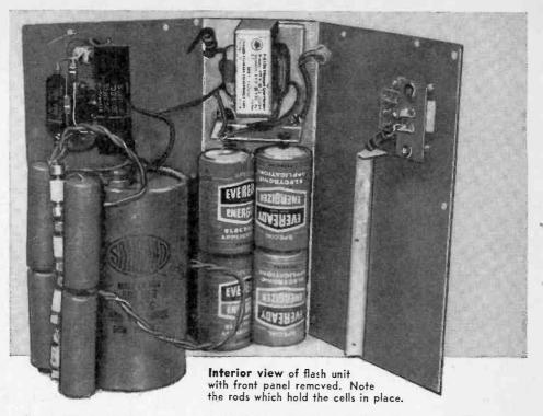
as we'd like it. The electronic photoflash outfit described here is a good and comparatively inexpensive compromise. It operates from either house current or from four inexpensive size D flashlight cells, so battery cost is trifling. It's a single unit, easy to build, rugged and dependable in operation. The photoflash tube is mounted in neoprene under a glass dome to protect it from injury.
