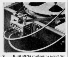
In-line stereo attachment to convert most popular make tape recorders without alteration. It consists of in-line stereo head, tape guides, pressure plate and mounting hardware. Cables feed recorder and amplifier. Dactron Steradapter 4902.
