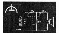
(transformer secondary and voice coil). It should be remembered that a comparatively high resistance in parallel with a low resistance produces very little change in the total circuit resistance. In this connection, then, the T-pad produces very little attenuation (about 1 db) and the output signal is just about as loud as it was before the pad was inserted.
