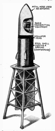
**Proposed design** of the Moon Rocket. A radio transmitter, in the nose, will send out waves continually on its course.
