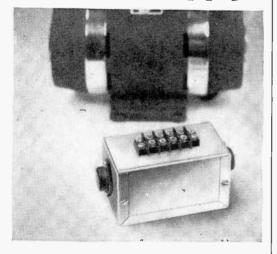
Easy to build, this modern power supply is as big in performance as it is little in size. Two CBS 2N256 power transistors, operating from a 12-volt battery, deliver 450 and 250 volts simultaneously. Combined output is 40 watts continuous service.
