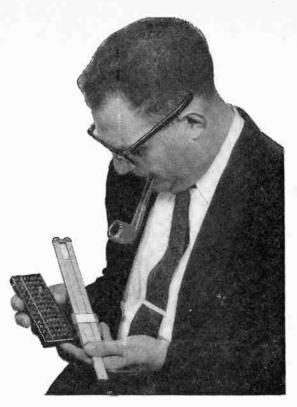
rule, you do the same thing mechanically, for a slide rule is only a table of logarithms. The slide rule, then, is an analog computer.
