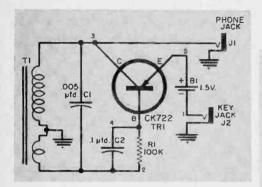
which it can be helpful. With the inexpensive transistors now available, it is easy to build a battery-operated oscillator tiny enough to fit in your pocket and have a battery life of a year or more.
