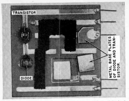
Greatly enlarged photo of thumbnailsize flip-flop circuit. The actual size is indicated on the first page of this article. As can be seen from the schematic diagram on the opposite page, the circuit is made up of two transistors, two diodes, eight resistors and two capacitors.
