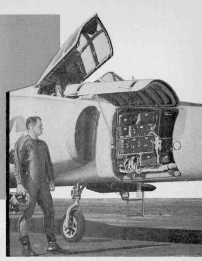
**Digital computer**s tend to be large, but some have been put in small packages, as in this Hughes Aircraft model in the fighter plane above. At left, above, two forms of basic computers are shown being examined; the abacus is actually a digital computer, while the slide rule is an analog computer.
