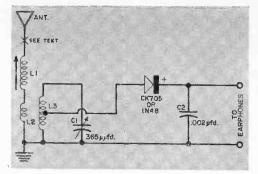
at 30 turns. Leave a  $\frac{3}{16}''$  space between coils. If you use an antenna that *is* over 75' long, insert a 3-30  $\mu\mu$ fd. trimmer at point "X." —Jim Brooks
