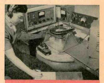
A permanent record of test figures of wow, flutter and rumble is sept on all changers. Meter at left measures wow directly in percentages. Flutter is checked on same equipment. Meter at right measures rumble, rated below audibility on the changer. Operator monitors test record tone with earphones. Finally, dielectric safety test of motor and wiring is made with center meter.
