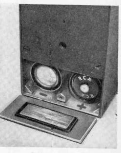
Battery installation; note the polarity markings and insulated contact plate.
