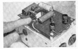
Transistor amplifier subassembly with RLI and standoff mounts.
