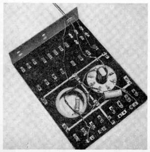
wood sub-base, using the same center. Then cut several 3" discs of Bakelite and mount the desired tube sockets in the center of the discs. Wire small Fahnestock clips on base panel for each tube prong. Each of these subassemblies will fit in the holes in the Bakelite base, resting on the plywood sub-base, with the tube prong clips on the top.
