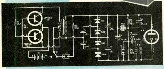
leaves only the four silicon rectifiers and the four capacitors (C1, C2, C3 and C4) of the voltage quadrupler. They also are prewired, using a physical layout which corresponds with the placement shown in the schematic. Considerable space is saved by using pigtails on the rectifiers instead of mountings clips.
