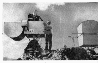
Scanning photoelectric photometer selects and measures the intensity of light too faint for the human eye and records its changes. This airglow camera is at Fritz Peak, Colorado.
