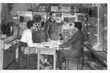
Measuring telemetered data from rockets in flight at an installation in Manitoba, Canada. At the far left is a telemetry recorder which takes data from airborne rockets; in the center is the main recorder which puts data on tape; the ballistic camera master control is at the right.
