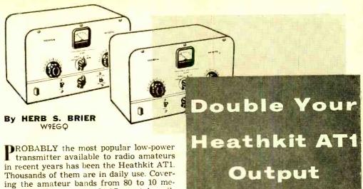
PROBABLY the most popular low-power transmitter available to radio amateurs in recent years has been the Heathkit AT1. Thousands of them are in daily use. Covering the amateur bands from 80 to 10 meters, the AT1 uses a 6AG7 crystal oscillator to drive a 6L6-G amplifier/frequency doubler to about 30 watts input. To insure stability, the 6L6 is operated as a frequency doubler on the bands above 80 meters and power output is no more than 10 watts on the 40-, 20-, 15-, and 10-meter bands.
