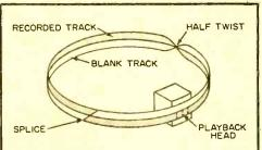
To repeat message, with silent period interspersed, use method shown above. Before splicing the two ends of your tape segment, put a half twist in it. When the tape plays, the message will be heard the first time around. When the splice passes the head, the tape will be turned around and the blank area will pass the head. Incidentally, this type of loop is known as a "Mobius strip" and is a mathematical oddity because it has, effectively, two surfaces bounded by a single curve.
