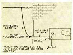
lead-in. The inner conductor is soldered to the outdoor lead-in at one end and connected to the receiver antenna post at the other end. The shield should be connected to the chassis and the outer end taped up to prevent contact with the building. (See drawing above for details.)
