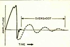
Showing damping problem graphically, the solid line represents the signal of a sharp sound burst (for instance, a drum beat). Improperly damped speaker keeps jiggling (dotted line) after actual sound stops. Extra undulations, called "overshoot," muddy the tone.
