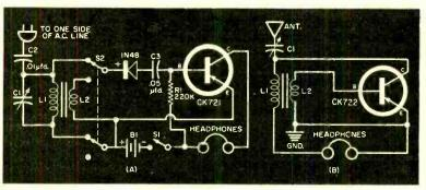
Fig. 1. Two simple receiver circuits submitted by our readers: (A) Richard Taylor's variable selectivity receiver and (B) Mike Swink's self-powered radio.
