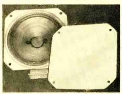
the speaker mounting holes and fasten with  $6-32 \times 14$ " machine screws. When the project is completed, remove the cardboard sheet and install the loudspeaker in its enclosure. —J.E.P.
