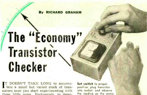
It DOESN'T TAKE LONG to accumulate a small but varied stock of transistors once you start experimenting with these little gems. Fortunately, to determine whether a transistor is good or bad requires a tester of extreme simplicity. The "Economy" Transistor Checker performs two sensitive tests which will quickly tell you if a transistor has been damaged due to overload or contamination of the germanium, whether the transistor is shorted or open-circuited, or if it is just excessively leaky.\*
