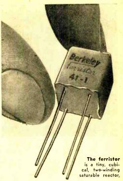
inductive reactance of *any* coil diminishes as saturation is approached. At this point, the r.f. winding circuit becomes series resonant, and its total impedance drops so low that enough r.f. current flows to saturate the ferristor even in the absence of control current in *L2*. This is a stable state in which the ferristor persists as long as nothing is done to change it; the name "full-on" is often applied to such a condition.
