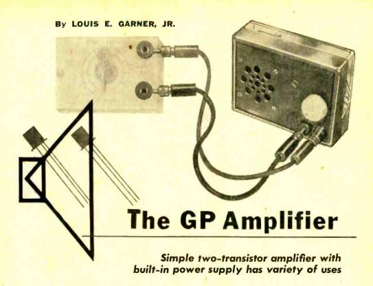
A SIDE from standard test equipment, one of the most valuable home electronics workshop gadgets is the general-purpose audio amplifier with a built-in loudspeaker. You can use it as an audio signal tracer to track down hum in hi-fi systems or defects in p.a. or phonograph amplifiers. Combine it with a simple r.f. detector probe and it becomes an r.f. signal tracer. Entertainment-wise, it may be connected in place of headphones to a small receiver to provide loudspeaker operation.
