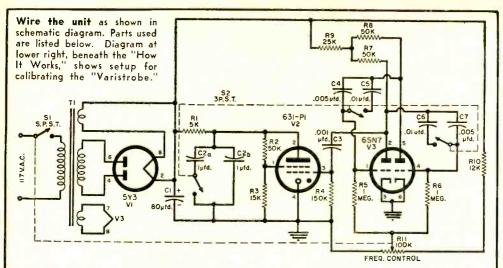
C1—80-µfd., 450-volt capacitor (Sprague TVL-1735, twistlok type, can ground)
