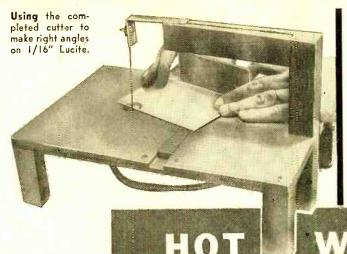
Slice thin sheet plastic with this easily constructed precision cutter
