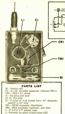
the box is a tuning capacitor, C1; this is an ordinary  $9-\mu\mu$ fd. midget capacitor.
