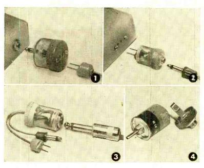
for the first three adapters and a tin container with the fourth unit. each having a friction lid. All cutting should be done with a finetooth, narrowblade hacksaw. Although Lafayette Radio catalog numbers are specified in most cases, a Telex Type 9231 plug may be substituted in the first adapter, and a Type 9240 miniature jack and mating plug could be employed with the second adapter. -Art Trauffer
