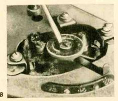
C To clean the driving mechanism, wipe the parts with a cloth soaked in carbon tetrachloride. If the rollers are glazed, causing slippage during operation, rub them gently with a fine grade of sandpaper or emery cloth. Idlers with "flats" or other obvious defects must then be replaced.
