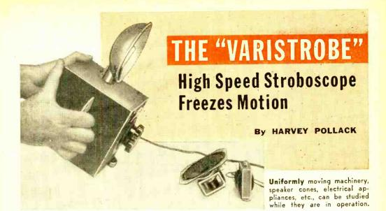
WOULD YOU LIKE to examine the contortions of your high-speed circular saw, drill or bandsaw under conditions that seem to slow it down to a crawl? Any repetitive movement, whether rotary or reciprocating, can be viewed as though the moving body were at rest or in very lazy motion—under the flashing illumination of this wide-range "Varistrobe" (variable flash-rate stroboscope).
