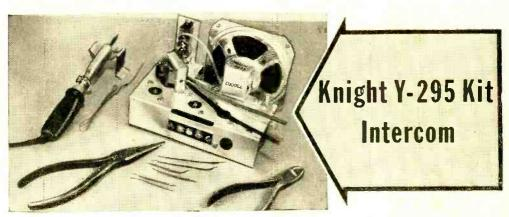
comes complete with all the electronic components needed to assemble a two-station system, including 50 feet of three-wire interconnecting cable—more than ample for most installations.
