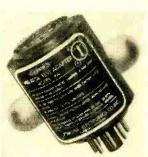
lights will be out. Model 4A (shown in photo) checks any standard 4-prong vibrator, 6- or 12-volt A-Base shunt-driven coil; Model 3D checks any standard 3-prong vibrator, 12-volt D-Base shunt-driven coil. (Pomona Electronics Co., Inc., 1126 W. Fifth Ave., Pomona, Calif.)
