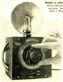
Model is attractively housed in black wrinkle steel cabinet with panel decals, a high-quality knob and vernier indicator, and a carrying handle. The 5"-diameter parabolic reflector, taken from a Bower pocket flash unit, slips easily over the strobotron.
