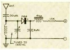
frequency of a local high-power AM broad-caster—I detected the signal through a 1N64 crystal diode and filtered it out via a 4-henry choke and a 8.0- $\mu$ fd. capacitor. This provided me with a power supply of 300 microamperes at 3 volts, or 1000  $\mu$ a. at 0.8 volt—enough for rough experimental work.
