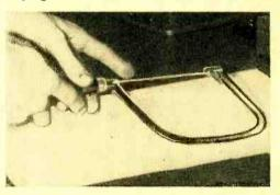
all sides of the blade rather than along one face, it simplifies cutting wood, plastic, and particularly aluminum. -C.C.
