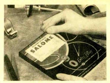
Messages of moderately long duration are put on continuous tape as shown below. Run tape over edge of table and hang empty reel on it. This provides enough weight to keep tape running smoothly. Be sure that tape does not pull away from recording head during the process or you'll lose some signal strength.
