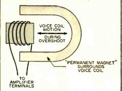
Loudspeaker coil moving against stationary magnet during "overshoot" acts as electric generator, causing current to flow back to amplifier. With proper damping, this current itself helps to check the overshoot.
