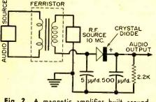
Fig. 2. A magnetic amplifier built around a ferristor. Amplification is achieved without use of either vacuum tubes or transistors.
