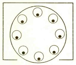
In strobe pattern above, black circles seem to rotate inside larger circles as disc is whirled under stroboscopic light of slightly higher or lower frequency than rpm of motor rotating the disc.
