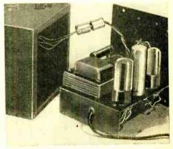
Components are mounted as shown here. Miniature cable connectors which join the four leads that go to strobotron socket on top of case make it simple to remove chassis for inspection or repairs.
