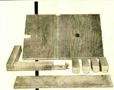
Disassembled view. Note position of feedthrough holes with respect to miter guide groove.
