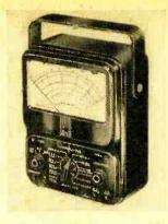
The Simpson Model 260 voltohm-milliammeter is useful for ohmmeter transistor tests.
