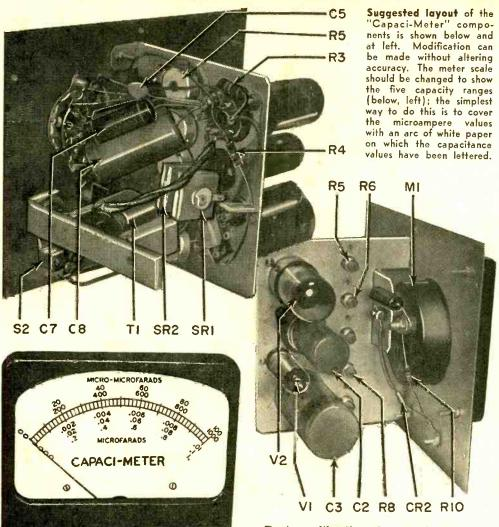
flected to full scale. Make this adjustment going toward full deflection rather than returning from beyond full scale. Follow this same procedure with each of the other standards (1000  $\mu\mu$ fd. and 0.01  $\mu$ fd.) for the respective range positions, and the calibration is complete.
