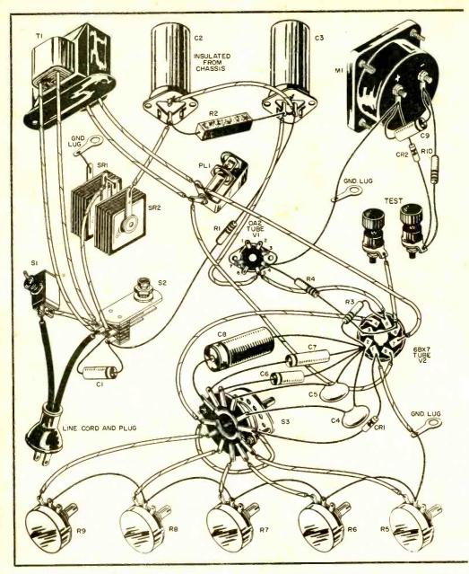
with a pair of pliers when soldering to prevent heat damage to the sensitive crystal. Check the wiring very carefully before turning the instrument on to avoid any possibilities of mistakes which might damage the meter. If all seems correct, turn the five potentiometers to the position which places maximum resistance in the circuit. Plug in the unit and turn it on.
