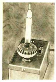
check to make sure the bubble tube is pushed down firmly against the lamp in the base. These units operate on the heat thrown off by the lamp, so a snug contact between bubble tube and lamp is necessary. Two out of three of the author's lights started and operated perfectly with this arrangement.
