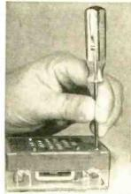
grasp its *shaft* between your thumb and forefinger. You'll find that you can control it quite easily, with a truly "delicate touch." You can spin it back and forth rapidly, but it is almost impossible to apply enough torque to damage miniature screws.
