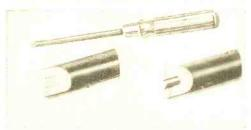
metal tubing supplied by Superior Tube Company, Norristown, Pa., it has a hollow blade which houses a secondary rotating blade. The tip of the secondary blade is located in a cut-out portion of the primary blade (as shown in close-up view at the left). Pushing the screwdriver handle turns the second blade at right angles to the width of the primary blade (see close-up view at right) to wedge it tightly against edges of the screw slot. (Hunter Tool Company, Los Angeles, Calif.)
