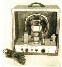
Rear view of amplifier case shows placement of the speaker and amplifier chassis. The gain control and jack for harmonica pickup are on the panel.
