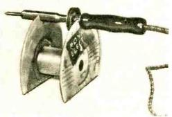
venient work. A suitable holder may be fashioned quite readily from an empty 6" metal wire reel. Such reels are available from radio or electrical supply houses. Simply cut off a section from each of the flanges on the reel, and then cut out the apposite sides to hold the iron.
