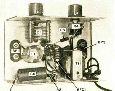
Placing the preselector stage in the receiver is usually an impossible task, but it can be conveniently made up on a small box and mounted atop the receiver. In this case, it is constructed on a 3" x 4" x 6" aluminum box, as shown above.
