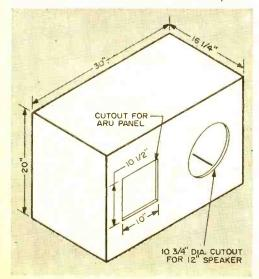
as one adequate solution to this problem, can smooth that bump and provide good clean bass. Yet many an attempt to construct what seems to be a very simple enclosure of this type ends up as little more than a "boom box." Then, too, the dimensions of such enclosures (minimum of 10,000 cubic inches for a 12" speaker) have stopped many hi-fi'ers cold.
