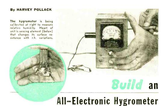
NEW PLASTIC humidity sensing element now makes it possible for you to build an electronic hygrometer for measuring relative humidity (r.h.). It can be used in your home, outside the house, in the egg incubator, in your refrigerator or freezer, or any other place where air moisture is significant. It combines the convenience of a hair hygrometer with the accuracy of the wet-and-dry bulb thermometer.
