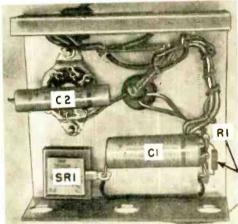
Two views of open-end chassis. Top view identifies enclosed-type relay RLI, isolation transformer TI, meter MI, and potentiometers R2 and R3. Underchassis view shows placement of selenium rectifier SRI, resistor RI, and capacitors CI and C2,
