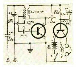
circuit in the wiring schematic represents a combination of the regenerative receiver described in Part 1 with the two-stage high-gain receiver in Part 2. It provides more gain than either circuit alone and will pick up strong nearby stations.
