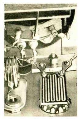
Close-up view of the El-Tronics sensor plate.
