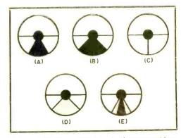
Voltage indications: (A) normal adjustment with no voltage applied to probe; (B) positive d.c. voltage—"eye" will change for a voltage as low as 0.5 volt, will open completely on about 20 volts; (C) negative d.c. voltage—"eye" will change for 0.5 volt, close on about 10 volts; (D) a.c. voltages as low as 0.5 volt rms will show some partial illumination; (E) a.f. peak voltages as low as 1 volt will be indicated, partial illumination varying with the signal voltage.
