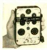
be the ideal answer to the open - filament locating problem now encountered in TV sets which useseries-string tubes. Completely self-contained and battery-powered, it provides a quick check of
