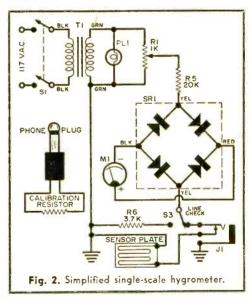
horizontal axis. Using resistors from about 100,000 ohms up to about 1.4 megohms, with switch S2 set on LOW, repeat the procedure above. Make the graph small enough to be cemented to side of case for easy reference as shown in photos.
