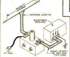
Fig. 4. How preselector is connected to receiver. For reception below 11.5 mc., preselector must be removed from antenna circuit.
