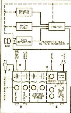
Block diagram of hi-fi system at left shows typical signal path connections (solid lines) and grounding bus (broken line). Apply grounding bus experimentally to each chassis, and to water pipe, since such connections may increase—rather than decrease—hum.
