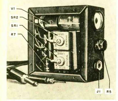
With the "magic-eye" tester, you can probe any point in a radio, television set or other electronic device from less than 0.5 to 500 volts. The "magic eye" indicates whether voltage is positive or negative d.c. or a.c. and differentiates between low and high d.c. voltages. At left, the unit is shown with power supply installed and major components identified. Capacitors are mounted on the other side of the Micarta insulating board.
