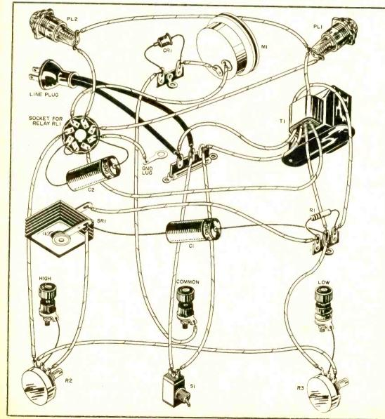
are connected between low (+) and common (-), those from 221/2 volts to 90 volts between high (+) and common (-). You should be able to run the current from a small value to 5 milliamperes or more.
