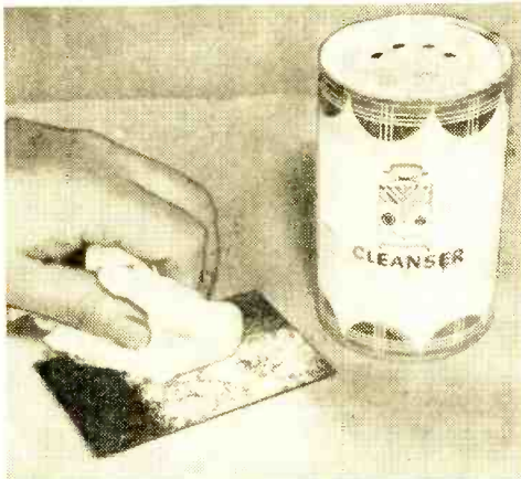
Clean the copper-clad phenolic wiring board of dirt and tarnish prior to applying the resist.
