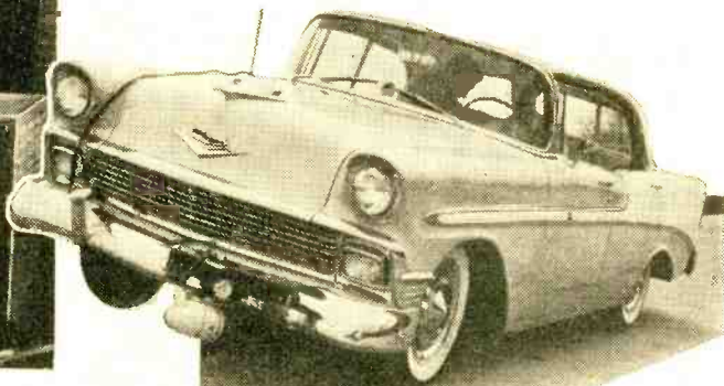
Action of underchassis spring is observed on TV screen located in rear of the car while vehicle undergoes strenuous road test.
