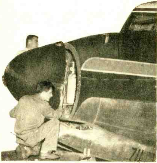
Radome nose , made of special plastic transparent to microwave radiation with only minimum power loss, is bolted onto the fuselage of Delta airliner housing the first commercial Collins Airborne Weather Radar. With radome removed, you can see antenna at right.
