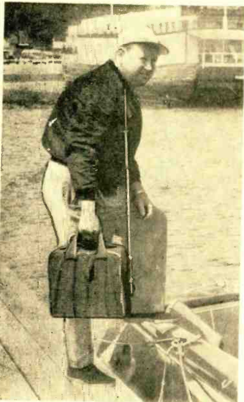
This bag totes a medium-frequency radiotelephone good for a hundred miles under favorable conditions. The "center-loaded" whip antenna telescopes into a socket on the side of the equipment, which is made by Sonar Radio Corporation. Unzip the cover, extend the antenna, connect ground, and you're ready to operate the portable six-channel unit.
