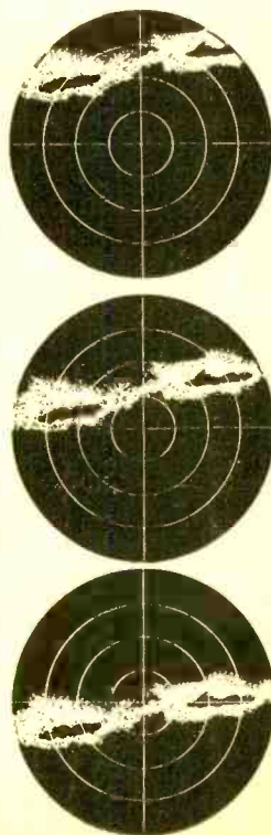
Compact cockpit control features special adjustment to gage cloud density, turbulence and force of precipitation.
