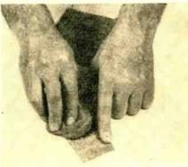
Tinning the tip of the soldering gun insures quickest possible transfer of heat from tool to work. Steel wool may be used to clean flat surfaces of metal; proper soldering flux removes oxidized surface film.
