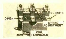
Screw adjustments vary the relay's sensitivity. Center screw alters spring tension; outer ones change gaps on "open" and "closed" contacts.
