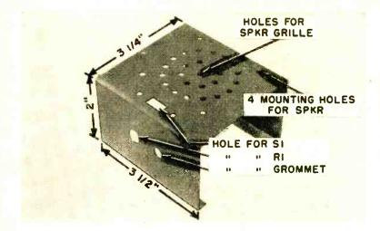
Enclosure is cut down from standard aluminum chassis. Exact hole sizes and spacings must be determined from the specific components which you use in building this unit.
