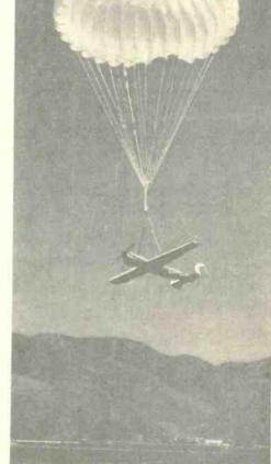
Radar corner reflectors in wing-tip appendages of drone insure that radarcontrolled guns receive echo from craft.
