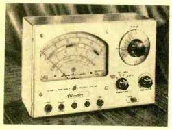
r.f. signal tracer and an audio signal tracer. Specifications include: eight d.c. voltage ranges (at a sensitivity of 20,000 ohms per volt); seven a.c. voltage ranges (5000 ohms per volt); three resistance ranges, two capacity ranges, five d.c. current ranges and three decibel ranges. (Superior Instrument Co., 2435 White Plains Rd., New York 67, N. Y.)
