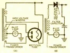
shown in the diagram (A), will act as both a pilot light and a fuse. The lamp should have a current rating approximating the amount of current drawn from the supply. For instance, a 60-milliampere lamp may be used if a current of 50 to 60 milliamperes is being drawn.
