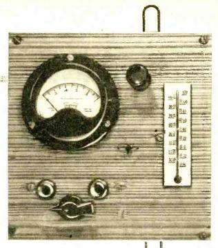
battery, and other necessary components as indicated in the parts list and photographs. You can mount these components in just about any way you wish—there are no tubes or transistors involved, and only a small amount of d.c. current is required. As the battery will have to be replaced occasionally, arrange your mounting so that such replacement won't be too difficult.
