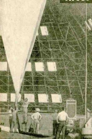
sounding." Large, free-flight balloons carry mobile transmitters over thousands of miles. Meteorological data is reported regularly, while standard position-finding techniques keep track of the flight path.
