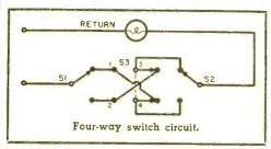
which the same light or outlet may be controlled independently from only one of three different positions. The four-way switch (83) shown in the drawing is really a double-pole, double-throw type with crossover connections between outer poles.
