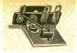
Transister-mounting assembly can be made by bending a piece of scrap aluminum to hold 3-lug terminal strip and 5-pin subminiature tube socket.
