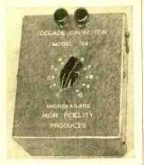
ers, tuned circuits, etc. It is housed in a gray hammertone finished aluminum case 4" wide, 5" long, and 3" high. Net price of the Model 100 is \$9.95.
