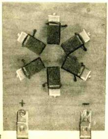
rangement) or more current at the same voltage (parallel arrangement). The best layout plan for five or six B2M cells has been a circle; this type of circuit has the advantage of receiving maximum light from the sun when used outdoors and an equal light distribution from a ceiling spotlight when used indoors.
