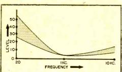
Fig. 1. Too much boost (shaded area) caused by running tape through loudness control twice (during recording and playback).
