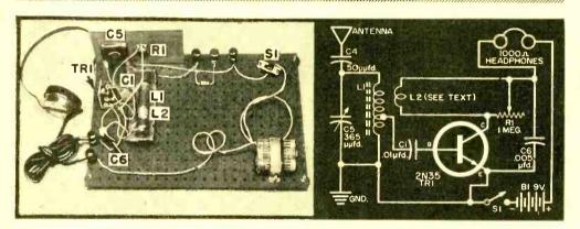
You can greatly increase the sensitivity of the receivers shown in projects 2 and 3 by adding regenerative feedback. A couple of simple wiring changes will do the trick.
