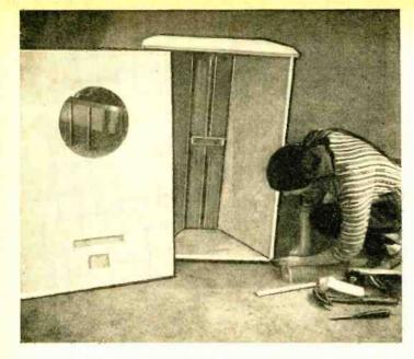
Rubber weather stripping is cemented to front edges of top, side, and bottom panels. This stripping helps secure fit of front panel which is screwed in place last. Fourteen screw holes are pre-drilled; roundhead screws are supplied in kit. Some skewing may be required to get an exact fit; the plane was used to shave off an overlap of about 3/32" on one edge.
