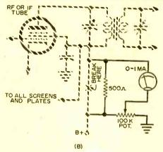
the meter sensitivity. The larger the resistor, the greater the potential difference across it. Of course, the meter sensitivity will affect the amount of meter deflection.
