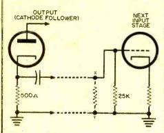
Fig. 2. Correct impedance level, after cathode-follower output, must be no lower than 25,000 ohms (between points x and y).
