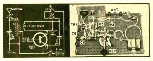
If you've ever built a regenerative receiver like the one shown opposite, you know that misadjustment of the feedback potentionneter can make the set squeal like a stuck pig.
