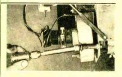
A socket wrench, or nut driver, is handiest in a case like this where a nut rather than a screw head is made accessible for adjustment. The hollow shaft of the driver "swallows" the part of the bolt that projects beyond the nut.
