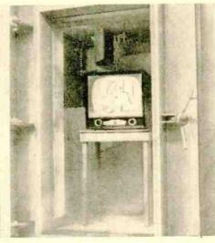
Heat and humidity tests are carried out in a vault-like chamber where temperature and moisture can be completely controlled by the test engineer.
