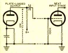
Fig. 3. Plate-loaded output of typical triode has impedance of about 10,000 ohms. Next input must be at least 100,000 ohms.
