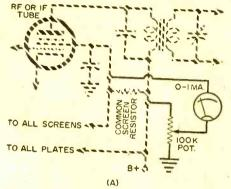
raising their plate or screen voltages. If, using a meter, this varying B+ voltage is compared to a fixed voltage, the meter will deflect more or less as the voltage difference between the two points varies.
