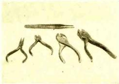
Pliers and nippers in full assortment could fill a large tool chest, but a good general-purpose kit should have at least one pair of tweezers (top) and, left to right, long-nose pliers, diagonal cutters, slip-jaw or "gas" pliers, and parallel-jaw pliers.
