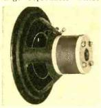
cone is sectioned and a mechanical crossover is used to separate highs and lows. Cloth suspension of the cone improves bass response. With a five-pound magnet, the 215 can handle power peaks up to 20 watts. Net price is \$65.00. (Hartley Products Co., 521 E. 162nd St., New York 51, N. Y.)
