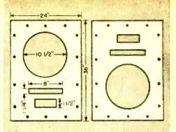
When single-cone or coaxial speaker is used, fit front panel so that the large circular hole is at top; cutouts remain blocked. With two-way or three-way system, mount front panel so that the large opening is at the bottom; unblock the cutouts to accommodate squawker and tweeter units.
