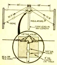
OVICES operating 80 and 40 meters often find that they have an antenna problem. The coaxial-fed dipole will only work on the fundamental or odd-order harmonic frequencies. A 130-foot antenna cut for 3700 kc. will not work on the 40-meter hand.
