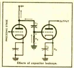
tube positive with respect to ground. During normal operation, negative grid bias for this tube is developed by the voltage drop across Rk. The leakage current is likely to produce a voltage that more than cancels the grid bias, producing distortion.
