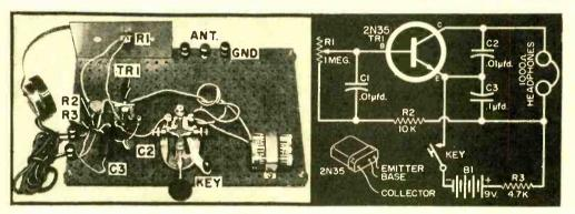
For learning the sound and touch of a radio ham's second language, nothing takes the place of a code-practice oscillator. This simple job has as good a tone as any you'll find, and being transistorized, it can keep pouring out *dits* and *dahs* practically forever on its original power supply.
