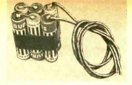
**Power pack** is a 9-volt battery made up of six series-connected penlite cells. You can tape the cells together as shown or fit them into standard clips.
