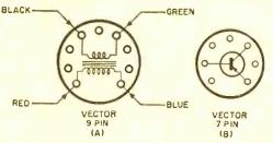
identified by The Vector Company as No. 7P and No. 9P respectively. The transistors and transformers were secured to the central plastic pillar of the plug with a drop of airplane cement. To separate the transistors and the transformers, a 7-pin plug was used for the transistors and a 9-pin plug for the transformers, making them in-
