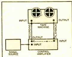
Fig. 4. This type of "circular conneccould cause positive feedback. tion"
