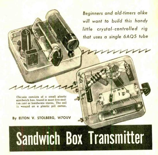
THIS inexpensive little transmitter consists of a one-tube crystal oscillator using a 6AQ5. It is a very active oscillator having plenty of output even with the most stubborn crystals. Incidentally, this circuit can be made to double and even quadruple the crystal frequency with good output.
