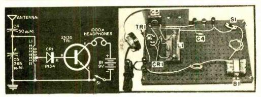
Though this simple receiver has a lot more gain than a crystal set, it still needs a good antenna and a ground for best results. A commercially available "transistor antenna coil"—tapped to provide a good impedance match to the input of the transistor—is used in the tuned circuit.
