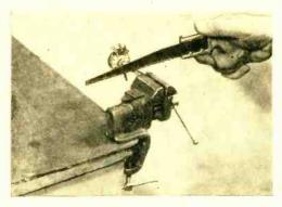
For clean, safe cutting, make sure the part you're working on can't slip or twist. A lazy short cut—like holding a shaft in your fingers while you saw it down to size—is more apt to shave your fingers than it is to shorten the work.
