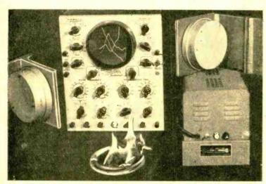
Fire moves air, too. so it can be detected by the ultrasonic alarm. Here, an oscilloscope has been substituted for the alarm, and frequency disturbance is indicated on the screen. Greater sensitivity is needed where the system is used as a fire alarm; setting can be adjusted by means of a knob on the master control chassis.
