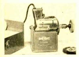
An electric drill becomes much more than a hole-making tool when you add a stand and attachments for grinding, buffing, wire-brushing, sandpapering, and other jobs. Most of the common drill attachments are made to fit quarter-inch chucks.
