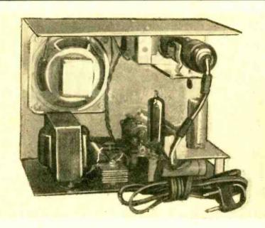
The internal power supply of this unit consists of a miniature power transformer T1, a 75-milliampere selenium rectifier SR1, filter resistor R7, and electrolytic filter capacitors C5 and C6. No pilot light is used, since the glow of the magic-eye tube serves the same purpose.
