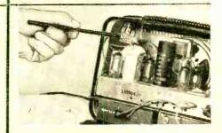
Non-conductive shafts keep your hands at a distance from frequency-sensitive peaking screws. Tips are often made of soft material; if you exert too much pressure, they'll break before they can seriously damage the screws.
