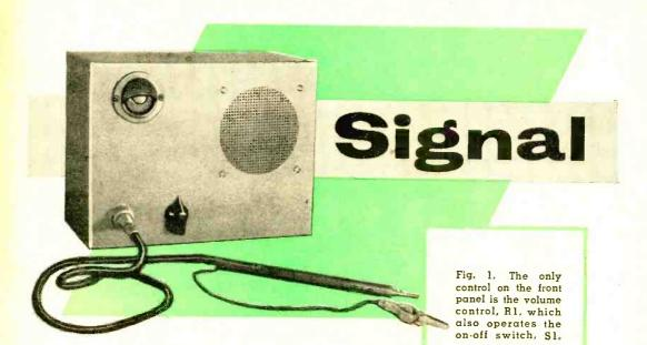
MANY service technicians rate signal tracing as the most useful technique ever developed for fast trouble-shooting. A signal tracer doesn't have to be tuned, and you don't need an engineering degree to understand how it works. In fact, a tracer is easier to handle than some meters; it can be used to locate trouble in radio, TV, audio, and other equipment.
