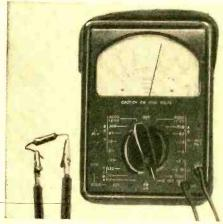
the accuracy of the ohmmeter calibration. Ideally, one should be on hand for each range, and should be so chosen as to fall between 10% and 90% of the scale reading, preferably towards the low side of the scale. The photo shows an ohmmeter being checked using a precision resistor.
