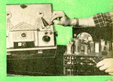
A phonograph using a high-level pickup (crystal or ceramic) may be taped by feeding its signal into the machine's high-level jack. Phenographs using low-level pickups (magnetic) should feed into a preamplifier-equalizer and then into the tape machine. A low-level magnetic phono signal may be fed into the tape recorder's low-level jack, but this does not assure proper phono equalization and is not recommended.
