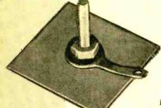
A SINGLE plate taken from the common selenium rectifier makes a surprisingly good self-generating photocell. While a burned-out rectifier will yield at least one or more plates that are in operating condition, a new rectifier will supply six excellent plates. With a rectifier costing about one dollar, this makes the home-made photocell very cheap indeed.
