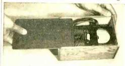
multitester in a simple plywood box will provide protection from both shock and dust
