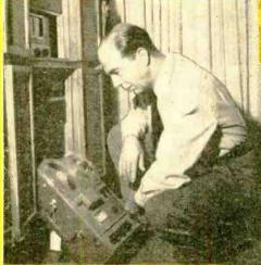
Bottom half of cabinet houses Ampex 600 tape recorder so mounted as to be readily removed when necessary. A McIntash 30-watt power amplifies sifs behind the Ampex tape recorder.
