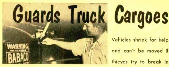
To enter cab after alarm has been set, the driver must shut off the alarm system. A special key is used; otherwise opening of door would release push button set in jamb and turn on siren. Even if a thief managed to enter the cab, a "parker" device would disable engine, and truck would not move.
