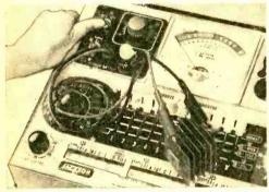
Ohio. All of the accessories use the basic meter and power supply to perform additional tube and component tests. To date, they include a high-resistance shorts tester, a selenium rectifier checker (shown in photo), and a heater current tester.
