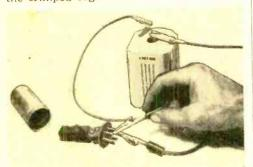
vibrator. Then the assembly may be removed from the can. As burnt contact points are a common cause of vibrator replacement, it will be necessary to polish the contact faces with fine sandpaper, and perhaps adjust the contact spacing.
