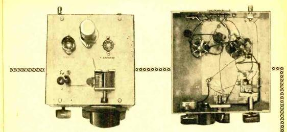
Top, bottom and rear views of the broadcast receiver. The wide-open construction shown here is not specifically required.
