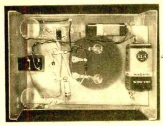
cell must be oriented so that light can reach the tiny window at the end of the unit over as wide an angle as possible.
