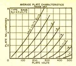
Fig. 3. Average plate characteristics of triode section of a 6AQ6 for use in quiz.
