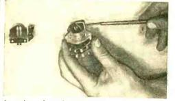
hex-shaped and will serve as a suitable wrench in an emergency. Cut the file tang at a point which will fit the particular socket setscrew. The file tang is soft and may be cut with a hack saw.
