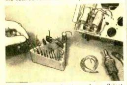
tion for rapid identification and use. Select the components needed for the job at hand and insert the wire leads in the corrugations.
