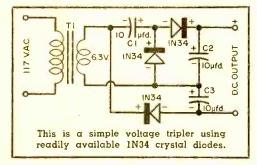
diodes. In each case, T1 is a 1-ampere, 6.3volt filament transformer. The circuits have been tested at a constant a.c. input voltage of 115 volts and their d.c. output characteristics are given in the graph. Except in the case of the doubler, the curves have not been carried beyond the current level at which the d.c. output voltage falls to 6.3, the r.m.s. voltage of the transformer secondary.
