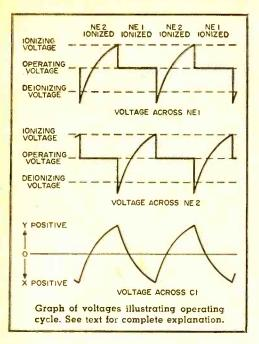
flashing alternately. The flashing rate is so high that each appears to be on continuously. Pressing the switch button stops the alternation, leaving on the lamp which happens to be glowing at the time.
