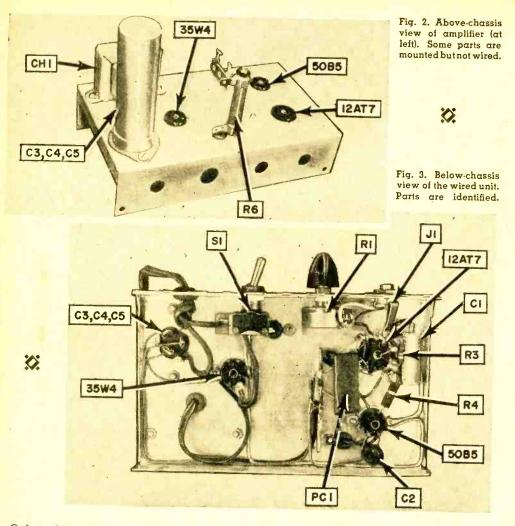
Only a few general precautions need be observed when wiring the amplifier. Carefully follow both the schematic and pictorial wiring diagrams, checking one diagram against the other as the wiring proceeds. Keep all signal leads as short and direct as possible. Insulate bare leads with spaghetti tubing. Don't bend the leads of the printed circuit plate too sharply as they may break off close to the plate.
