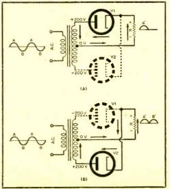
a generator were connected in place of *R*. This is called "half-wave rectification."
