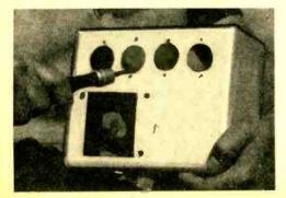
This type of deburring tool will clean out drilled holes in a chassis neatly, without flaring the surplus metal around the edge of a hole.
