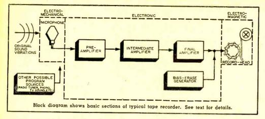
tude) of the sound. The recording head's core is made of iron so that it is magnetically "soft." Thus, it becomes a magnet only when, and to the extent that, current flows in the coil.
