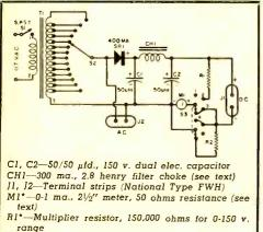
R2\*—Meter shunt, 0.33 ohms for 0-150 ma. range S1—S.p.s.t. toggle switch
