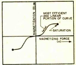
Above, magnetizing force (H) is current present in recording head. Resultant magnetization (B) does not follow straight linear pattern. Note "knees" in B-H curve at the points near zero magnetizing force and also as saturation is approached. Below, a.c. bias "straightens" curve to improve fidelity. Bias occupies inner white area, while signal modulation occupies shaded area. Thus, the signal to be recarded operates on the two most linear portions of the curve.
