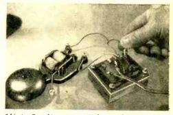
$1\frac{1}{2}$  to 6 volts may still be usable. Let the old transformer supply the low voltages needed for door bells, buzzers, toy electric motors, and similar jobs.
