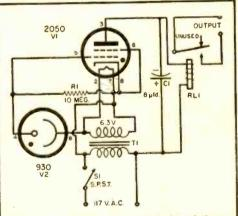
C1-8 µld., 450 v. midget tubular electrolytic capacitor
