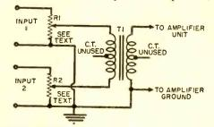
phono pickup, the potentiometer should be about 500,000 ohms.
