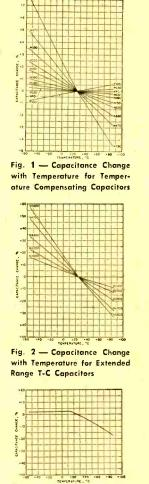
Fig. 3 — Capacitance Change with Temperature for Typical Class GA ±20% Tol. Units
