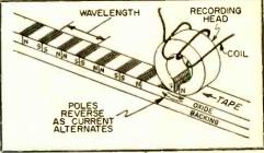
As tape passes under recording head, row of tiny bar magnets is impressed on it. Coil connects to output of tape amplifier.
