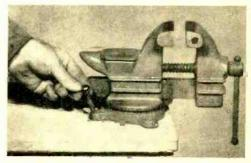
through the vise frame. By lifting the top slightly, nuts may be placed on the underside of the top for tightening the vise in place. This arrangement is particularly valuable in crowded quarters. -30-
