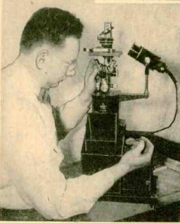
Highly accurate shadowgraph and microscopic studies are made of the finished diamond styli tips.
