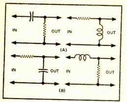
Fig. 4. Four basic arrangements involving resistance and either inductance or capacitance. The two arrangements at (Å) produce low-frequency loss and time advance of a continuous wave; the arrangements at (B) produce high-frequency loss and time delay.
