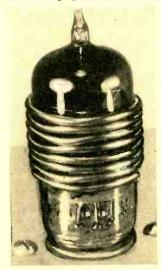
like a microphone (hence the name "microphonic"). A microphonic tube may be identified by tapping the various tubes in the equipment with the rubber tip of a pencil—if the complaint is caused as a particular tube is tapped, the defect has been located.
