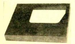
For home use, a simple base may serve to mount the turntable as well as the tone arm. Note the cutout for the motor. Tone arm is mounted at specified distance from turntable center by means of simple drilled holes. Manufacturer's templates provide complete guidance.
