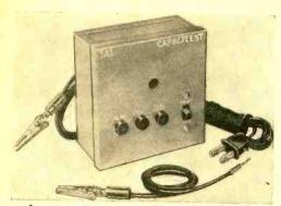
and a.c. and d.c. voltages. It differs from most meters in that it can check capacitors at 150 volts, which is approximately the working voltage in a radio or TV set. Most meters will not provide this type of check because the applied voltage is 20 volts or less.
