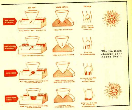
frequencies as stylus wear becomes progressively worse. Since musical sounds consist of a mixture of a dominant frequency combined with higher frequencies (overtones), stylus wear will almost always cause distortion.
