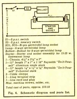
Regular power switch S1 permits the lamp to be turned off whenever the hamper is not in use.
